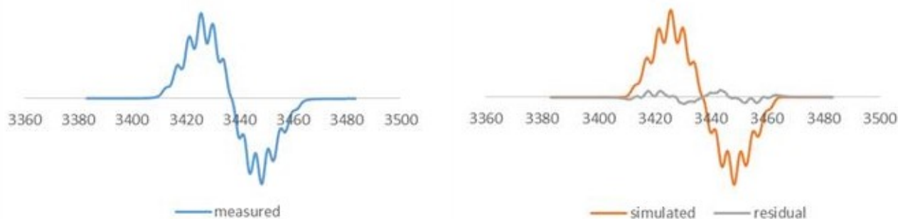
Figure S6. Experimental (blue, left), simulated (orange, right) and difference (grey, right) spectra for 1b recorded in benzene at ca 20 °C.
