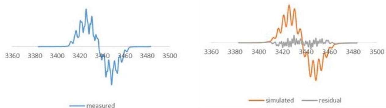
Figure S7. Experimental (blue, left), simulated (orange, right) and difference (grey, right) spectra for 1c recorded in benzene at ca 20 °C.
