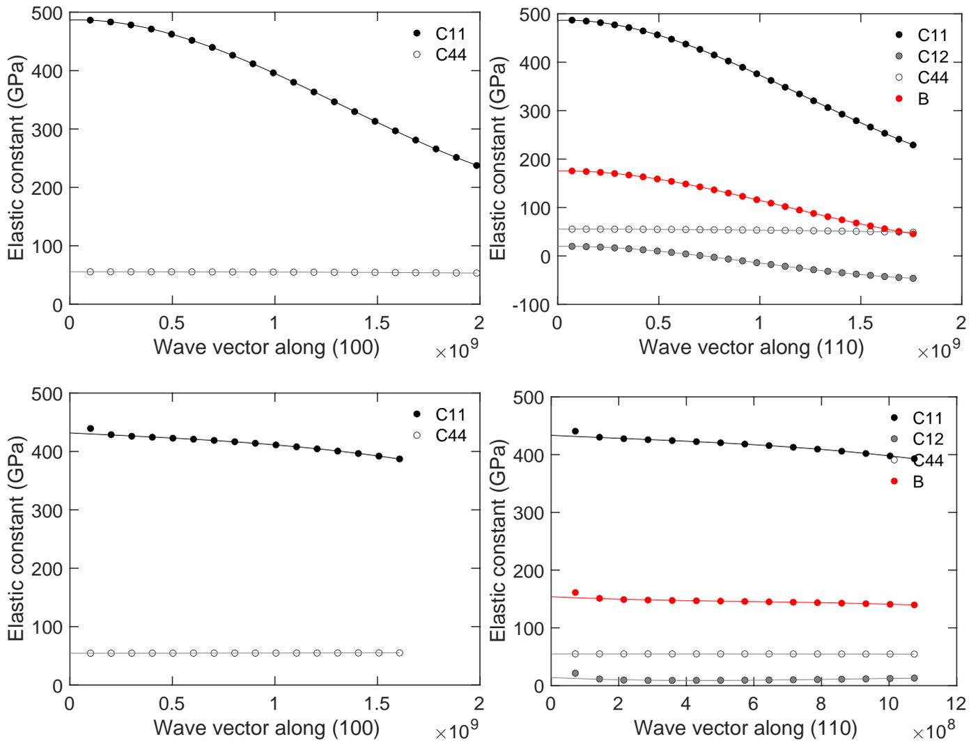
Fig. S3 Elastic constants of SmB<sub>6</sub> (top) and CaB<sub>6</sub> (bottom) evaluated for a range of wave vectors following equations ?? –??.
