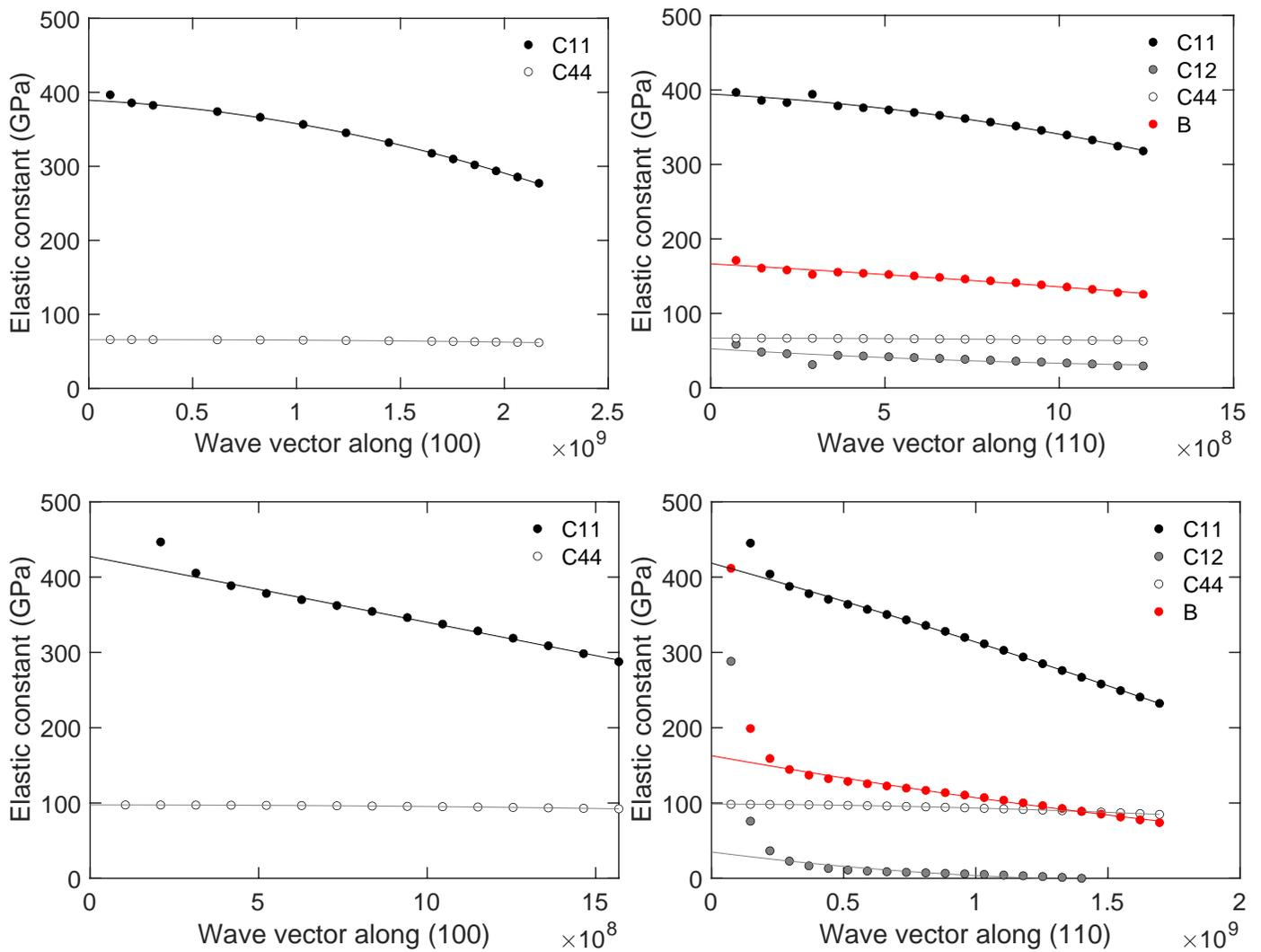
Fig. S4 Elastic constants of SrB<sub>6</sub> (top) and BaB<sub>6</sub> (bottom) evaluated for a range of wave vectors following equations ??-??.
