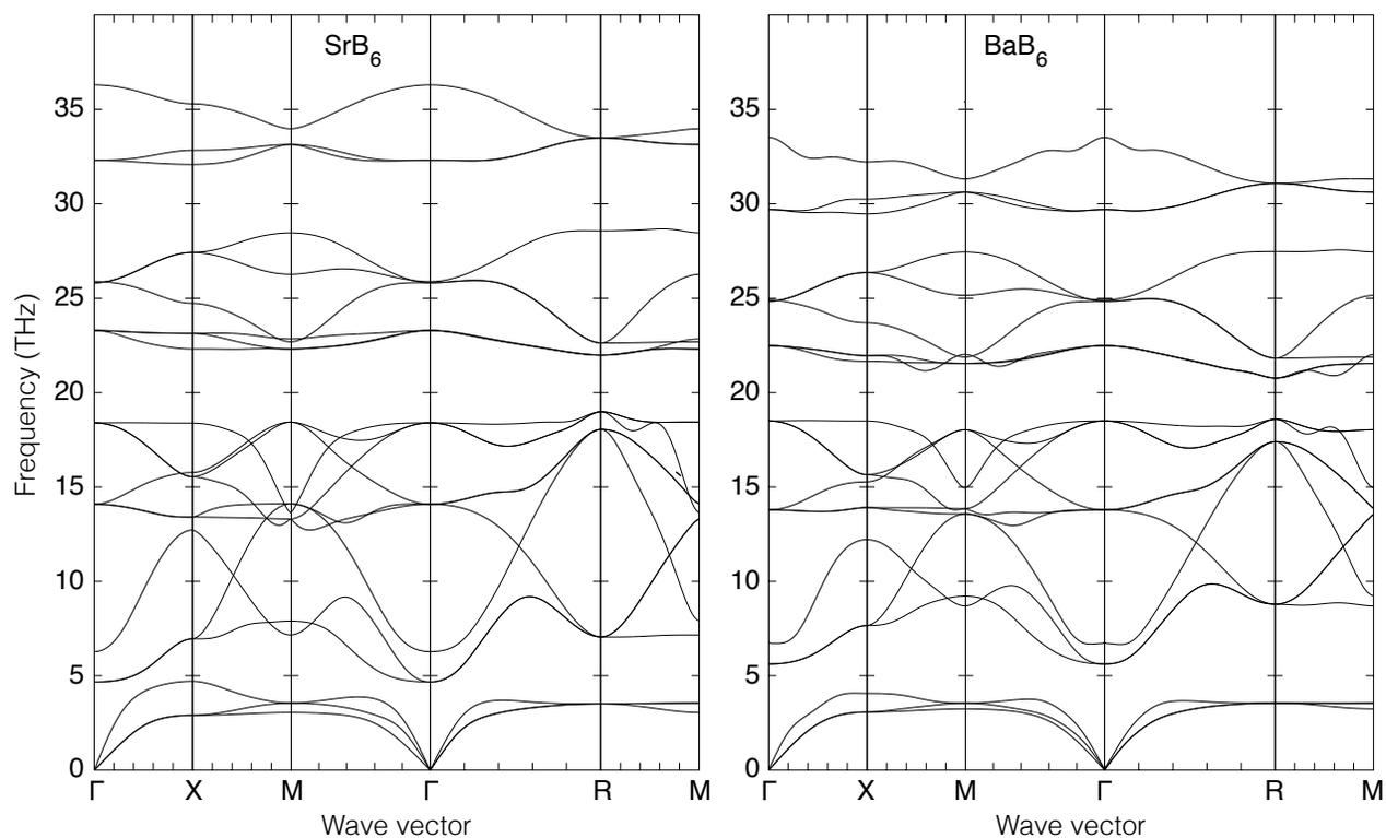
Fig. S1 Calculated phonon dispersion curves of  $\text{SrB}_6$  (left) and  $\text{BaB}_6$  (right). The wave vector labels have conventional meaning:  $\Gamma$  represents the wave vector  $[0,0,0]$ , X represents  $(\frac{1}{2},0,0)$ , M represents  $(\frac{1}{2},\frac{1}{2},0)$  and R represents  $(\frac{1}{2},\frac{1}{2},\frac{1}{2})$ .
