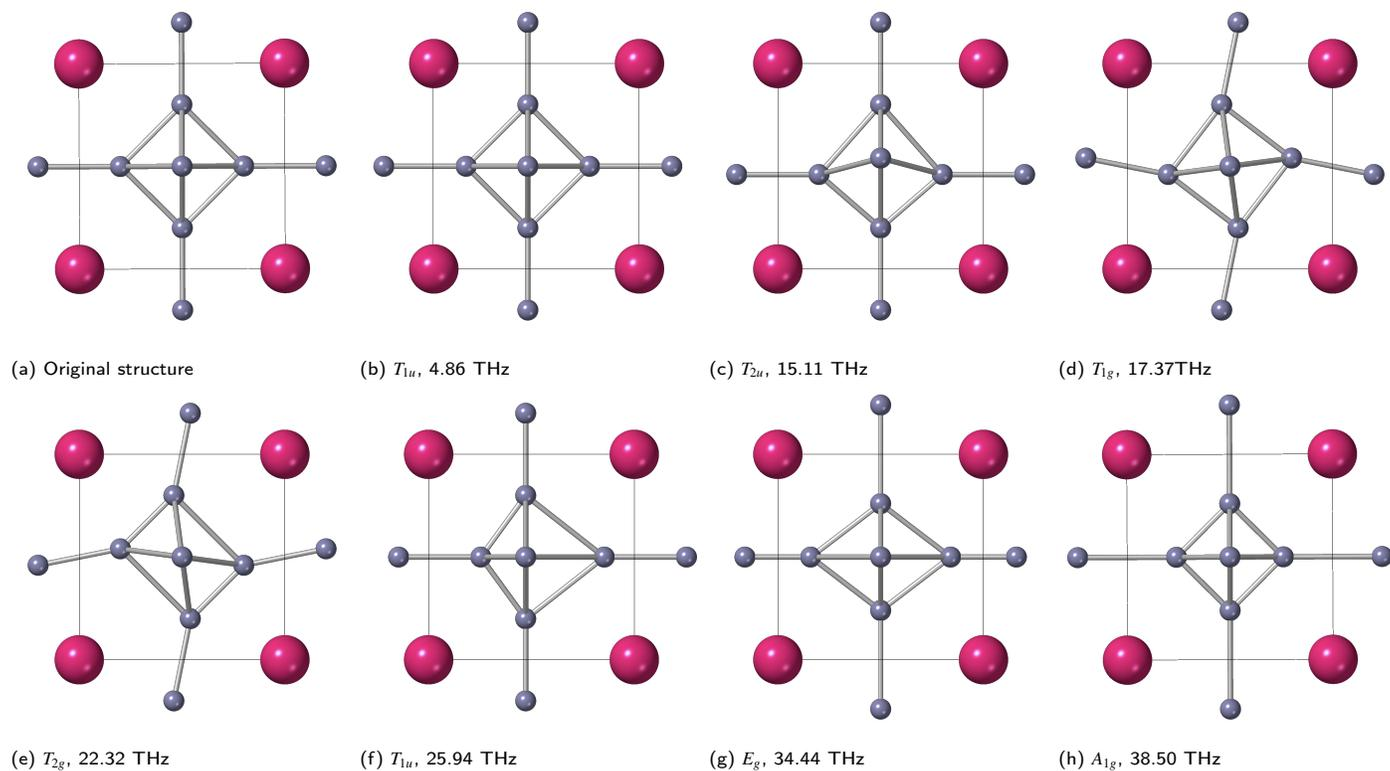
Fig. S2 Representation of the mode eigenvectors of the seven normal modes of  $\text{SmB}_6$  at zero wave vector. a) gives the original structure, and the other plots show the distortion of the crystal structure caused by each mode with corresponding irreducible representation and frequency.
