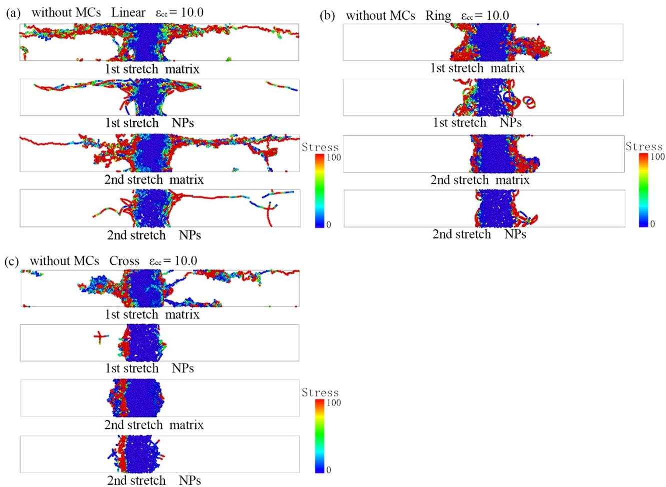
**Figure S12.** In the configurations without MCs. The heatmaps of matrix and NPs of (a) Linear, (b) Ring and (c) Cross structure PNCs at  $\epsilon_{cc} = 10.0$  during approximate triaxial tension and recovery process when stretched to maximum strain.
