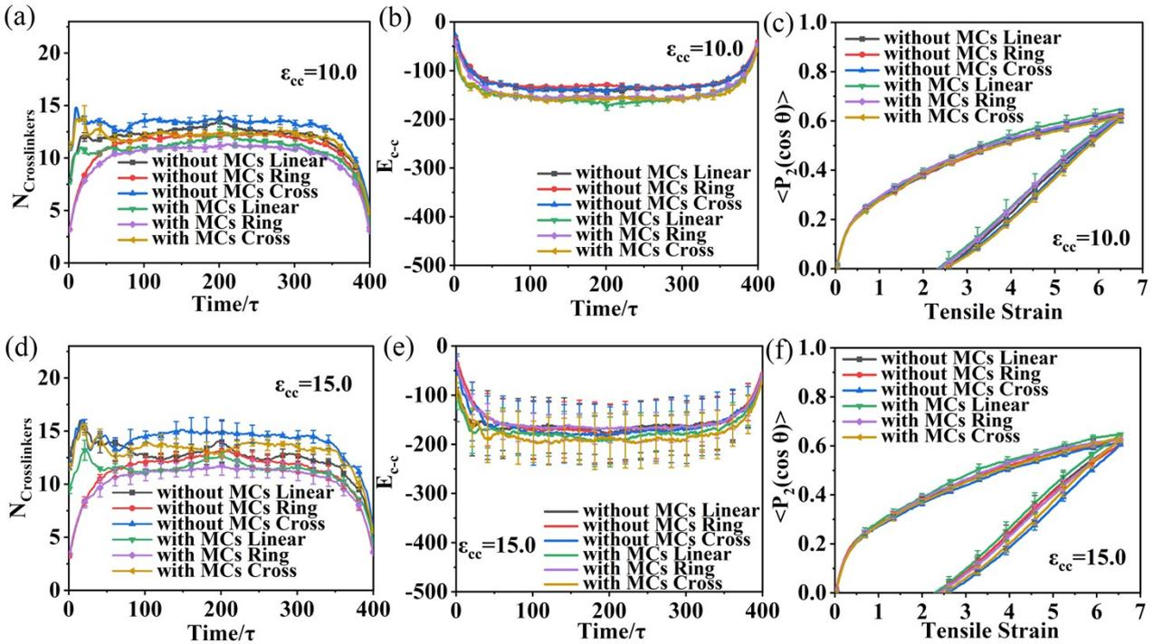
**Figure S5.** During the uniaxial tension and recovery process. (a) The average number of neighbor Crosslinkers, (b) the total interaction energy between Crosslinkers and (c) the matrix chains orientation at  $\epsilon_{cc} = 10.0$ . (d) The average number of neighbor Crosslinkers, (e) the total interaction energy between Crosslinkers and (f) the matrix chains orientation at  $\epsilon_{cc} = 15.0$ .
