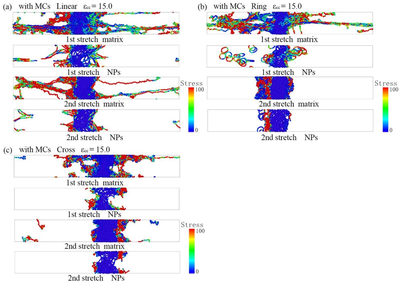
**Figure S20.** In the configurations with MCs. The heatmaps of matrix and NPs of (a) Linear, (b) Ring and (c) Cross structure PNCs at  $\epsilon_{cc} = 15.0$  during approximate triaxial tension and recovery process when stretched to maximum strain.
