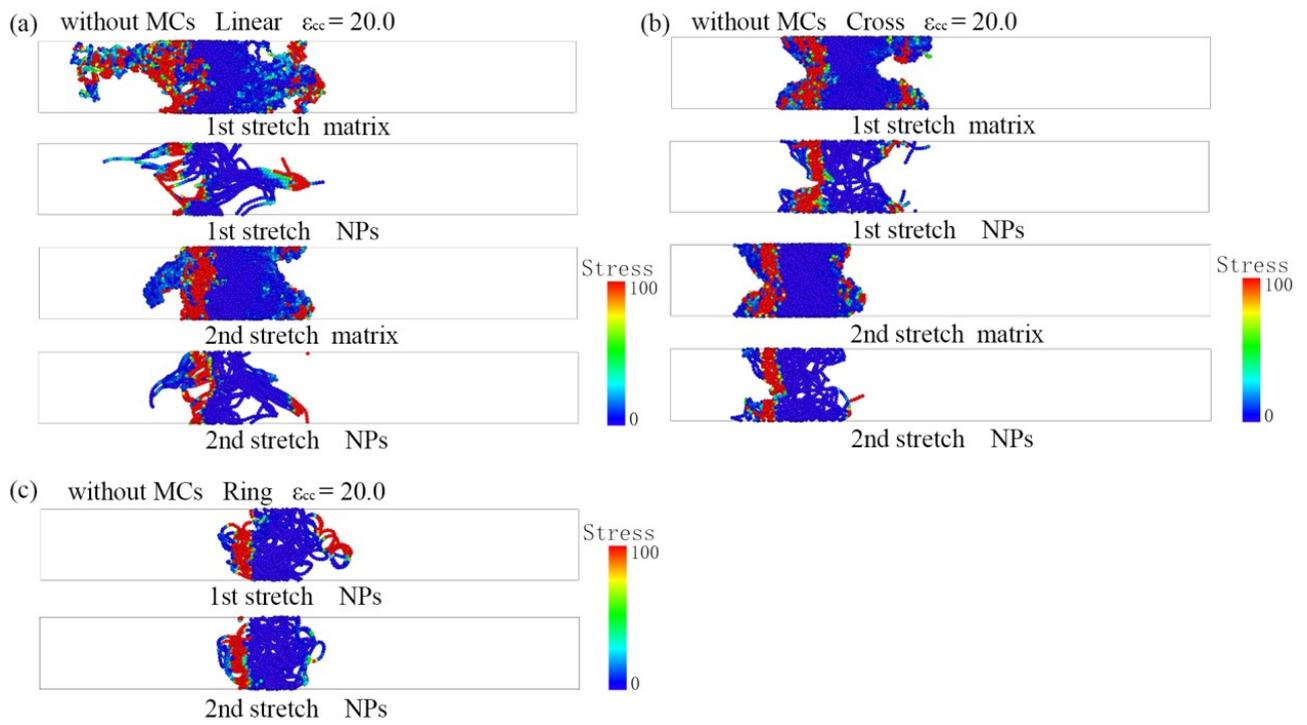
**Figure S14.** In the configurations without MCs. The heatmaps of matrix and NPs of (a) Linear and (b) Cross structure PNCs at  $\epsilon_{cc} = 20.0$ , and (c) the heatmaps of NPs of Ring structure PNCs at  $\epsilon_{cc} = 20.0$  during approximate triaxial tension and recovery process when stretched to maximum strain.
