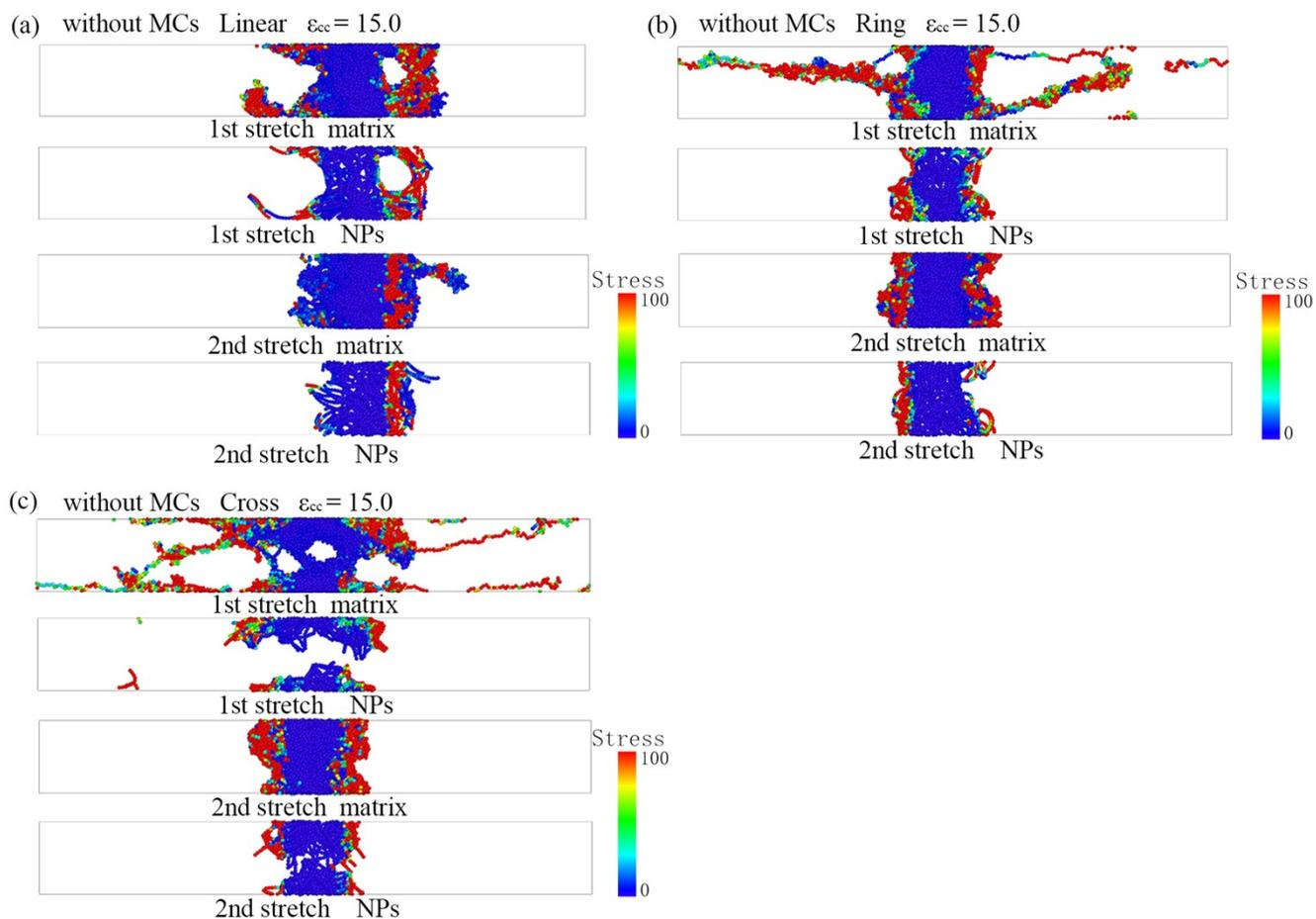
**Figure S13.** In the configurations without MCs. The heatmaps of matrix and NPs of (a) Linear, (b) Ring and (c) Cross structure PNCs at  $\epsilon_{cc} = 15.0$  during approximate triaxial tension and recovery process when stretched to maximum strain.
