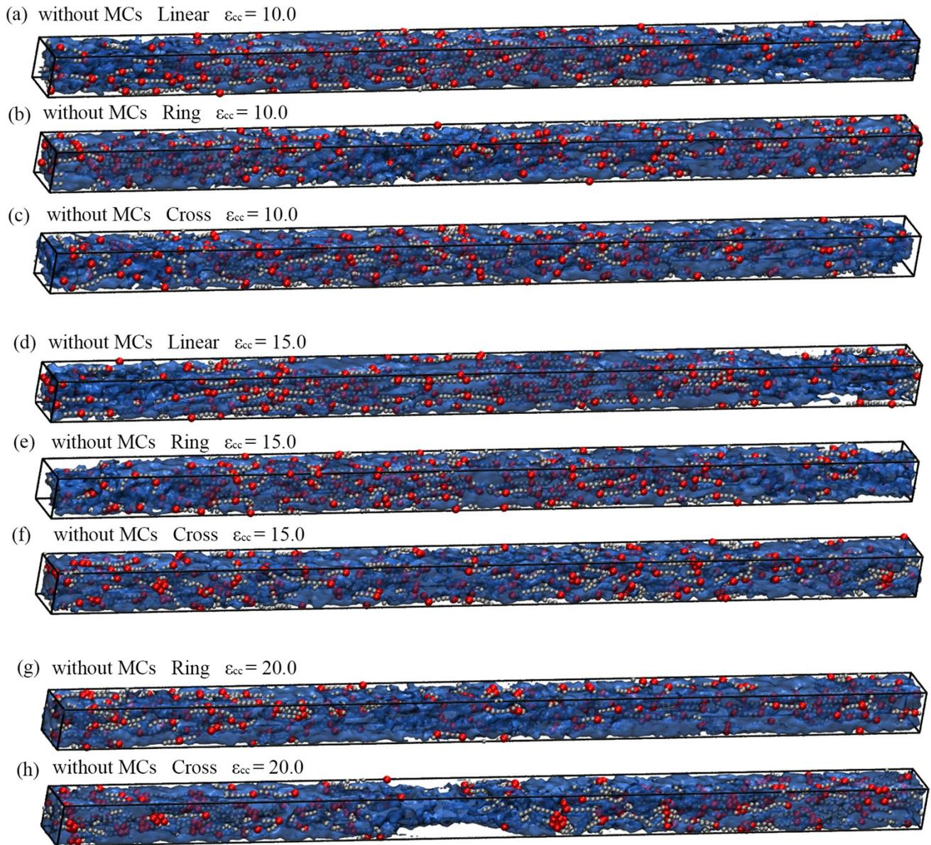
**Figure S6.** The snapshots at maximum uniaxial strain of (a) Linear, (b) Ring and (c) Cross structure PNCs without MCs at  $\epsilon_{cc} = 10.0$ . (d) Linear, (e) Ring and (f) Cross structure PNCs without MCs at  $\epsilon_{cc} = 15.0$ . (g) Ring and (h) Cross structure PNCs without MCs at  $\epsilon_{cc} = 20.0$ .
