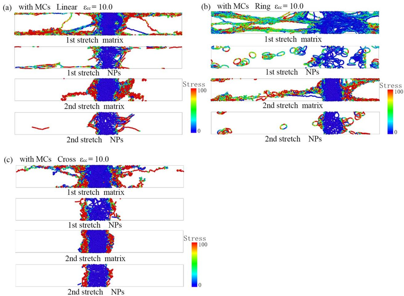
**Figure S19.** In the configurations with MCs. The heatmaps of matrix and NPs of (a) Linear, (b) Ring and (c) Cross structure PNCs at  $\epsilon_{cc} = 10.0$  during approximate triaxial tension and recovery process when stretched to maximum strain.
