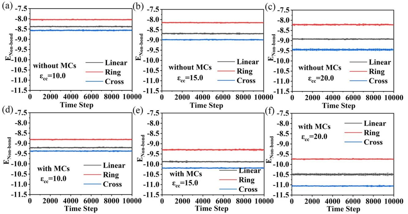
**Figure S22.** The last 10,000 steps of the equilibrium process of non-bond interaction energy curve: configurations without MCs at (a)  $\epsilon_{cc} = 10.0$ , (b)  $\epsilon_{cc} = 15.0$ , (c)  $\epsilon_{cc} = 20.0$ , and configurations with MCs at: (d)  $\epsilon_{cc} = 10.0$ , (e)  $\epsilon_{cc} = 15.0$ , (f)  $\epsilon_{cc} = 20.0$ .
