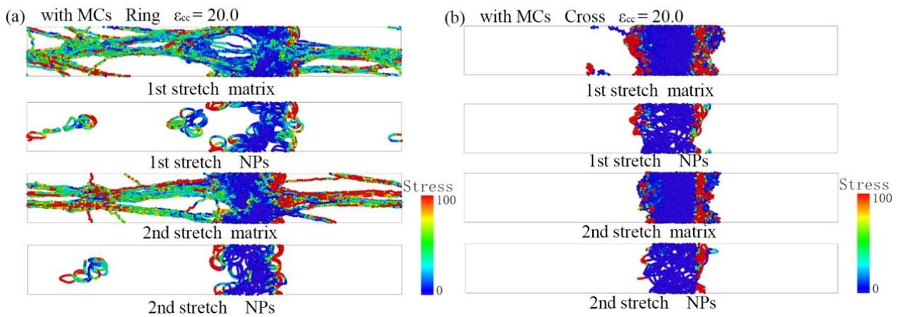
**Figure S21.** In the configurations with MCs. The heatmaps of matrix and NPs of (a) Ring and (b) Cross structure PNCs at  $\epsilon_{cc} = 20.0$  during approximate triaxial tension and recovery process when stretched to maximum strain.
