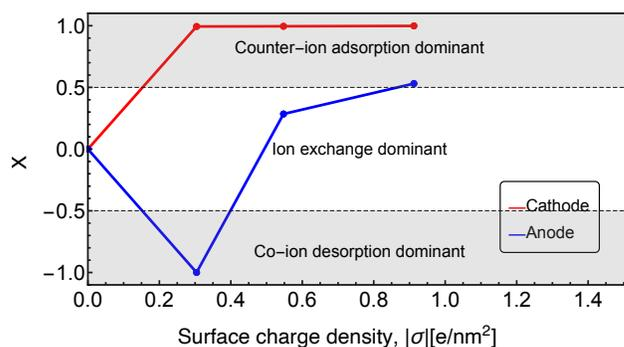
**Fig. S8** X-parameter calculated within the first layer of solution at the interface, during charging at the cathode (red) and at the anode (blue) system with polarisable water and polarisable gold.
