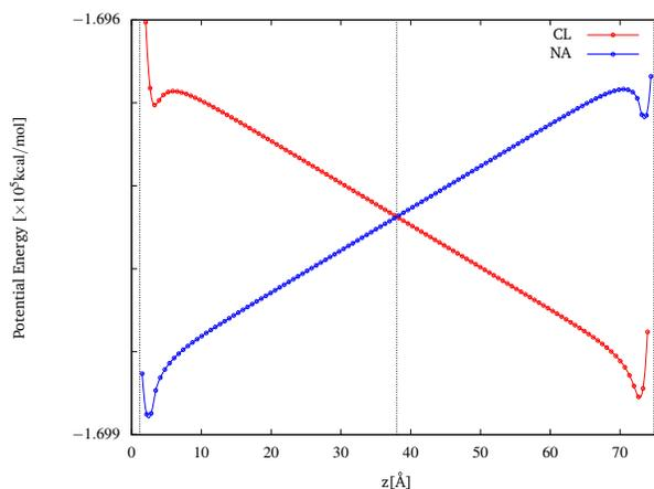
**Fig. S2** Potential energy of Na (blue) or Cl (red) with  $-0.061 e \text{ nm}^{-2}$  on left electrode and  $0.061 e \text{ nm}^{-2}$  on right electrode.
