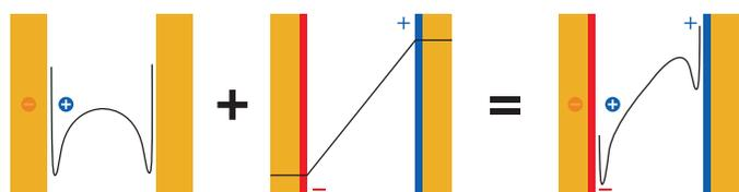
**Fig. S1** Schematic depiction expected potential energy within the parallel plate capacitor. The blue dots represent a unit test positive charge and its image charge in the metal.
