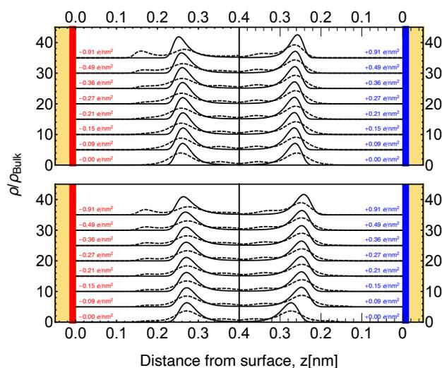
**Fig. S5** Number densities  $\rho$  of O (solid), H (dashed) normalised with their bulk densities  $\rho_{Bulk}$ , at the cathode (left) and at the anode (right) at varying surface charge. The top and bottom panels correspond to non-polarisable and polarisable gold respectively. The number densities are shifted up in steps of 5 in ascending surface charge for clarity.
