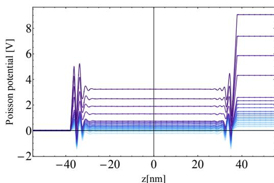
**Fig. S4** Poisson potential drops at different surface charges at a non-polarisable gold surface. Increasing magnitude of surface charge is shown by increasingly darker lines.
