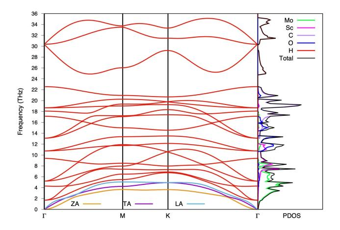
Figure. Phonon dispersion curve and phonon density of states obtained using the hipHive code.
