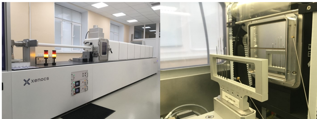
Supplementary Fig. S4. Photos of the Xeuss 3.0 SAXS/WAXS System (installed and operated in FLNP, JINR, Dubna) used for acquiring the main XRD data. On the left side is the general view of the system and on the right is the sample holder with capillaries containing hydrated eumelanins.
