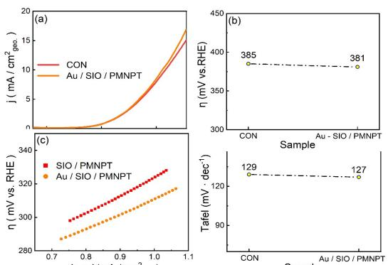
FigureS1 Electrocal Slytic Characterization of OER in SIO/PMNPT (CSR) and Au/SIO/PMNPT samples. (a) LSV curve when a scanning rate of 5 mV/s. (b) Overpotential at  $\eta_{j=10}$ . (c) Tafel diagram, (d) Tafel slope.
