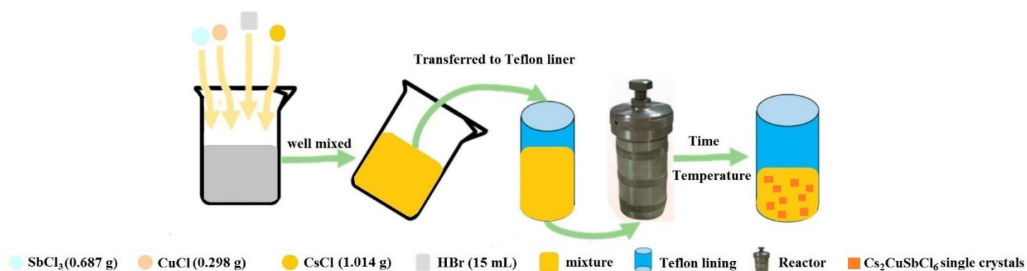
Fig. S1. Schematic picture of the solvothermal method to obtain \text{Cs}_2\text{CuSbCl}_6 single crystals.
