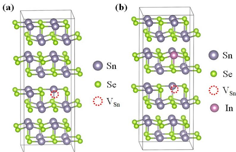
SFig1 crystal structure model of  $Sn_{31}Se_{32}$  (a) and  $Sn_{30}InSe_{32}$  (b)
