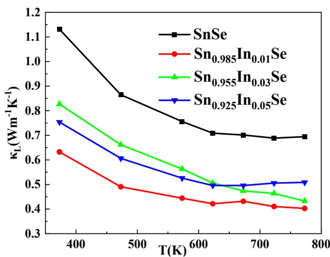
SFig2 Temperature dependency of lattice thermal conductivity for  $Sn_{1-3x/2}In_xSe$  ( $x = 0.0, 0.01, 0.03, 0.05$ ) samples.
