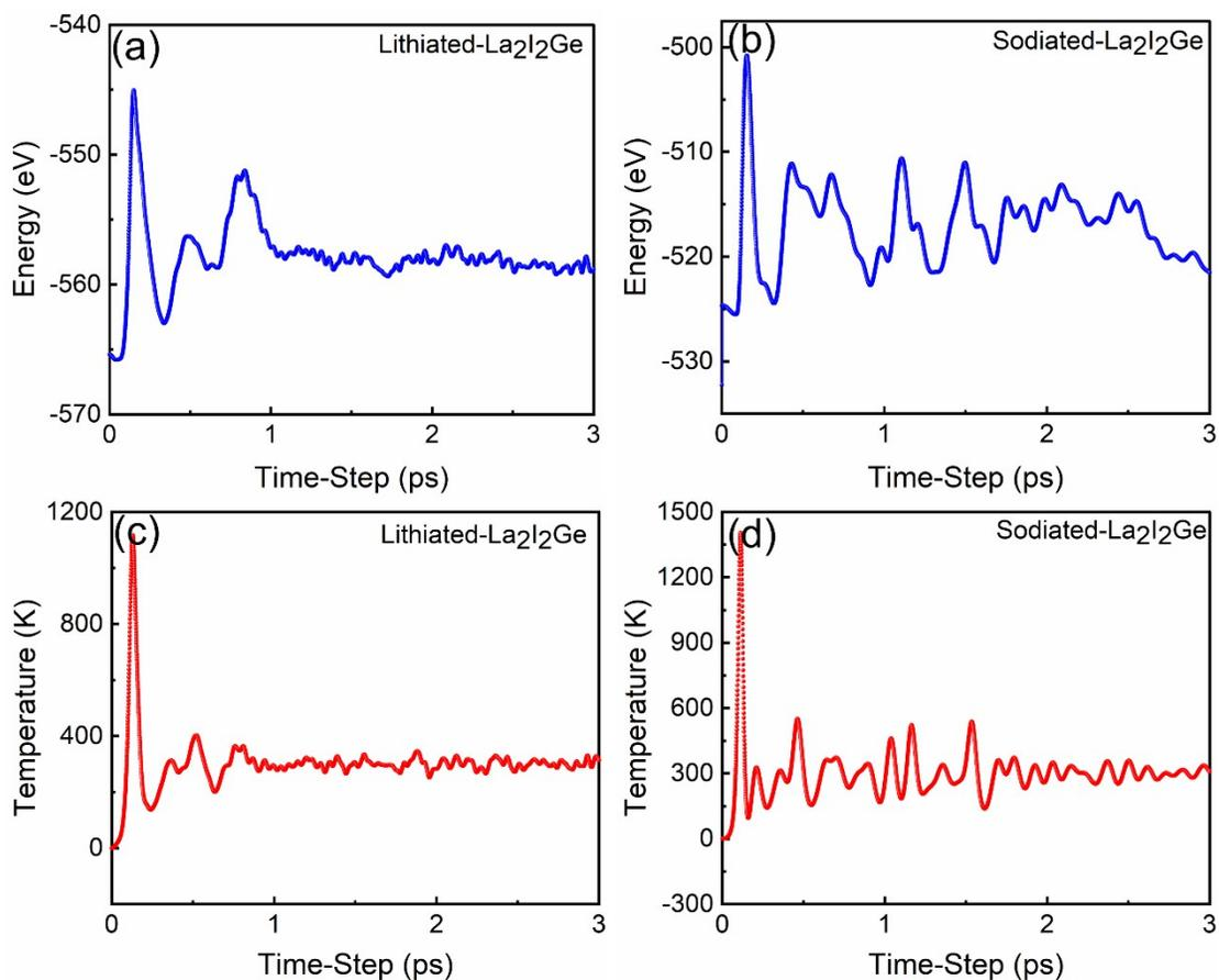
Fig. S5 Evolutions of the total energy and temperature of fully lithated and sodiated La<sub>2</sub>I<sub>2</sub>Ge nanosheets during the AIMD simulations at 300 up to 3 ps. These results indicate that La<sub>2</sub>I<sub>2</sub>Ge nanosheets are thermodynamically stable.
