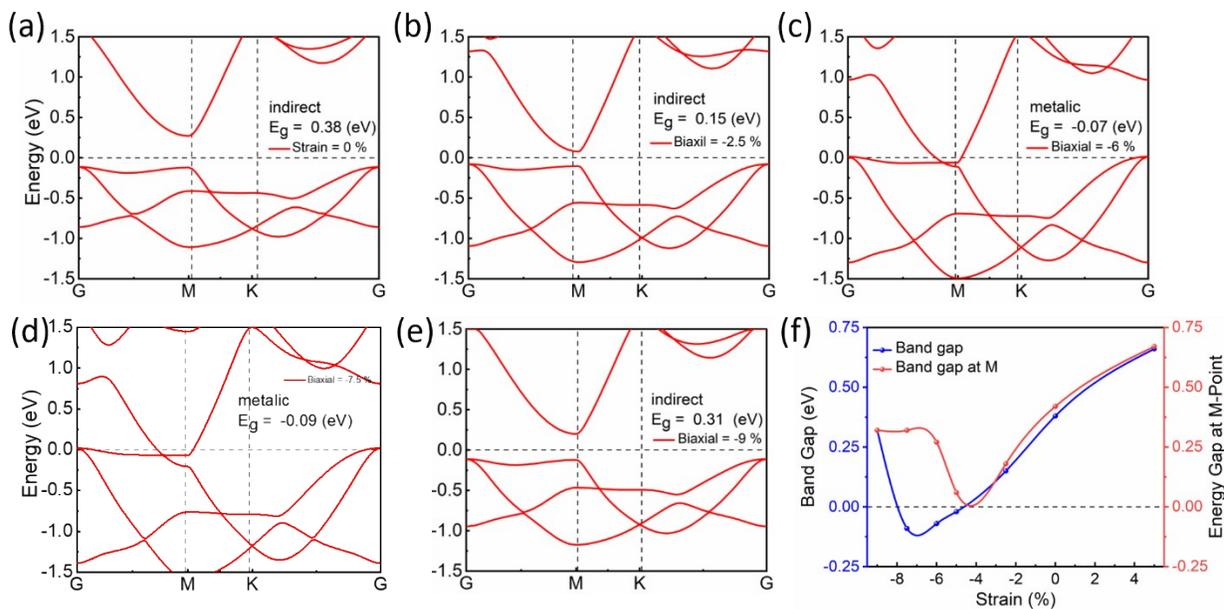
Fig. S2 Electron band structure of  $\text{La}_2\text{I}_2\text{Ge}$ , (a) no strain (b), 2.5% (c), 6% (d) 7% (e) 9% biaxial compressive strain. And (f) depicts that band gap nearly closes at 6% compressive strain, and reopens with further increase of the compressive strain.
