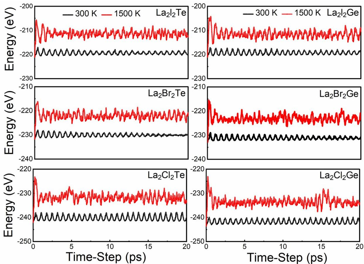
Fig. S3 Evolutions of the total energy of  $\text{La}_2\text{X}_2\text{Y}$  ( $\text{X} = \text{I}, \text{Br}, \text{Cl}$ ;  $\text{Y} = \text{Ge}, \text{Te}$ ) nanosheets during the AIMD simulations at 300, and 1500 K up to 20 ps. These results indicate that  $\text{La}_2\text{X}_2\text{Y}$  nanosheets are thermodynamically stable.
