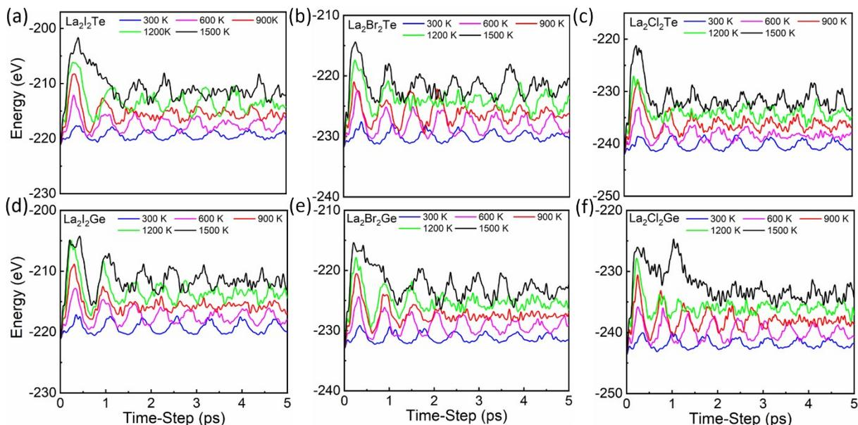
Fig. S1 Evolutions of the total energy of  $\text{La}_2\text{X}_2\text{Y}$  ( $\text{X} = \text{I}, \text{Br}, \text{Cl}; \text{Y} = \text{Ge}, \text{Te}$ ) nanosheets during the AIMD simulations from 300-1500 K up to 5 ps. These results indicate that  $\text{La}_2\text{X}_2\text{Y}$  nanosheets are thermodynamically stable.
