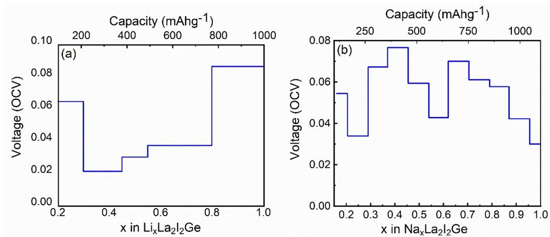
Fig. S7 Open-circuit voltage (OCV) as a function of the (a) Li concentration  $x$ , and (b) Na concentration  $x$
