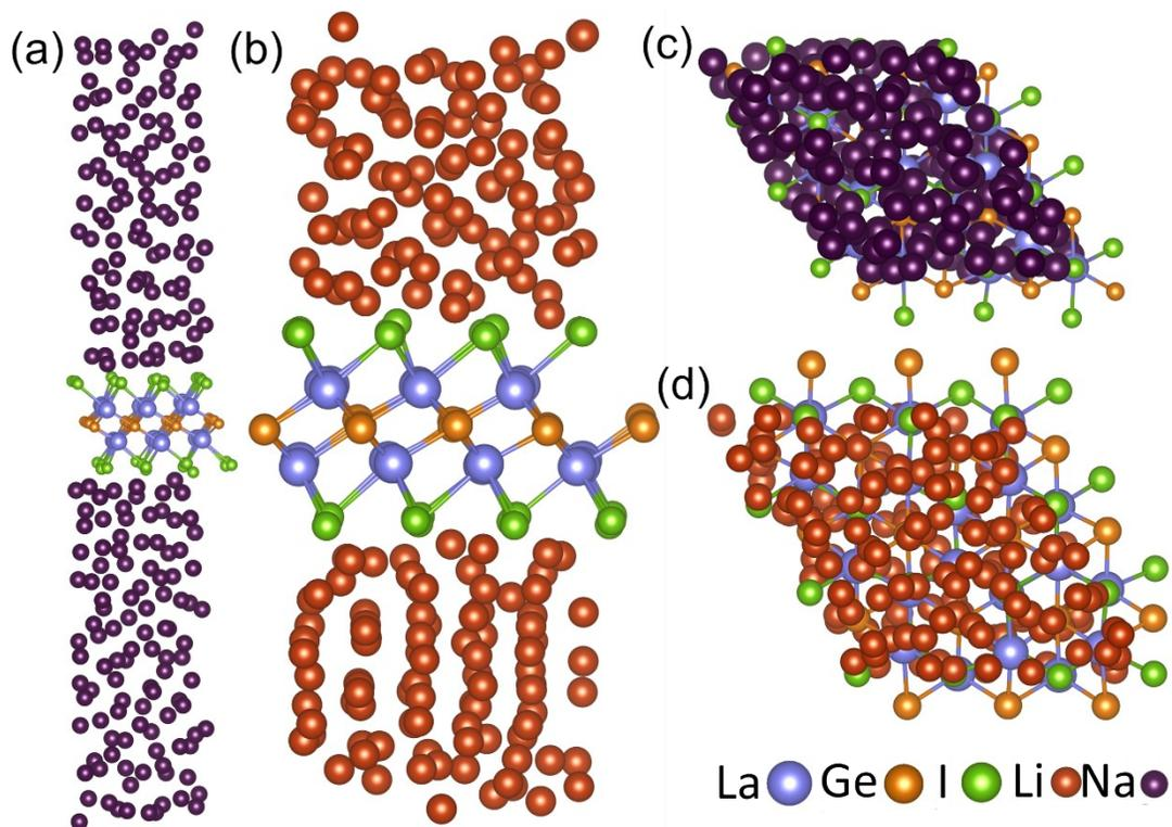
Fig. S6 Geometric configurations of  $\text{La}_2\text{I}_2\text{Ge}$  nanosheets during AIMD simulations at 300K over 3 ps. (a, b) Side views; (c, d) Top views. The structures suggest thermodynamic stability in fully lithiated/sodiated states.
