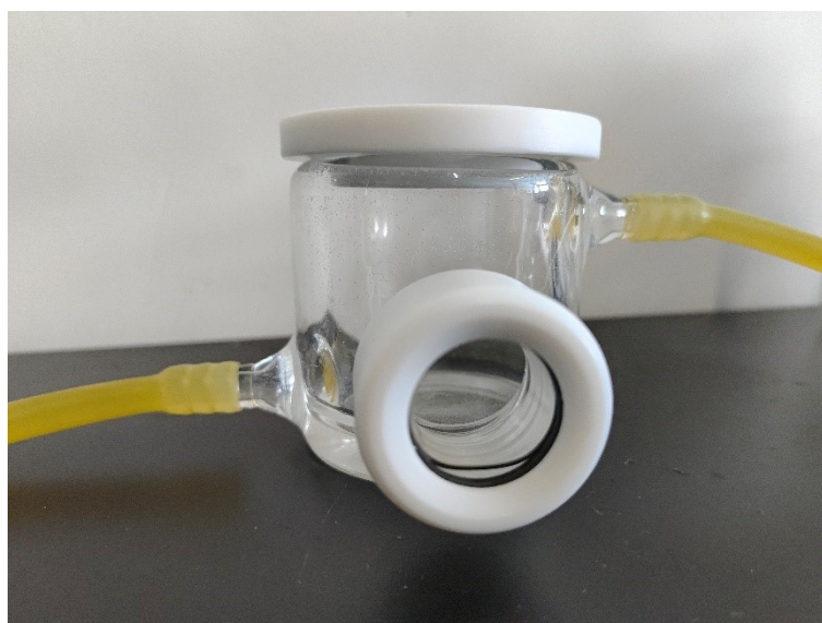
Figure S1 The photograph of double-layer electrochemical cell with recirculating water.
