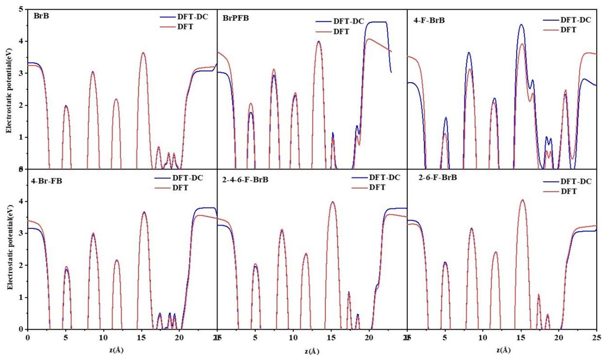
**Fig. S9.** The difference in the planar average potential calculated using dipole correction in the adsorption of small molecules with different F contents at the  $\text{PbI}_2$ -terminated surfaces. Blue refers to adding dipole correction during calculation, while red refers to using DFT instead of adding dipole correction during calculation.
