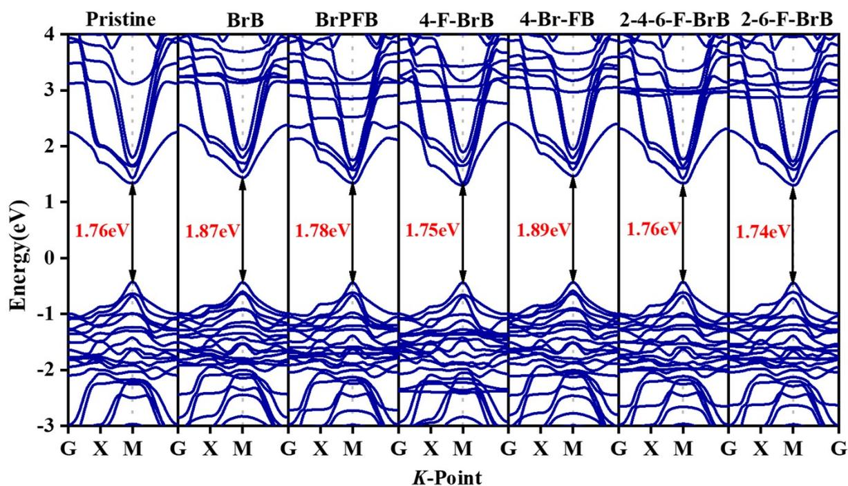
**Fig. S6.** Band structures is displayed at the PbI<sub>2</sub>-terminated surface with the addition of BrB, BrPFB, 4-F-BrB, 4-Br-FB, 2-4-6-F-BrB, and 2-6-F-BrB, respectively.
