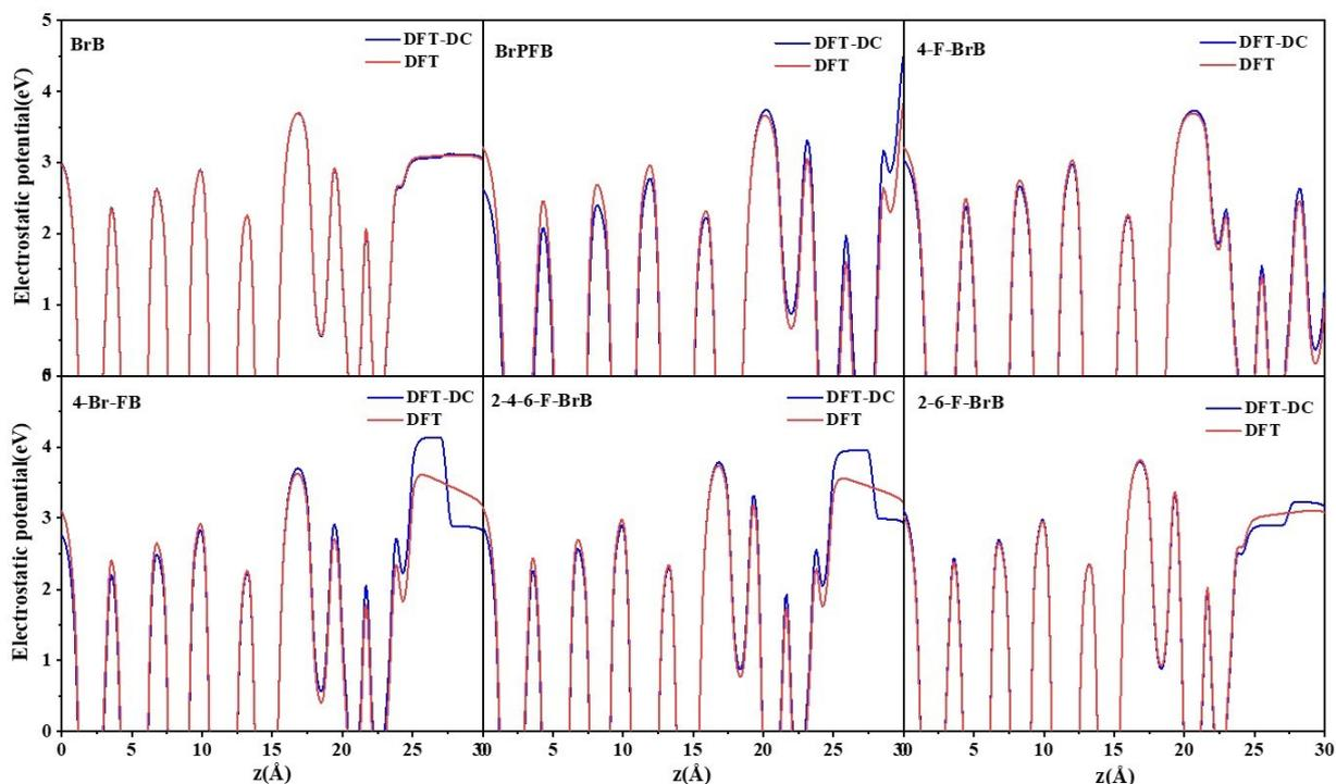
**Fig. S10.** The difference in the planar average potential calculated using dipole correction in the adsorption of small molecules with different F contents at the MAI-terminated surfaces. Blue refers to adding dipole correction during calculation, while red refers to using DFT instead of adding dipole correction during calculation.
