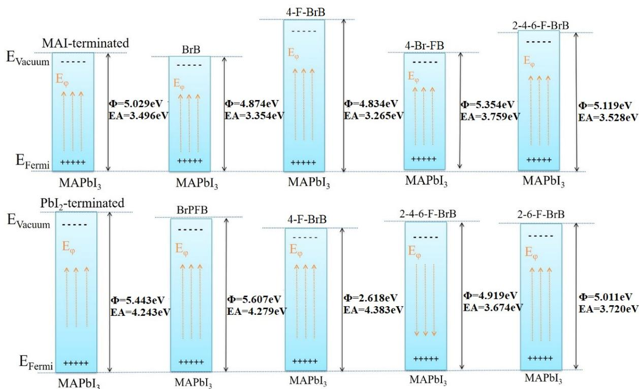
**Fig. S7.** The surface work function of the intrinsic structure and the electron affinity potential(EA) after adsorbing BrB, 4-F-BrB, 4-Br-FB and 2-4-6-F-BrB on the MAI-terminated surface and adsorbing BrPFB, 4-F-BrB, 2-4-6-F-BrB, and 2-6-F-BrB on the PbI<sub>2</sub>-terminated surface.
