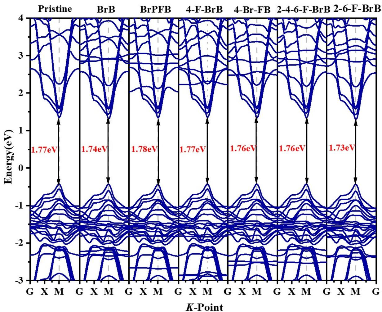
**Fig. S5.** Band structures is displayed at the MAI-terminated surface with the addition of BrB, BrPFB, 4-F-BrB, 4-Br-FB, 2-4-6-F-BrB, and 2-6-F-BrB, respectively.
