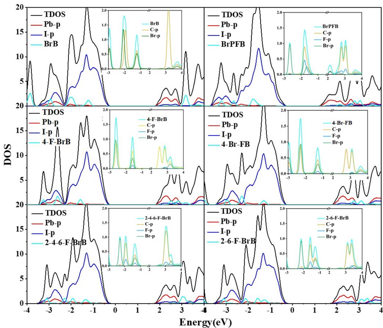
**Fig. S4.** The partial densities of states at the  $\text{PbI}_2$ -terminated surface with the addition of BrB, BrPFB, 4-F-BrB, 4-Br-FB, 2-4-6-F-BrB, and 2-6-F-BrB, respectively.
