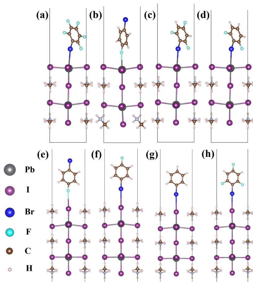
**Fig. S1.** Passivation models for different terminals of perovskite. (a)-(d) represents the addition of BrPFB, 4-F-BrB, 2-4-6-F-BrB and 2-6-F-BrB on the PbI<sub>2</sub>-terminated surface. (e)-(h) represents the addition of 4-F-BrF, 4-Br-BrF, BrB and 2-4-6-F-BrB on the MAI-terminated surface.
