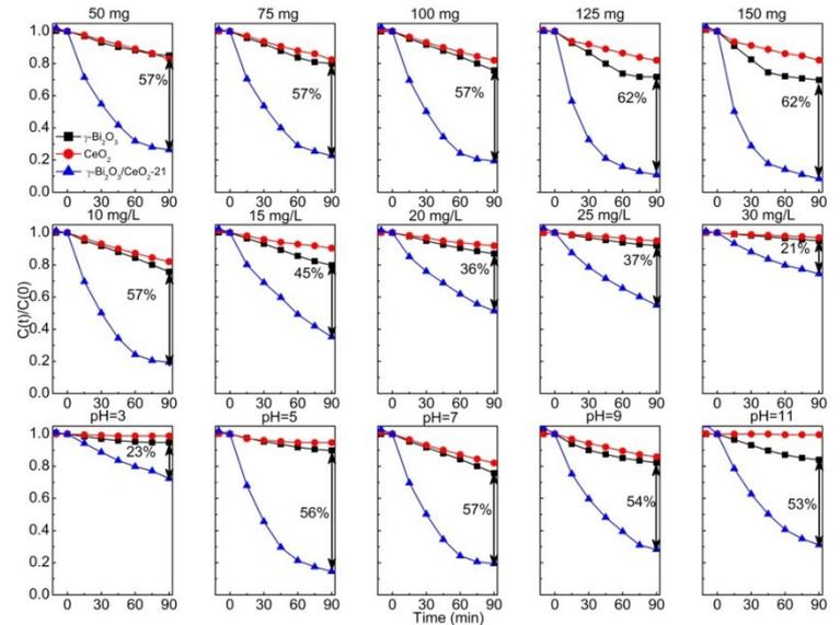
Figure S6 Tetracycline degradation efficiency for different initial conditions
