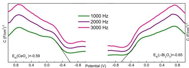
Figure S9 Mott-Schottky curves of  $\text{CeO}_2$  and  $\gamma\text{-Bi}_2\text{O}_3$
