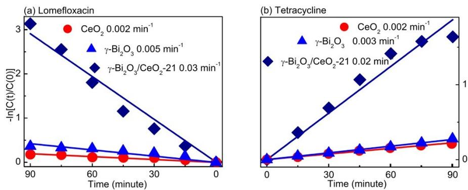
Figure S3 First-order degradation rate constants upon three typical samples
