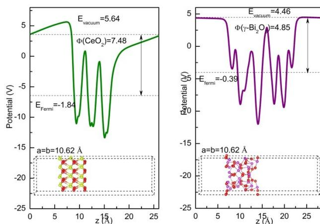
Figure S8 Optimized structures and electrostatic potential curves of  $\text{CeO}_2$  (100) and  $\gamma\text{-Bi}_2\text{O}_3$  (100) surfaces
