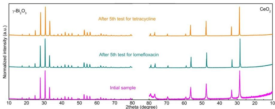
Figure S7 XRD profiles of the pure phase samples upon before and after the fifth cycling test
