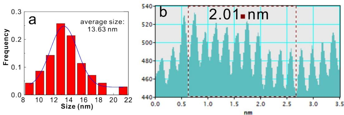
Fig. S1 (a) particle size distribution of the metal nanoparticles in Fe-CoNC, (b) measurement of lattice fringe in Fig. 1d
