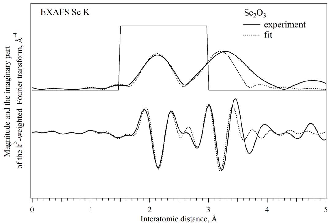
Fig. S4: Experimental (solid line) and fitted (dotted line) magnitude and the imaginary part of the FT of Sc<sub>2</sub>O<sub>3</sub>, the fitting range is marked by thin solid line.
