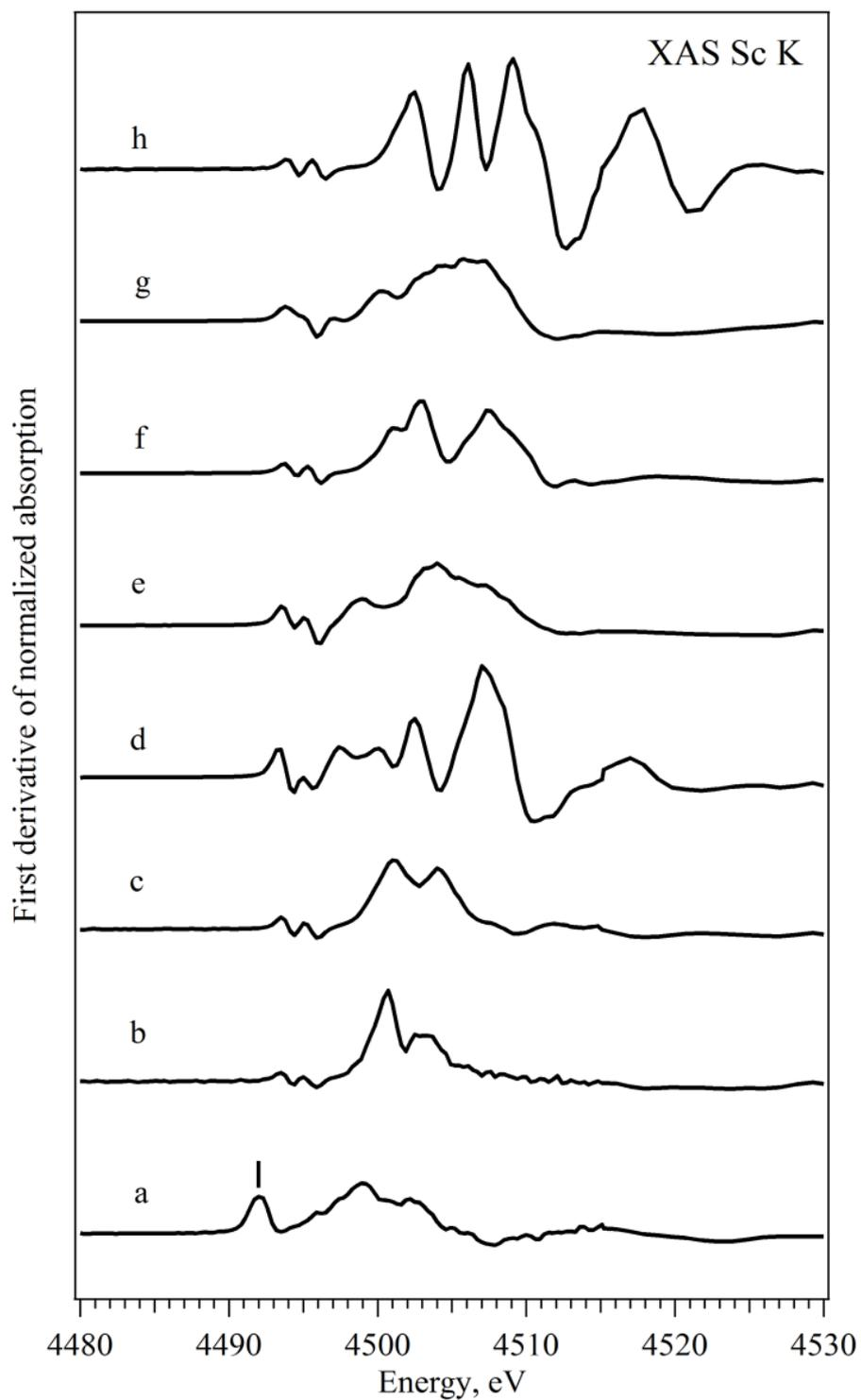
Fig. S2. First derivative of normalized XAS Sc K spectra of different Sc compounds: (a) Sc metal, (b)  $\text{ScBr}_3$ , (c)  $\text{ScCl}_3$ , (d)  $\text{Sc}_2\text{O}_3$ , (e)  $\text{Sc}_2(\text{CO}_3)_3$ , (f)  $\text{Sc}_2(\text{SO}_4)_3$ , (g)  $\text{Sc}(\text{NO}_3)_3$ , (h)  $\text{ScF}_3$ . The vertical line marks the position of the absorption edge of the Sc metal.
