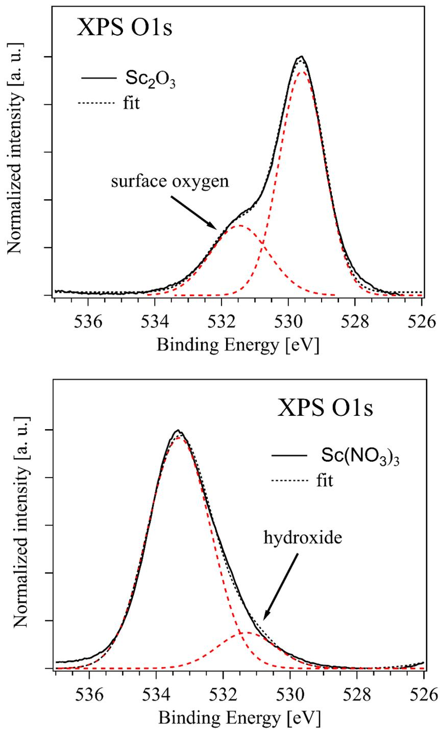
Fig. S3. Results of the peak decomposition analysis of the O 1s XPS data on  $\text{Sc}_2\text{O}_3$  and  $\text{Sc}(\text{NO}_3)_3$ .
