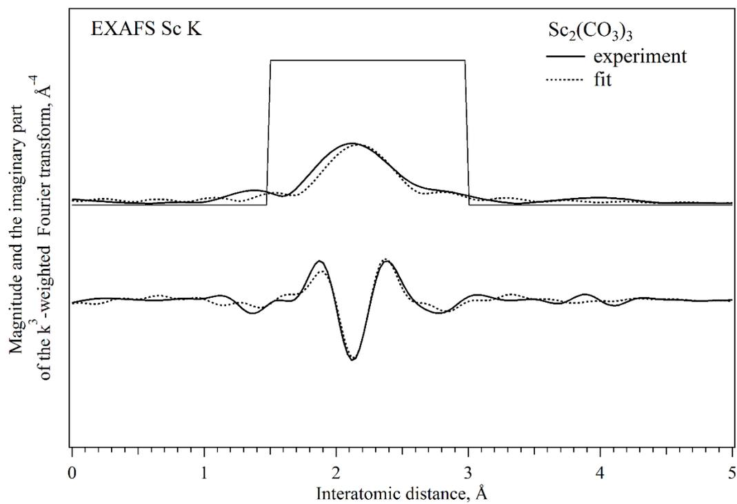
Fig. S7: Experimental (solid line) and fitted (dotted line) magnitude and the imaginary part of the FT of Sc<sub>2</sub>(CO<sub>3</sub>)<sub>3</sub>, the fitting range is marked by thin solid line.
