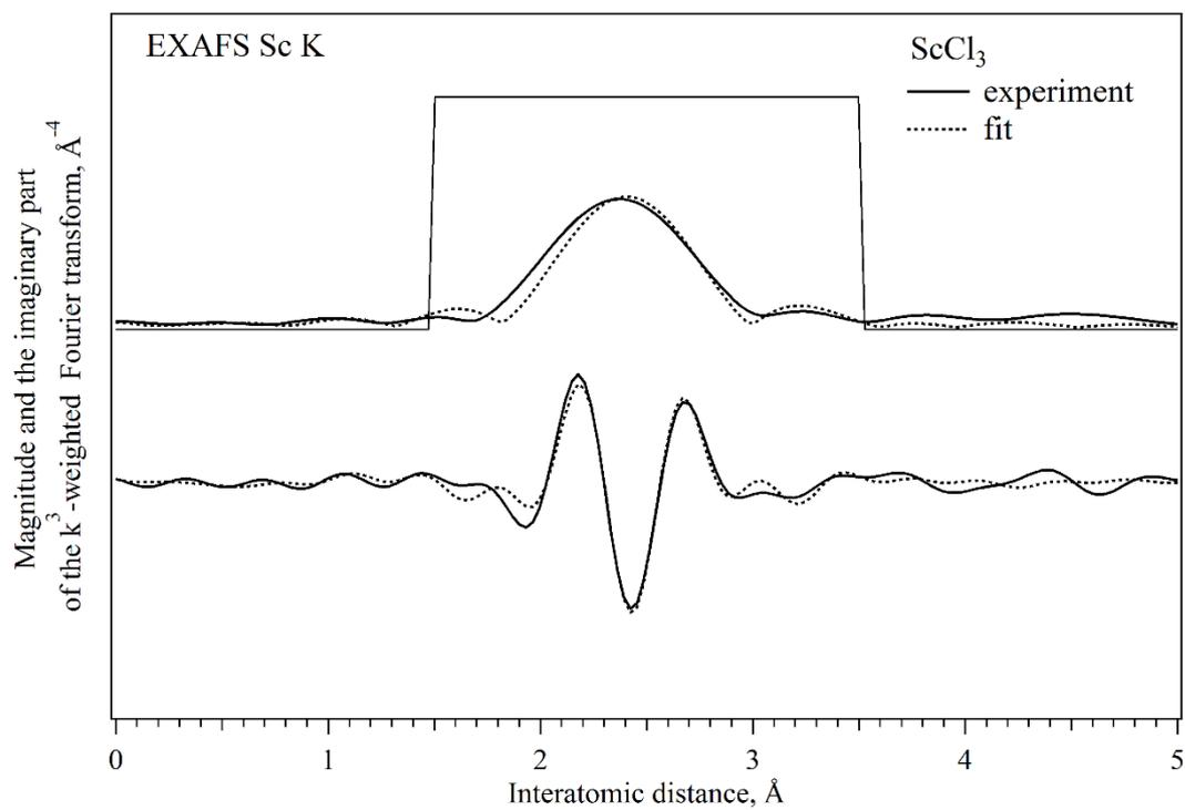
Fig. S5: Experimental (solid line) and fitted (dotted line) magnitude and the imaginary part of the FT of ScCl<sub>3</sub>, the fitting range is marked by thin solid line.
