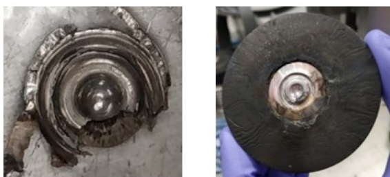
Figure S2 Ruptured Ti-Zr gasket and cracked anvil after violent decomposition at 4.46 GPa.
