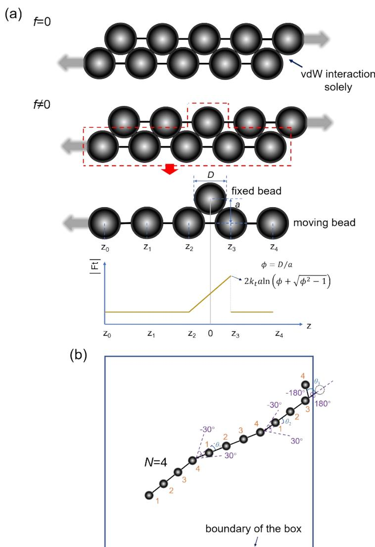
Figure S1 (a) The mechanical behavior of the interface friction  $f$ .<sup>1</sup> (b) Generation process of beads ( $N=4$ ).
