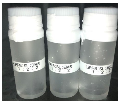
Figure S6. Photograph of the ternary mixtures of [\text{LiPF}_6]/[\text{SL}]/[\text{another sulfone}] = 1/2/2 after one month of storage in a -20\text{ }^\circ\text{C} freezer.
