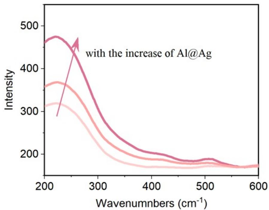
Figure S3. Roman spectrum of elastomers with different content of Al@Ag
