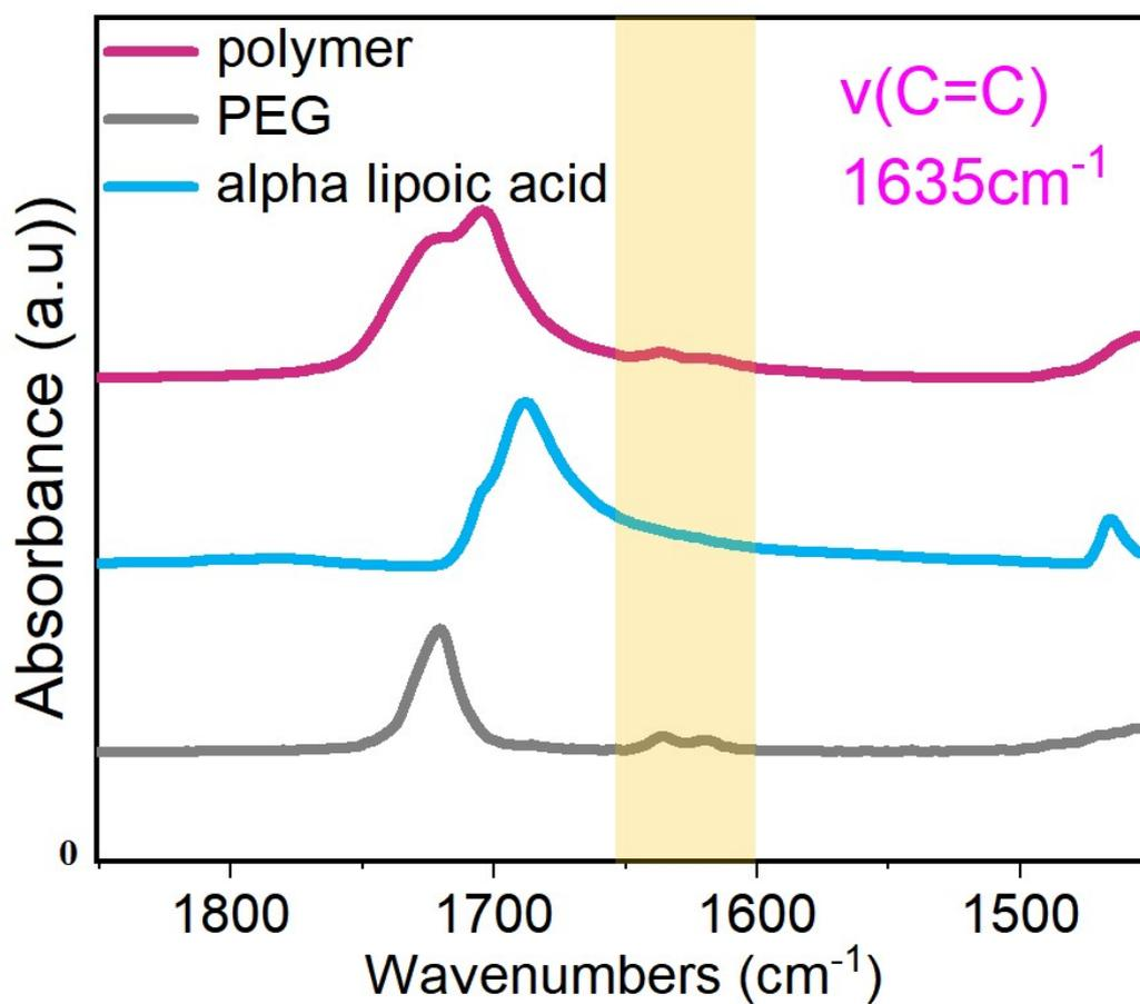
Figure S1. FTIR characterization. The abatement of C=C signal at  $1635\text{cm}^{-1}$ , indicates ring-opening polymerization of lipoic acid, forming the poly (lipoic acid) elastomer.
