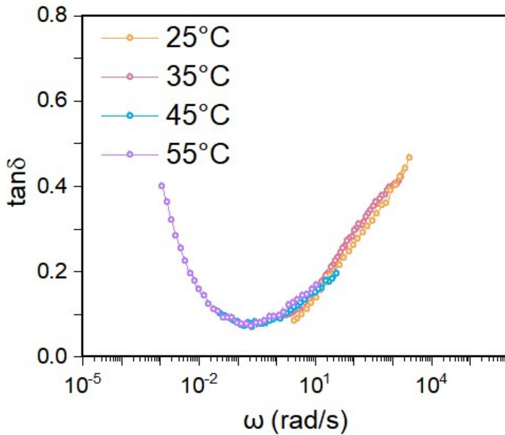
Figure S8. The master curves of loss factor by using the time-temperature superposition of the poly (TA).
