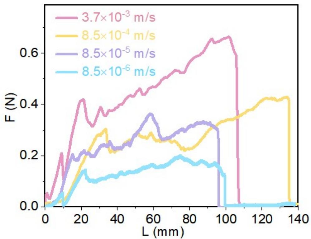
Figure S4. Force–displacement curves of the poly (LA)/Al elastomer composites with different tearing velocities at 25 °C.
