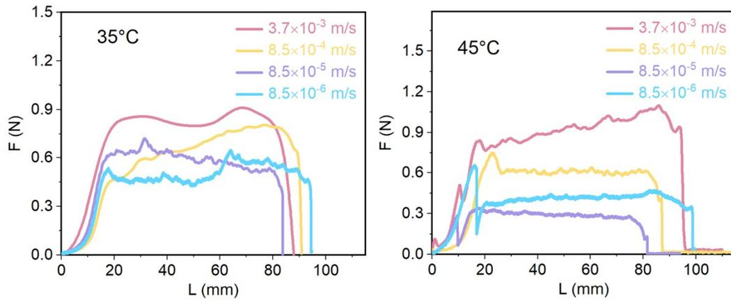
**Figure S12. Force–displacement curves of the poly (LA)/Al@Ag elastomer composites with different tearing velocities at 35 °C and 45 °C.**
