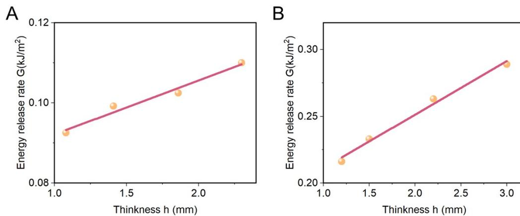
**Figure S6. (A) Energy release rate as a function of thickness of the films with  $8.5 \times 10^{-5} \text{ m s}^{-1}$  of the poly (LA) elastomer. (B) Energy release rate as a function of thickness of the films with  $8.5 \times 10^{-5} \text{ m s}^{-1}$  of the poly (LA)/Al@Ag elastomer.**
