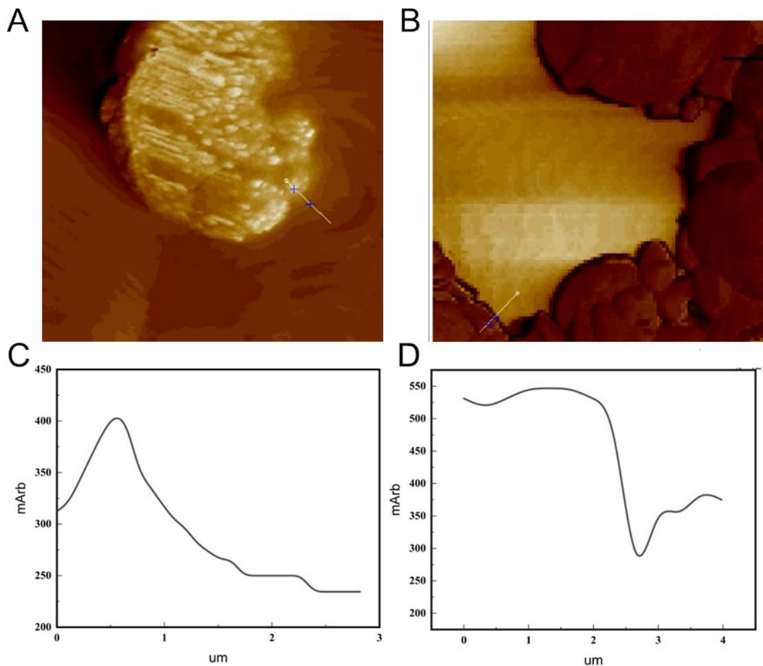
**Figure S15. (A) The AFM image of the poly (LA)/ Al@Ag. (B) The AFM image of the poly (LA)/ Al. (C) The modulus change diagram is obtained by linear scanning of the scribed part of Figure A. (D) The modulus change diagram is obtained by linear scanning of the scribed part of Figure B.**
