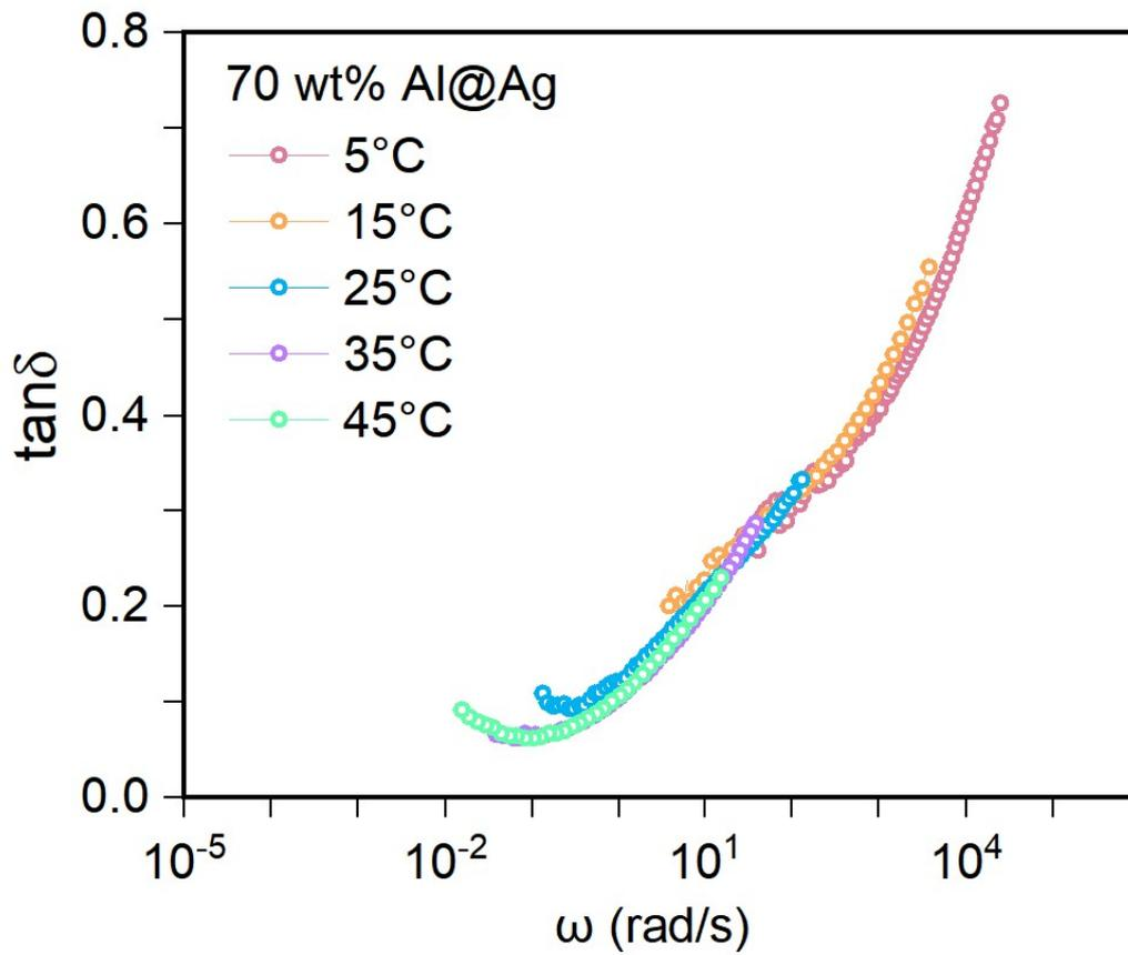
Figure S9. The master curves of loss factor by using the time-temperature superposition of the poly (TA)/Al@Ag.
