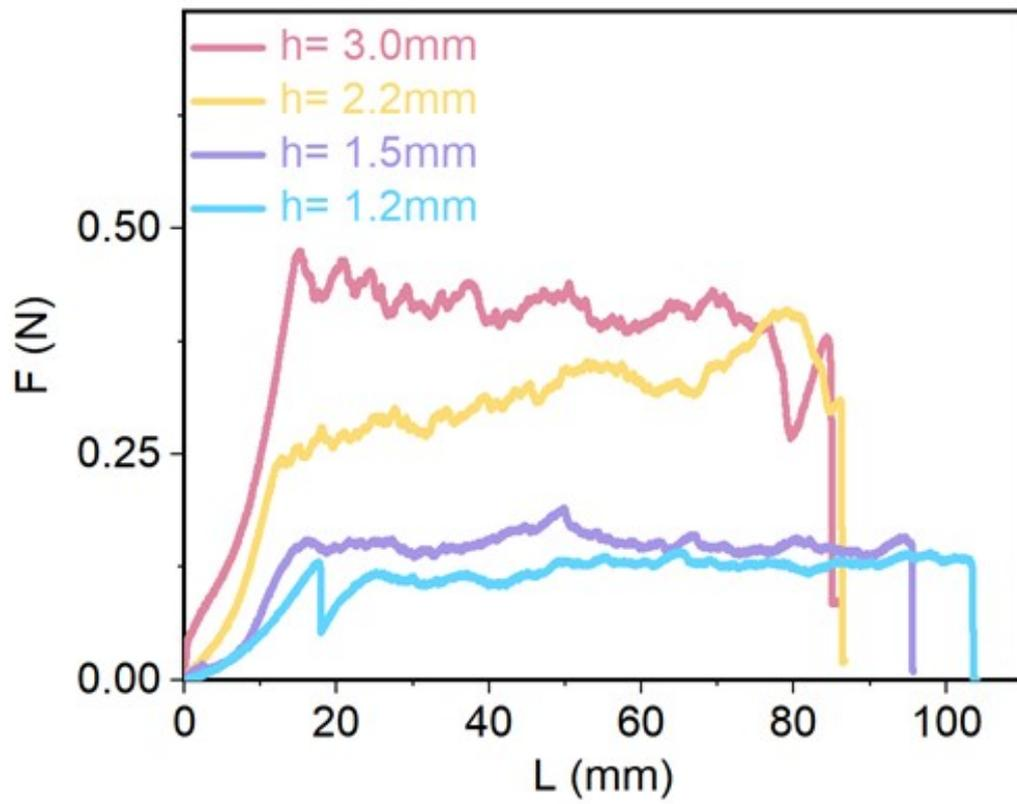
Figure S5. Force–displacement curves of the poly (LA)/Al elastomer composites with  $8.5 \times 10^{-5} \text{ m s}^{-1}$  at 25 °C.
