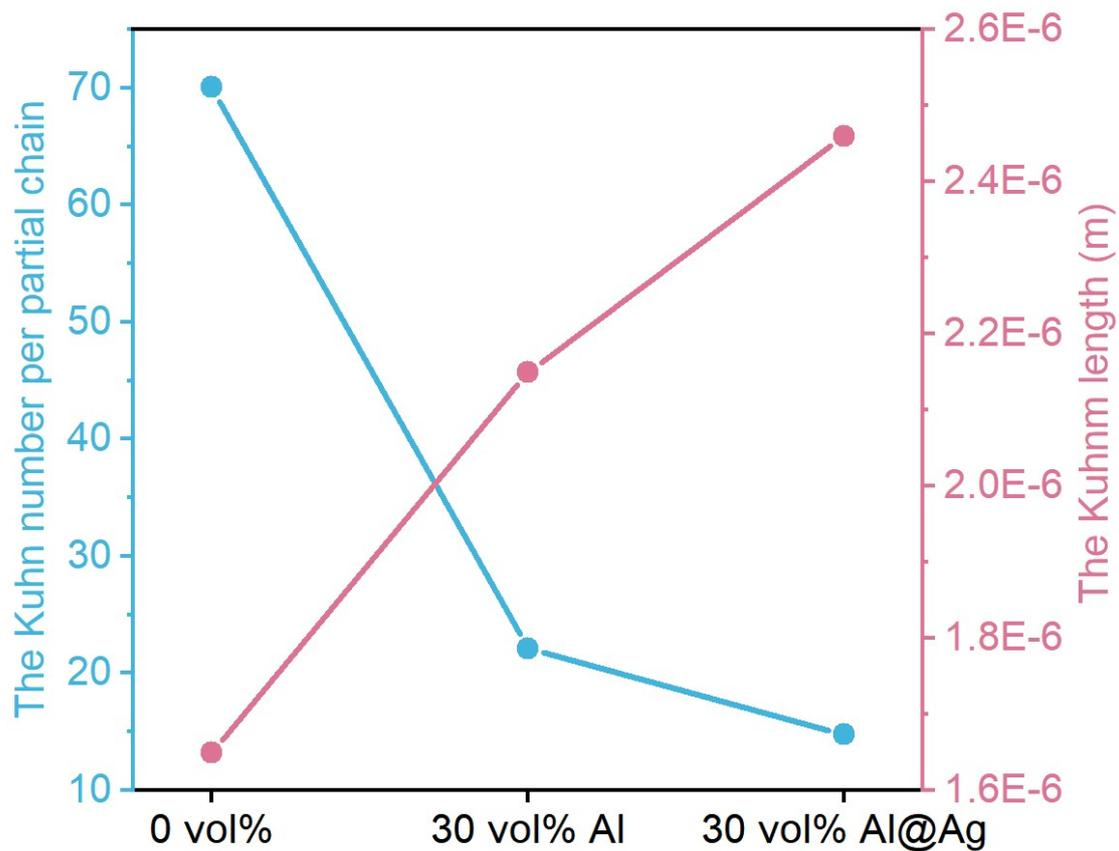
Figure S14. (A) Kuhn number  $N_p$  and Kuhn length  $b_k$  of the elastomer composites with different fillers.
