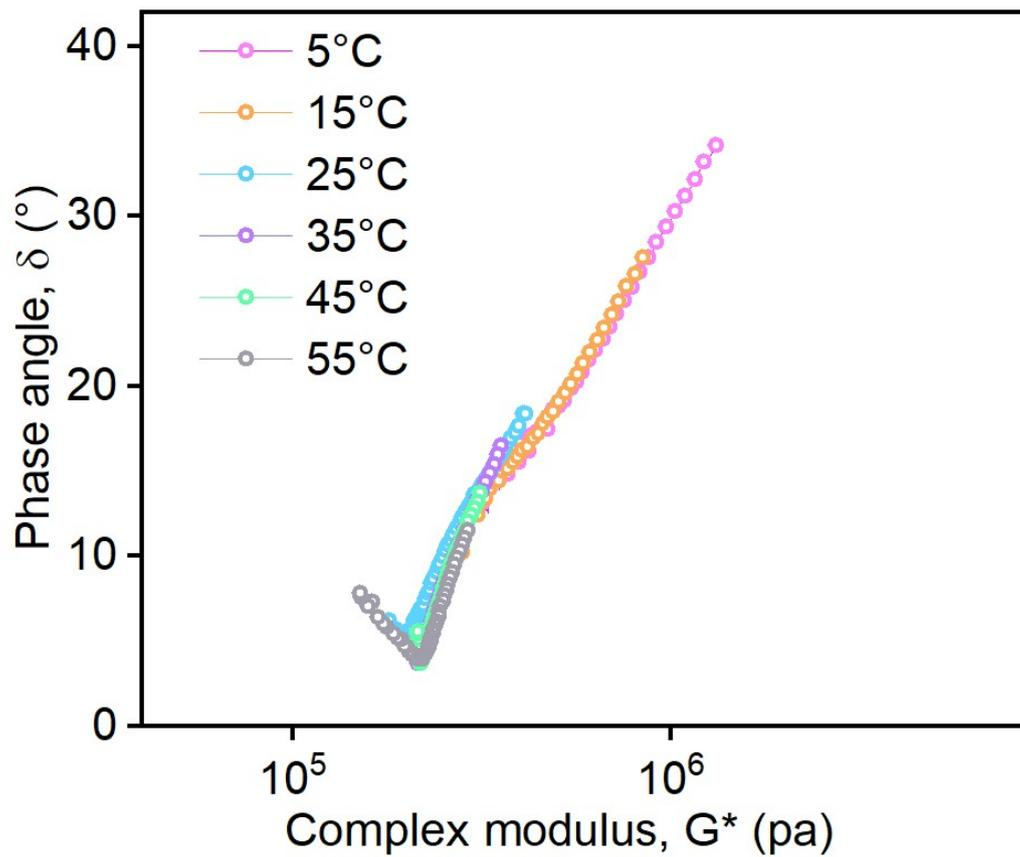
Figure S10. Relationship between the complex modulus  $G^*$  and phase angle  $\delta$  of the poly/Al@Ag composites elastomer.
