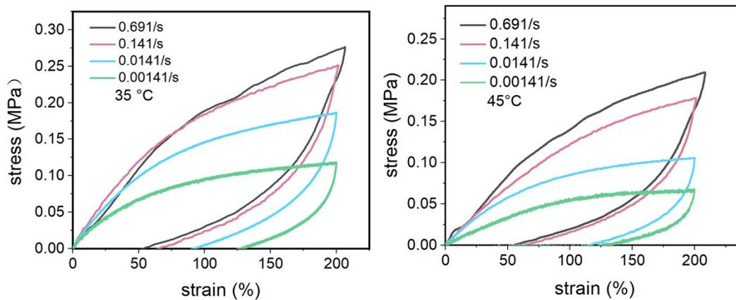
**Figure S11.** The cyclic stress-strain curves of the poly (LA)/Al@Ag elastomer composites under various stretch strain rate at 35 °C and 45 °C.
