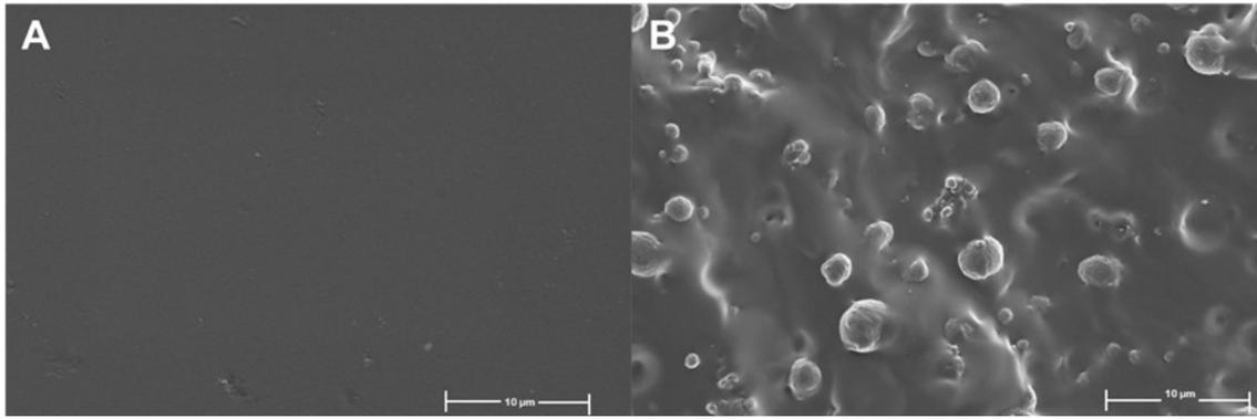
**Figure S7. (A) The SEM image of the poly (LA). (B) The SEM image of the poly (LA)/Al@Ag.**
