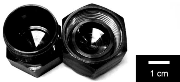
Fig. S2 Photo of the carbon-coated reactor. Due to the small amount of the reactant in each batch of the synthesis, this small reactor is employed, where the carbon coating plays a role same as the Teflon cup in the conventional autoclave.
