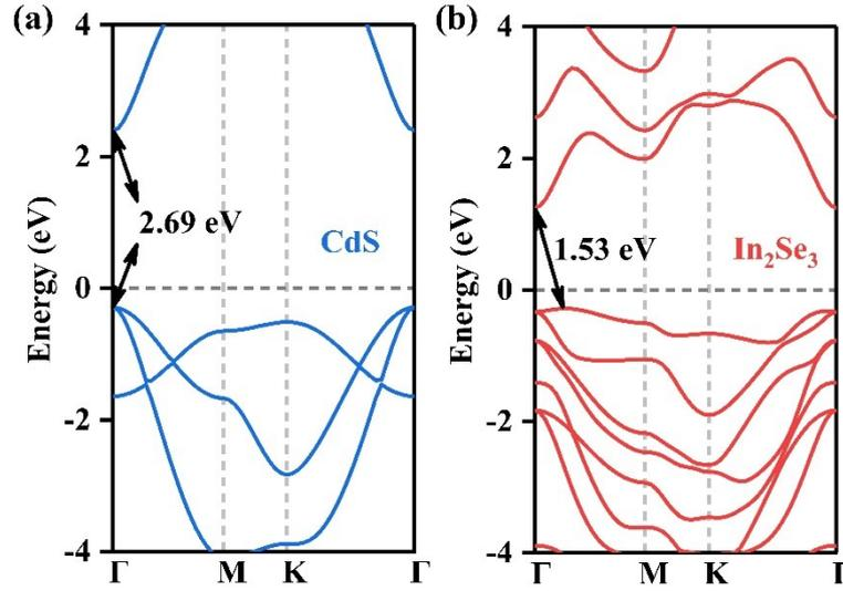
Figure S5 Band structures for (a) CdS and (b) In<sub>2</sub>Se<sub>3</sub>, respectively, on the basis of the HSE06 functional.
