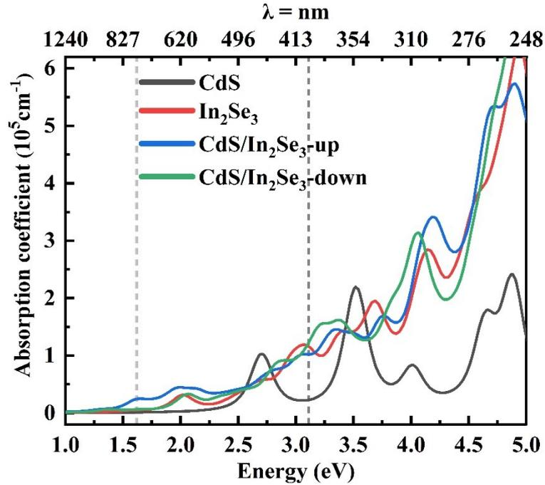
Figure S7 Calculated optical absorption spectra of CdS,  $\text{In}_2\text{Se}_3$ , CdS/ $\text{In}_2\text{Se}_3$ -up and CdS/ $\text{In}_2\text{Se}_3$ -down heterostructures using TDHF.
