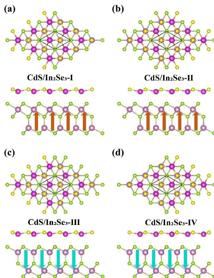
Figure S3 (a-d) Top and side views of the optimized structure for the CdS/In<sub>2</sub>Se<sub>3</sub>-(I-IV) heterostructures.
