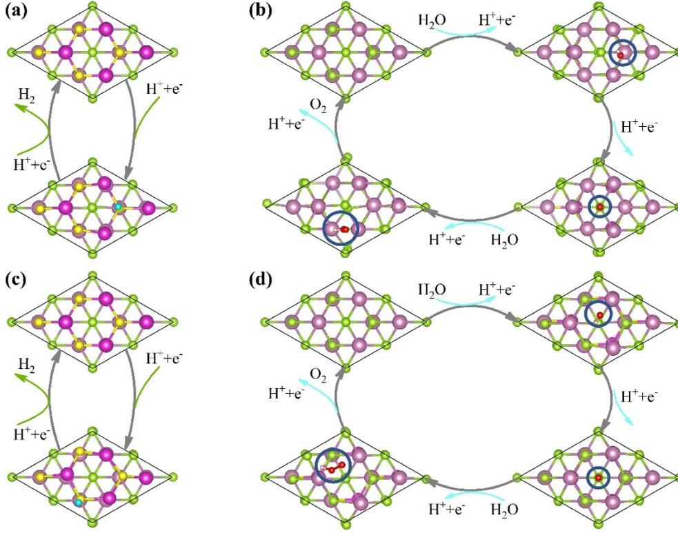
Figure S6 (a) (c) The optimized structures for different hydrogen coverage on the CdS monolayer in CdS/In<sub>2</sub>Se<sub>3</sub>-up and CdS/In<sub>2</sub>Se<sub>3</sub>-down heterostructures, respectively. (b) (d) The optimized structures for OH\*, O\* and OOH\* intermediates for CdS/In<sub>2</sub>Se<sub>3</sub>-up and CdS/In<sub>2</sub>Se<sub>3</sub>-down heterostructures, respectively.
