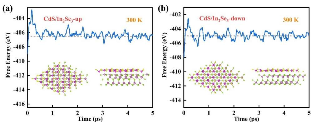
Figure S4 Total potential energies and the corresponding snapshots of (a) CdS/In<sub>2</sub>Se<sub>3</sub>-up and (b) CdS/In<sub>2</sub>Se<sub>3</sub>-down in the AIMD simulations after stabilizing at 300 K for 5 ps.
