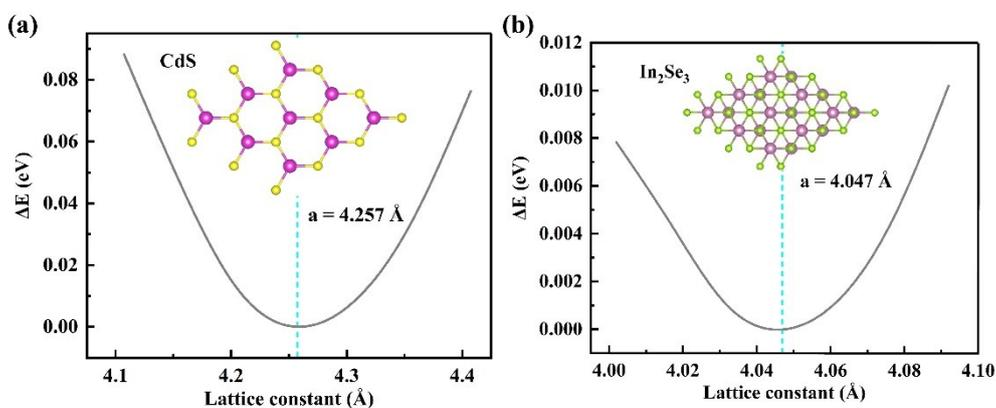
Figure S2 (a) (b) Testing the lattice constants of CdS and In<sub>2</sub>Se<sub>3</sub>, respectively.
