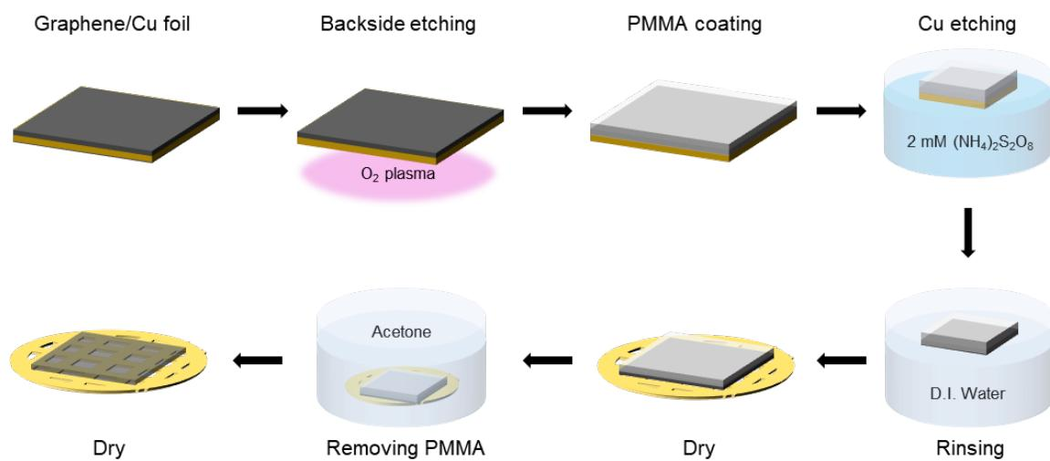
**Figure S1.** Sequence of the preparation steps for the preparation of graphene-coated TEM grids.
