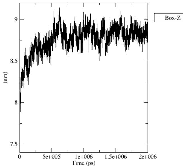
**Fig. S 2.** The equilibrium curve of the phospholipid membrane system with time. The thickness does not change dramatically or fluctuate after about 600ns, which implies that the system has reached equilibrium state.
