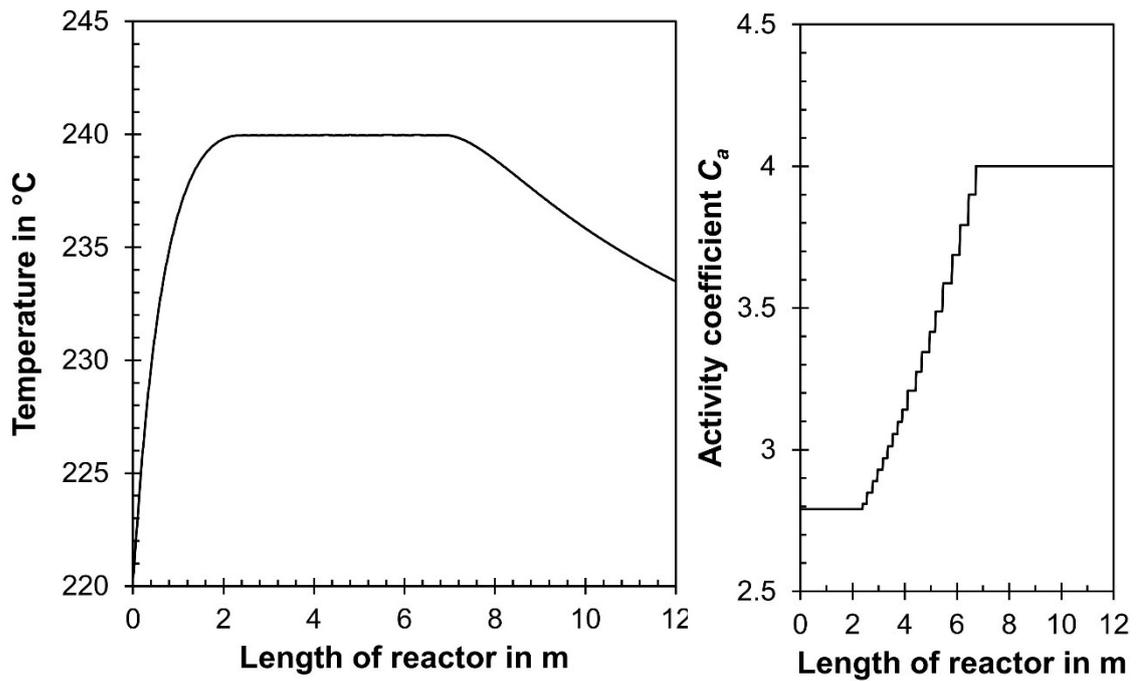
**Fig. S19:** T-profiles ( $r = 0$ ) and grading of activity in a single tube for  $C_{a,initial} = 2.79$  until  $240^\circ\text{C}$  is reached ( $z = 2.5$  m) and then a rise of  $C_a$  to keep the temperature ( $240^\circ\text{C}$  at  $r = 0$ ) constant until  $C_{a,max}$  of 4 is reached at  $z = 6$  m (30 bar;  $X_{CO,total} = 95\%$ ;  $\text{CH}_4$  selectivity = 20%,  $\text{H}_2$ -to-CO ratio = 2.2;  $T_{max} = 240^\circ\text{C}$ ;  $u_{s, z=0} = 1$  m/s; further data in Tab. S3).
