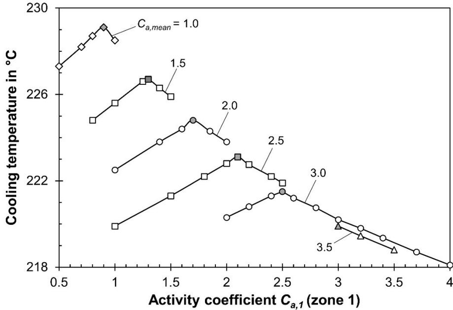
**Fig. S17:** Two-zone FT reactor with zones of equal length (6 m): Influence of activity coefficient  $C_{a,1}$  on  $T_{cool}$  for different mean activities  $C_{a,mean}$ . Filled symbols represent case that maximum yield is reached, see also Fig. S16 ( $p_{total} = 30$  bar;  $u_s = 1$  m/s;  $\text{CH}_4$  selectivity = 20%;  $\text{H}_2$ -to-CO ratio = 2.2;  $T_{max} = 240^\circ\text{C}$ ).
