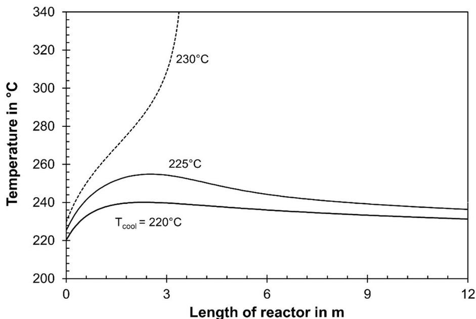
**Fig. S9:** Axial temperature profiles in the center of the single tube ( $r = 0$ ) for three different cooling temperatures. For  $T_{cool} = 230^{\circ}\text{C}$  (dashed-dotted line), thermal runaway occurs ( $C_a = 3$ ;  $p_{total} = 30$  bar;  $u_s = 1$  m/s;  $X_{CO,total} = 95\%$ ;  $\text{CH}_4$  selectivity = 20%;  $\text{H}_2$ -to-CO ratio = 2.2;  $T_{max} = 240^{\circ}\text{C}$ ).
