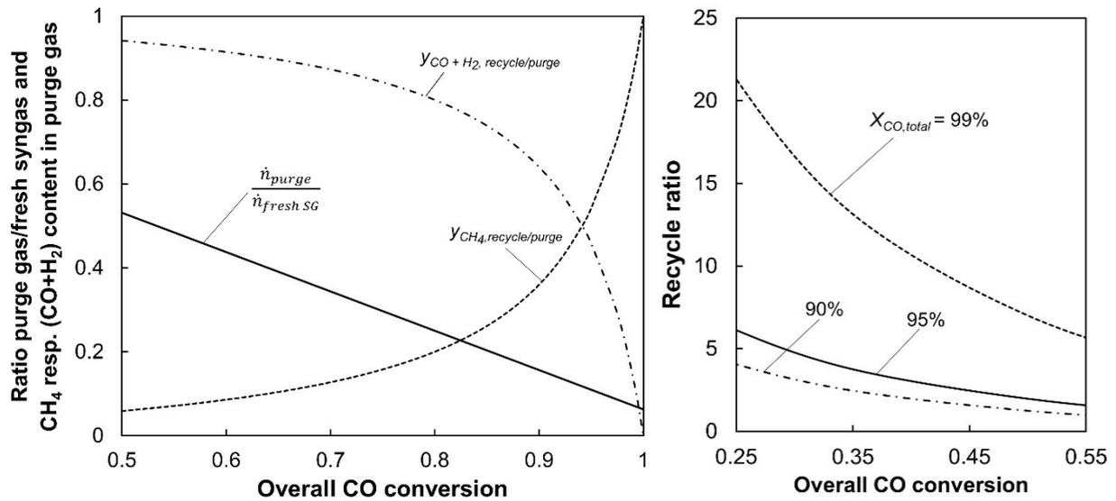
**Fig. S1:** Influence of overall CO conversion ( $X_{CO,total}$ ) on the ratio of purge gas stream to the stream of fresh syngas and on the CH<sub>4</sub> and combined CO/H<sub>2</sub> content in the recycle and purge gas of a FT reactor (left) and on the recycle ratio  $R$  (right) (CH<sub>4</sub> selectivity = 20%, H<sub>2</sub>-to-CO ratio = 2.2).
