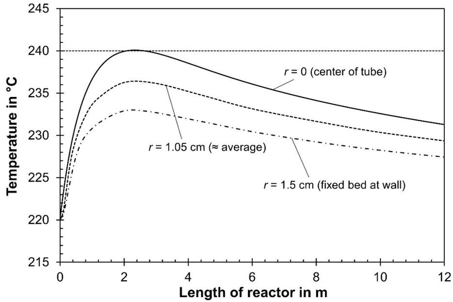
**Fig. S7:** Axial temperature profiles in the center of the single tube ( $r = 0$ ), at the position  $r = 1.05$  cm, and in the fixed bed directly at the wall ( $r = 1.5$  cm) ( $C_a = 3$ ;  $p_{total} = 30$  bar;  $u_s = 1$  m/s;  $X_{CO,total} = 95\%$ ;  $CH_4$  selectivity = 20%;  $H_2$ -to-CO ratio = 2.2;  $T_{max} = 240^\circ C$ ).
