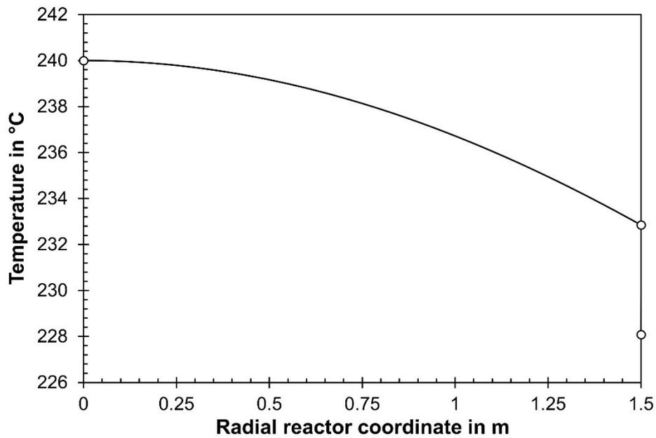
**Fig. S8:** Radial temperature profile at the position of the axial temperature maximum ( $z = 2.2$  m) ( $C_a = 3$ ;  $p_{total} = 30$  bar;  $u_s = 1$  m/s;  $X_{CO,total} = 95\%$ ;  $CH_4$  selectivity = 20%;  $H_2$ -to-CO ratio = 2.2;  $T_{max} = 240^\circ C$ ).
