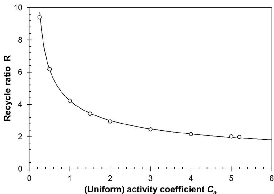
**Fig. S5:** Influence of (uniform) axial activity  $C_a$  on recycle ratio of FT reactor ( $p_{total} = 30$  bar;  $u_s = 1$  m/s;  $X_{CO,total} = 95\%$ ;  $CH_4$  selectivity = 20%;  $H_2$ -to-CO ratio = 2.2;  $T_{max} = 240^\circ C$ ).
