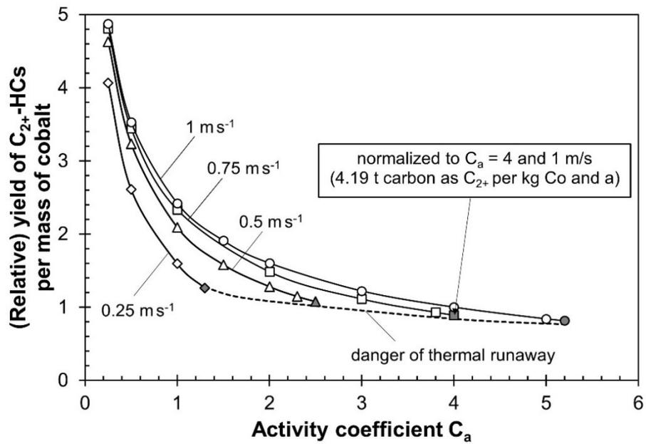
**Fig. S3:** Influence of the activity coefficient  $C_a$  on the (relative) yield of  $C_{2+}$ -HCs per mass of cobalt at different superficial gas velocities  $u_s$  ( $p_{total} = 30$  bar;  $X_{CO, total} = 95\%$ ;  $CH_4$  selectivity = 20%;  $H_2$ -to-CO ratio = 2.2;  $T_{max} = 240^\circ C$ ). Filled symbols represent critical cases with regard to thermal runaway.
