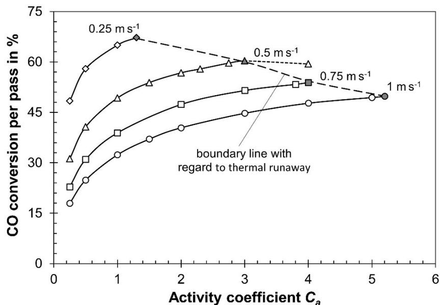
**Fig. S2:** Influence of activity coefficient  $C_a$  on the CO conversion per pass for different values of  $u_s$  ( $p_{total} = 30$  bar;  $X_{CO,total} = 95\%$ ;  $CH_4$  selectivity = 20%;  $H_2$ -to-CO ratio = 2.2;  $T_{max} = 240^\circ C$  except for 0.5 m/s and  $C_a = 4$  with  $T_{cool} = 208^\circ C$  and  $T_{max} = 235^\circ C$ ). Filled symbols: critical cases with regard to thermal runaway ( $T_{max} = 240^\circ C$ ).
