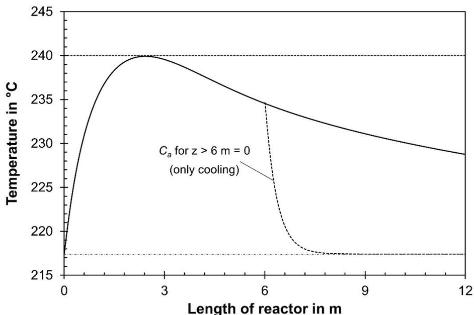
**Fig. S11:** Axial temperature profile in a single tube of a FT reactor with constant catalytic activity ( $C_a = 4$ ). The dotted line indicates the T-profile for the hypothetical case of no activity in the second part of the tube ( $C_a = 4$  for  $z > 6$  m) to show the high intensity of cooling in a multi-tubular FT-reactor ( $p_{total} = 30$  bar;  $u_s = 1$ ).
