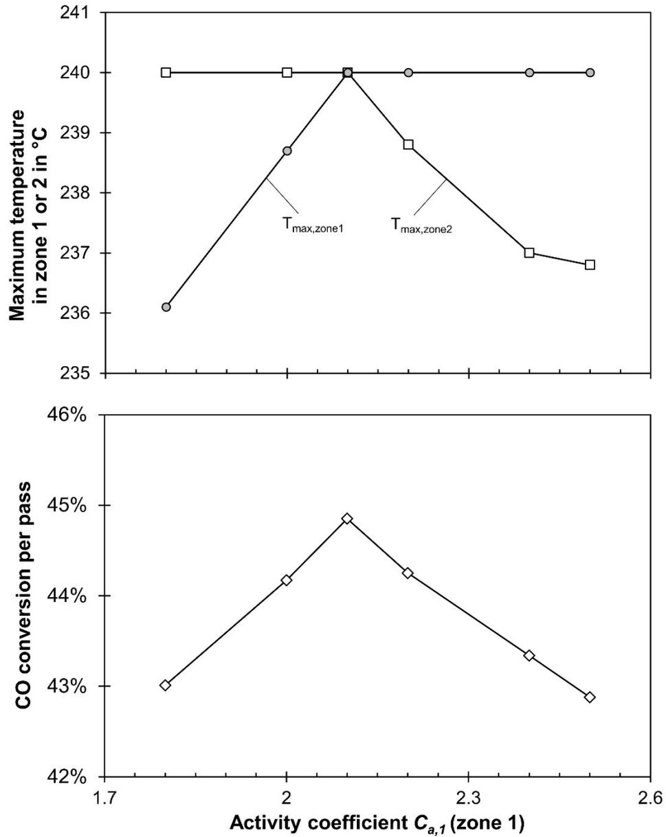
**Fig. S14:** Maximum axial temperatures in both zones of a two-zone FT reactor (top) and CO-conversion per pass (bottom) for a variation of  $C_{a,1}$  and a constant value of  $C_{a,mean}$  of 2.5, i.e.  $C_{a,2} = 5 - C_{a,1}$  ( $p_{total} = 30$  bar;  $u_s = 1$  m/s;  $\text{CH}_4$  selectivity = 20%;  $\text{H}_2$ -to-CO ratio = 2.2).
