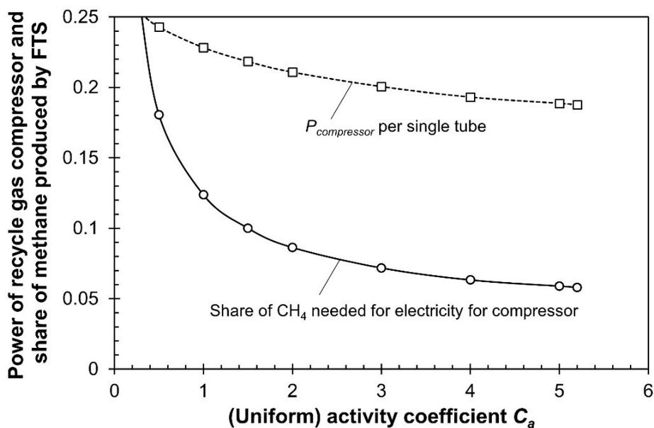
**Fig. S6:** Influence of (uniform) axial activity  $C_a$  on the power of the recycle gas compressor and on the share of methane produced by FTS (as a simple measure for the electrical energy need for gas recycling assuming an efficiency of power production of 40%) ( $p_{total} = 30$  bar;  $\Delta p = 6$  bar;  $u_s = 1$  m/s;  $X_{CO,total} = 95\%$ ;  $CH_4$  selectivity = 20%;  $H_2$ -to-CO ratio = 2.2;  $T_{max} = 240^\circ C$ ).
