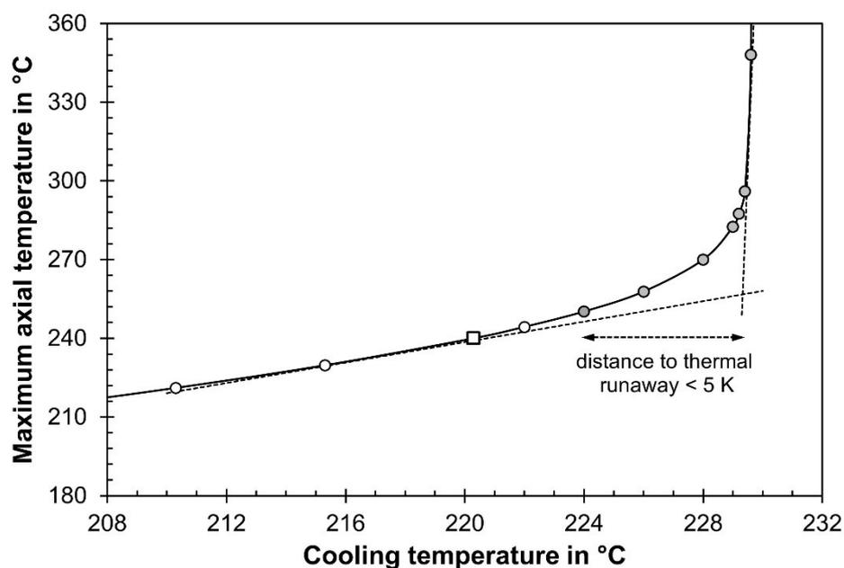
**Fig. S10:** Influence of  $T_{cool}$  on  $T_{max}$  (center of tube) at axial position of around  $z = 2$  m, where maximum axial temperature is reached (see Fig. S9). Thermal runaway occurs for  $T_{cool}$  of about  $230^{\circ}\text{C}$ ; hence,  $T_{cool}$  should be  $225^{\circ}\text{C}$  ( $C_a = 3$ ;  $p_{total} = 30$  bar;  $u_s = 1$  m/s;  $X_{CO,total} = 95\%$ ;  $\text{CH}_4$  selectivity = 20%; molar  $\text{H}_2$ -to-CO ratio = 2.2;  $T_{max} = 240^{\circ}\text{C}$ ).
