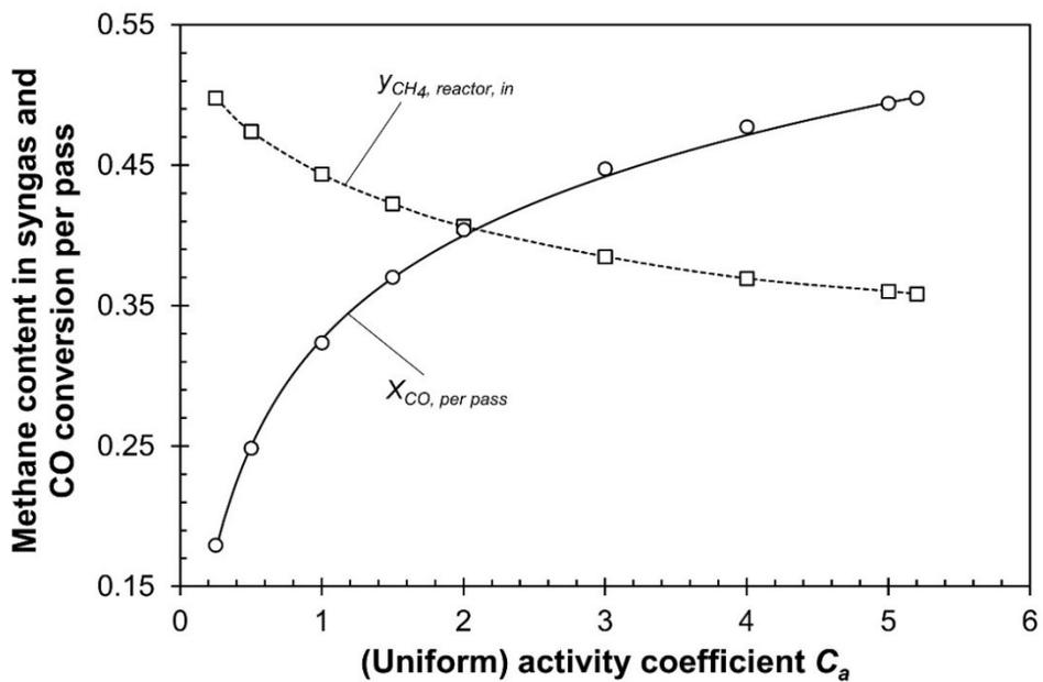
**Fig. S4:** Influence of (uniform) axial activity  $C_a$  on methane content in syngas entering the FT reactor and on the CO conversion per pass ( $p_{total} = 30$  bar;  $u_s = 1$  m/s;  $X_{CO, total} = 95\%$ ;  $CH_4$  selectivity = 20%;  $H_2$ -to-CO ratio = 2.2;  $T_{max} = 240^\circ C$ ).
