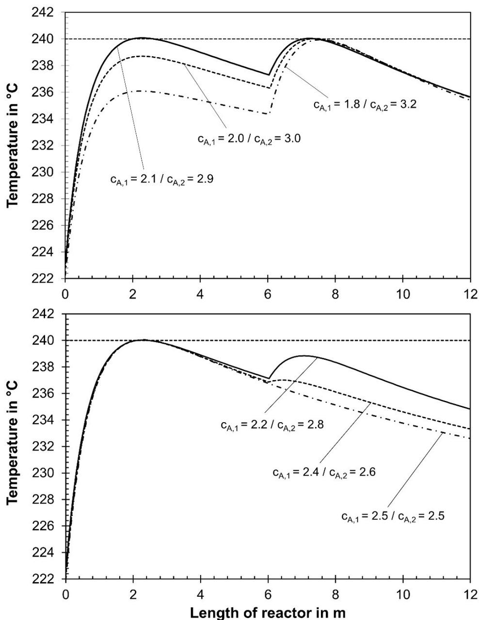
**Fig. S13:** Axial temperature profiles in a two-zone FT reactor with two catalytic zones of equal length (6 m) for different values of the activities  $C_{a,1}$  and  $C_{a,2}$  and a constant mean activity  $C_{a,mean}$  of 2.5. The corresponding values of the yield of  $C_{2+}$ -HCs are shown in Fig. S11 ( $p_{total} = 30$  bar;  $u_s = 1$  m/s;  $CH_4$  selectivity = 20%;  $H_2$ -to-CO ratio = 2.2;  $T_{max} = 240^\circ C$ ).
