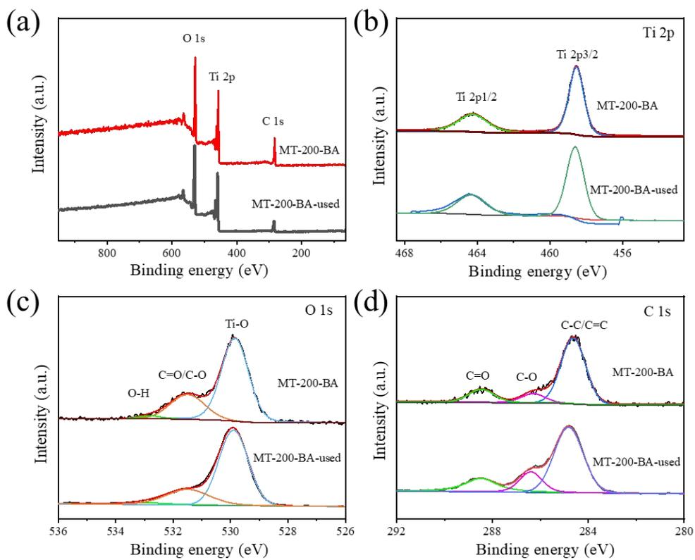
**Fig. S14** (a) XPS survey spectra, (b) Ti 2p, (c) O 1s and (d) C 1s spectra of MT-200-BA and MT-200-BA-used samples.
