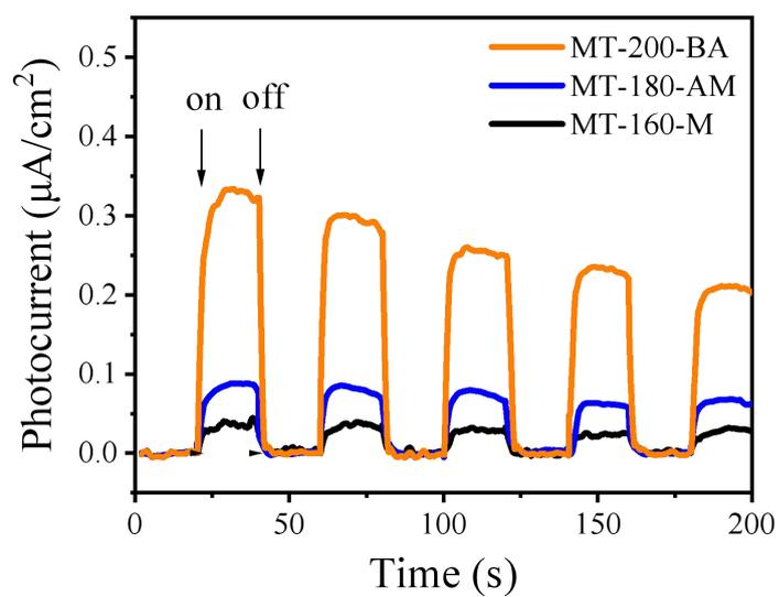
**Fig. S9** Transient photocurrent measurements for MT-160-M, MT-180-AM and MT-200-BA on FTO substrate in a 0.2 M  $\text{Na}_2\text{SO}_4$  electrolyte.
