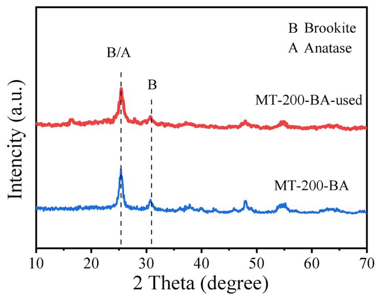
**Fig. S13** XRD patterns of MT-200-BA and MT-200-BA-used samples.
