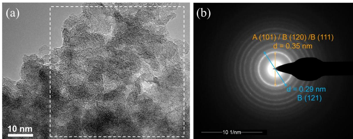
**Fig. S5** (a) TEM image and (b) SAED pattern of the MT-200-BA sample
