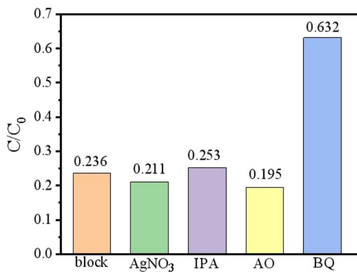
**Fig. S15** Trapping experiments of active species during photocatalytic degradation of TCH (100 mg/L) over MT-200-BA under Xe light irradiation.
