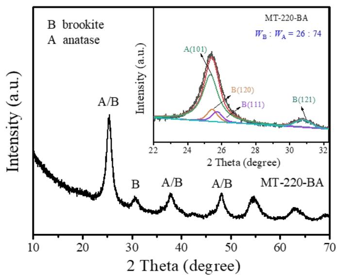
**Fig. S10** XRD pattern of the MT-220-BA reference sample prepared at solvothermal temperature of 220 °C, the inset is deconvolution of XRD pattern of MT-220-BA.
