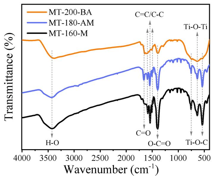
**Fig. S6** FT-IR spectra of MT-160-M, MT-180-AM and MT-200-BA.
