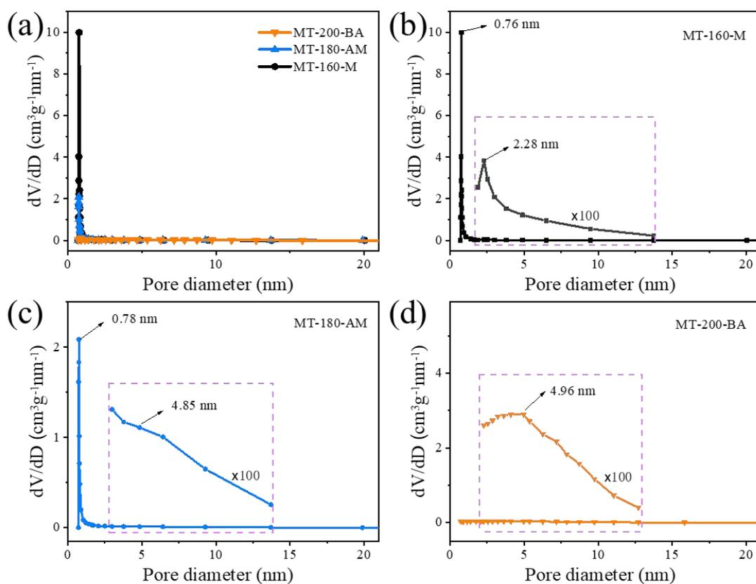
**Fig. S2** (a) The pore size distributions and separately magnified curves of MT-160-M (b), MT-180-AM (c) and (d) MT-200-BA samples.
