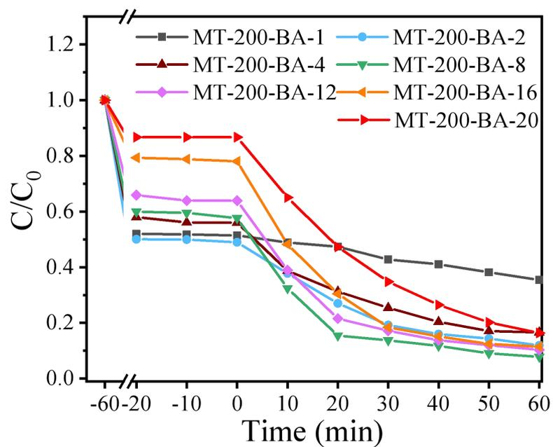
**Fig. S12** Photocatalytic degradation of TCH over various MT-200-BA-X samples at a concentration of 100 mg L<sup>-1</sup>.
