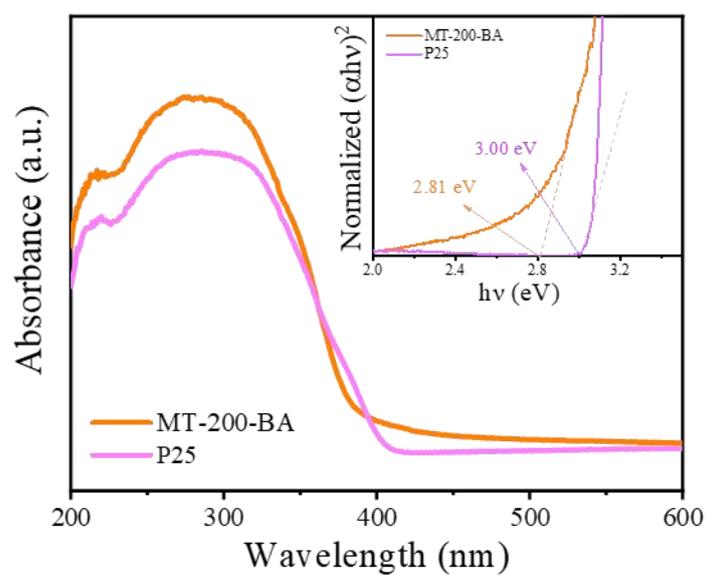
**Fig. S7** UV-vis DRS spectra of P25 and MT-200-BA, and corresponding band gap energies calculated by using the Tauc plot method (inset).
