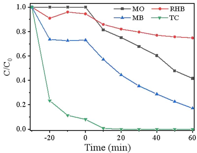
**Fig. S11** Photocatalytic degradation of MO, RHB, MB and TCH pollutants in solution ( $20 \text{ mg L}^{-1}$ ) upon MT-200-BA sample.
