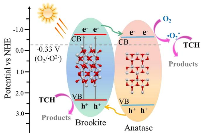
**Fig. S16** The possible mechanism schematic for photocatalytic TCH degradation upon MT-200-BA under light irradiation.
