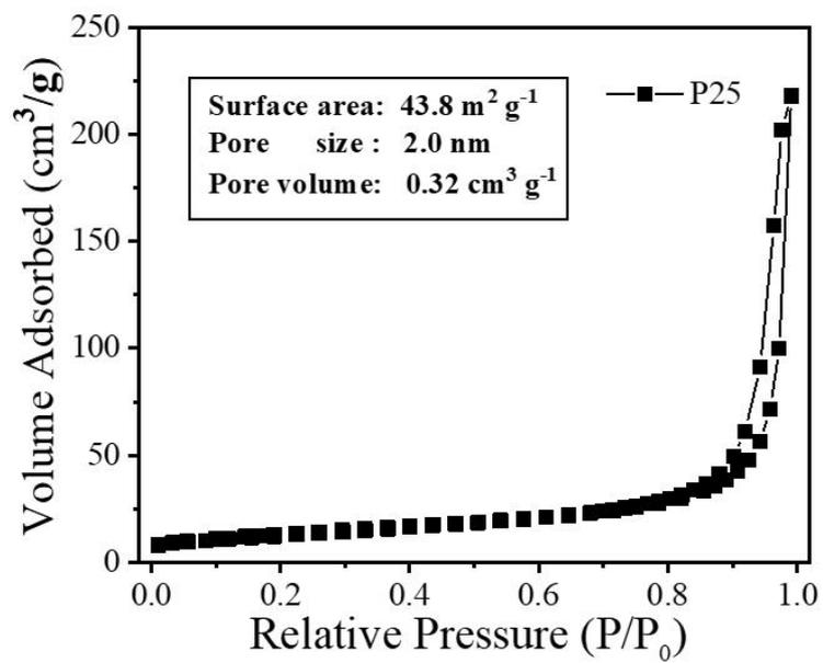
**Fig. S3**  $\text{N}_2$  adsorption-desorption isotherms of commercial P25 catalyst.
