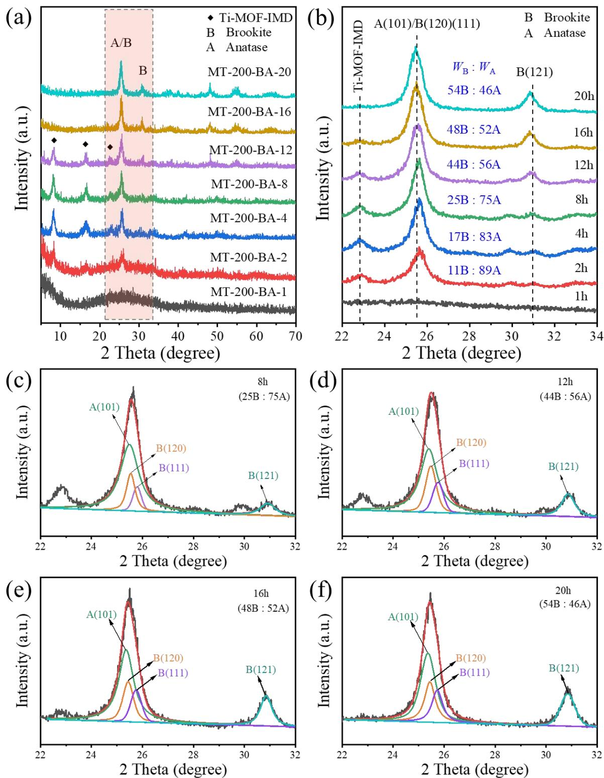
**Fig. S1** (a) Wide angle XRD and (b) selected range slow scanning XRD patterns of MT-200-BA-X (X = 1, 2, 4, 8, 12, 16 and 20) samples prepared at different synthesis times, and deconvolution of XRD patterns of MT-200-BA-8 (c), MT-200-BA-12 (d), MT-200-BA-16 (e) and MT-200-BA-20 (f).
