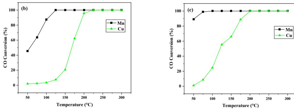
Fig. 2. (a) Conversion rate of NO<sub>x</sub> in CO-SCR reaction, reaction conditions: 1000 ppm CO, 500 ppm NO, 5% O<sub>2</sub>, balanced N<sub>2</sub>; GHSV = 30,000 h<sup>-1</sup>. (b) Conversion rate of CO in CO-SCR reaction, reaction conditions same as (a). (c) Conversion rate of CO in CO oxidation reaction, reaction conditions: 1000 ppm CO, 5% O<sub>2</sub>, balanced N<sub>2</sub>; GHSV = 30,000 h<sup>-1</sup>.
