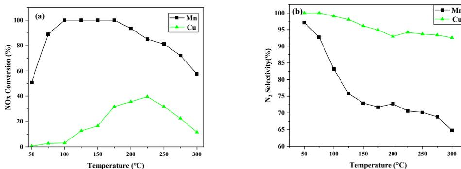
Fig. 1, The catalytic performance of transition metal oxide catalysts in NH<sub>3</sub>-SCR, (a) conversion rate of NO<sub>x</sub>, (b) N<sub>2</sub> selectivity, under the reaction conditions of 500 ppm NH<sub>3</sub>, 500 ppm NO, 5% O<sub>2</sub>, N<sub>2</sub> balance; GHSV = 30,000 h<sup>-1</sup>.
