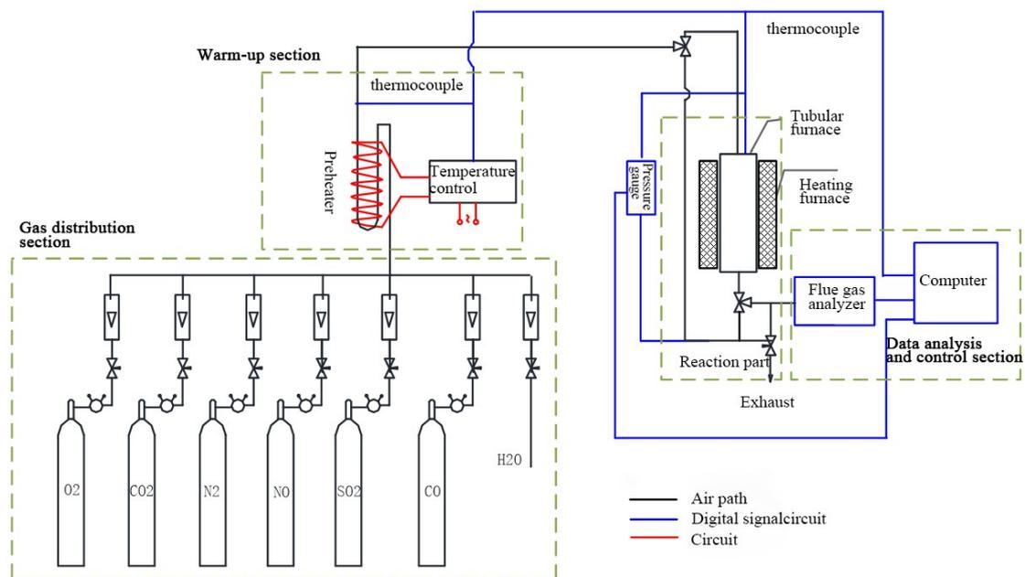
Schematic diagram of fixed bed reaction system.
