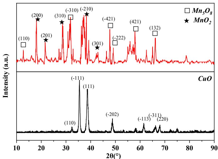
Fig. 3. XRD spectra of single metal oxide Mn and Cu catalysts.
