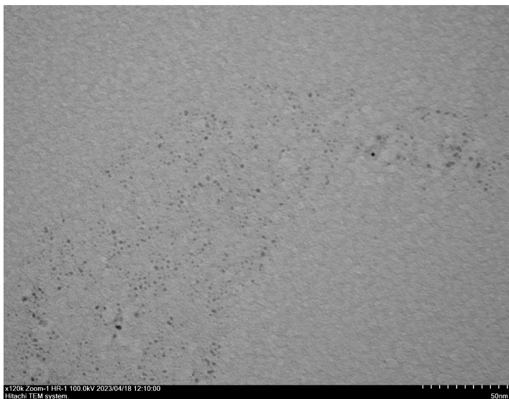
Figure S8. Pt particles captured from \text{Pt}_2\text{dba}_3 in benzene- \text{d}_6 after heating for 18 h at 70 °C.
