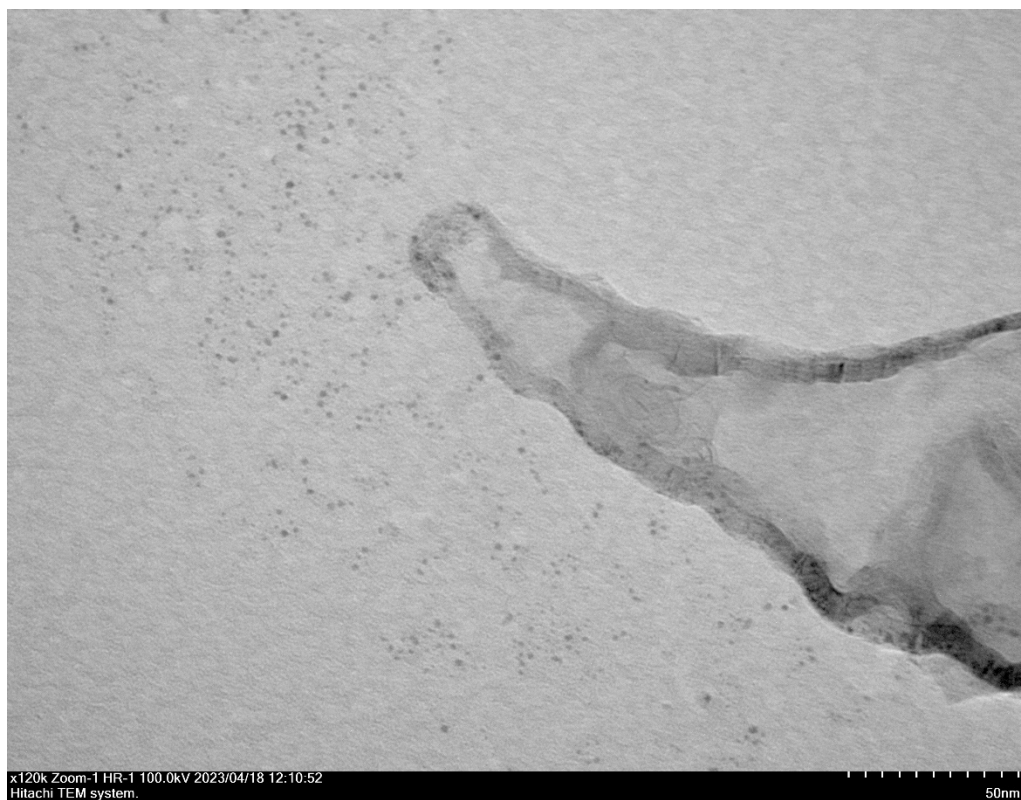
Figure S9. Pt particles captured from \text{Pt}_2\text{dba}_3 in benzene- \text{d}_6 after heating for 18 h at 70 °C.
