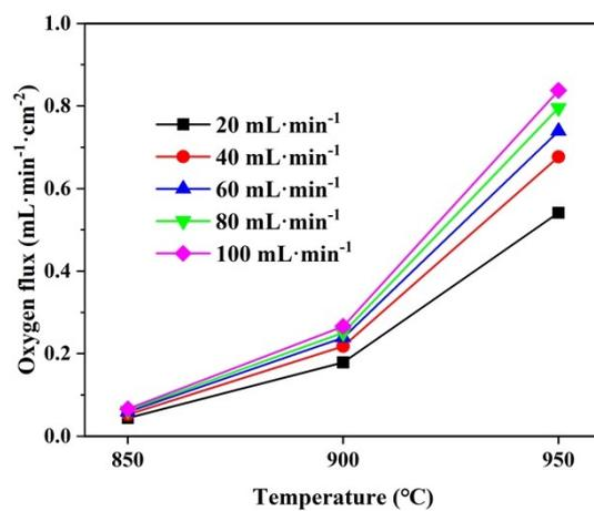
Fig. S5 Effect of He sweep flow rate on oxygen flux of LCAF-SDC hollow fiber membrane as a function of temperature (Air feed flow rate was 100 mL min<sup>-1</sup>).
