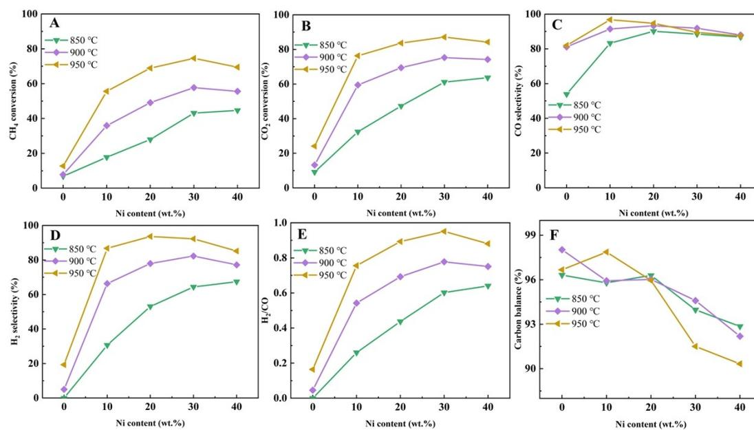
Fig. S3 DRM catalytic performance of catalysts with different Ni contents: (A) CH<sub>4</sub> and (B) CO<sub>2</sub> conversion, (C) CO and (D) H<sub>2</sub> selectivity, (E) H<sub>2</sub>/CO molar ratio, and (F) carbon balance (feed gas was 50 mL min<sup>-1</sup> CH<sub>4</sub> and 50 mL min<sup>-1</sup> CO<sub>2</sub>).
