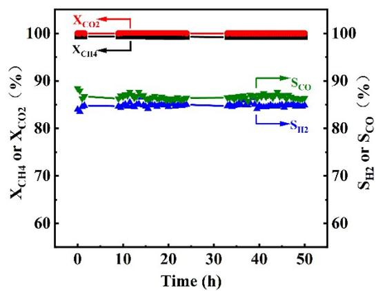
Fig. S6 DRM stability of SDC-LCAF HFM reactor at 900 °C (flow rate of CH<sub>4</sub>-CO<sub>2</sub>-He was 10-10-20 mL min<sup>-1</sup>, respectively).
