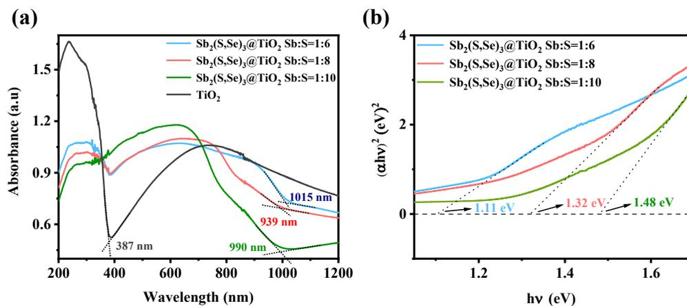
**Fig. S5.** (a) UV-vis-NIR spectra of  $\text{Sb}_2(\text{S,Se})_3@ \text{TiO}_2$  at different S concentrations, (b) Semiconductor band gap of  $\text{Sb}_2(\text{S,Se})_3@ \text{TiO}_2$  at different S concentrations.
