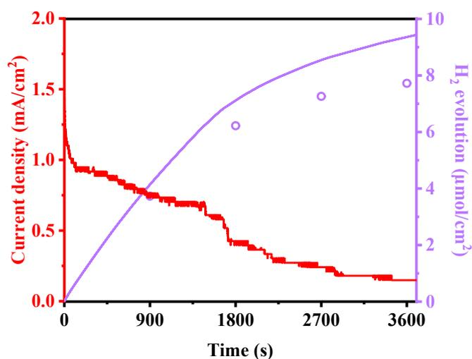
**Fig. S7.**  $\text{H}_2$  evolution curve and the concurrent J-t curve of  $\text{Sb}_2(\text{S,Se})_3@/\text{TiO}_2$  at 1.23 V vs. RHE in 0.5 M  $\text{Na}_2\text{SO}_4$  under AM 1.5G illumination.
