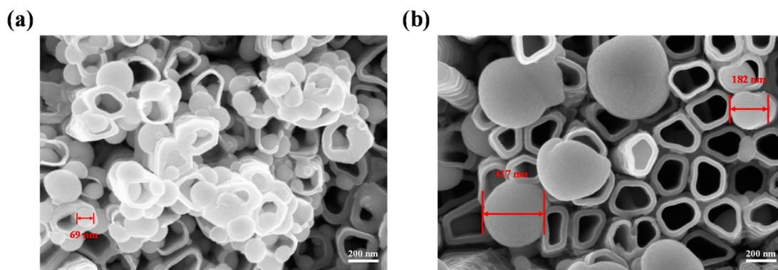
**Fig. S2.** (a) SEM image of  $\text{Sb}_2(\text{S,Se})_3@ \text{TiO}_2$  at low concentrations of Se, (b) SEM image of  $\text{Sb}_2(\text{S,Se})_3@ \text{TiO}_2$  at high concentrations of Se.
