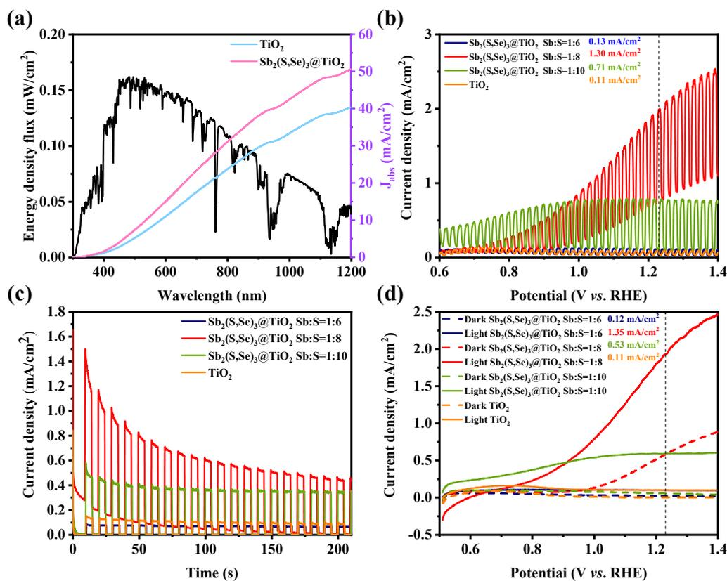
**Fig. S6.** (a) The current density fluxes and integrated current densities ( $J_{\text{abs}}$ ) of monomers  $\text{TiO}_2$  and  $\text{Sb}_2(\text{S,Se})_3@/\text{TiO}_2$  heterojunctions were calculated, (b) J-V curves of  $\text{TiO}_2$  NTs of the different samples, (c) J-t curves of  $\text{TiO}_2$  NTs of the different samples, (d) LSV curves under full on or full off light.
