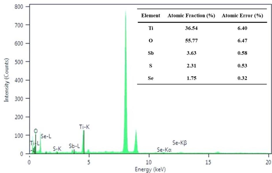
**Fig. S3.** EDS spectrum of  $\text{Sb}_2(\text{S,Se})_3@ \text{TiO}_2$ .
