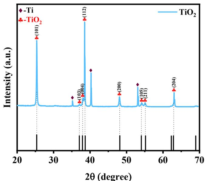
Fig. S1. The XRD diagram of monomeTiO<sub>2</sub>.
