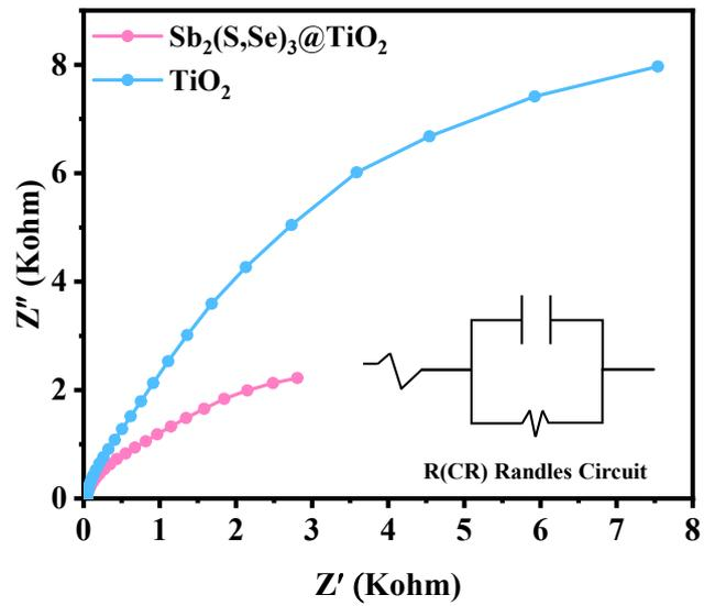
**Fig. S8.** Nyquist plots (EIS) under AM 1.5G illumination, the equivalent circuit model is shown in the illustration for data fitting.
