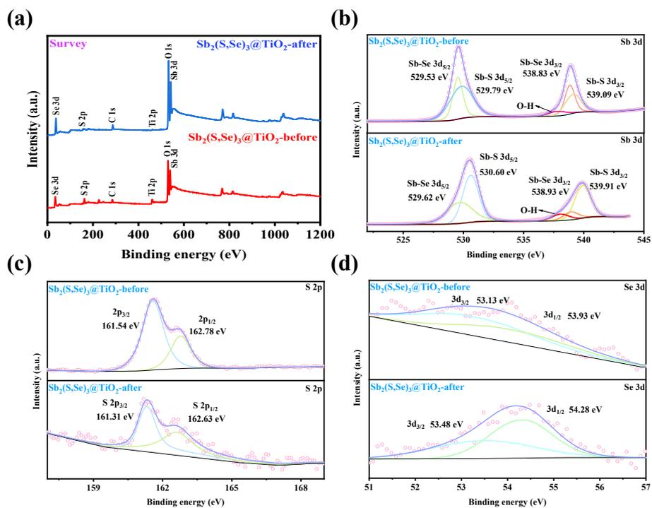
**Fig. S4.** (a) XPS survey spectrum, (b) Sb 3d, (c) S 2p and (d) Se 3d high-resolution XPS spectra for  $\text{Sb}_2(\text{S,Se})_3@ \text{TiO}_2$  photoanodes before and after test.
