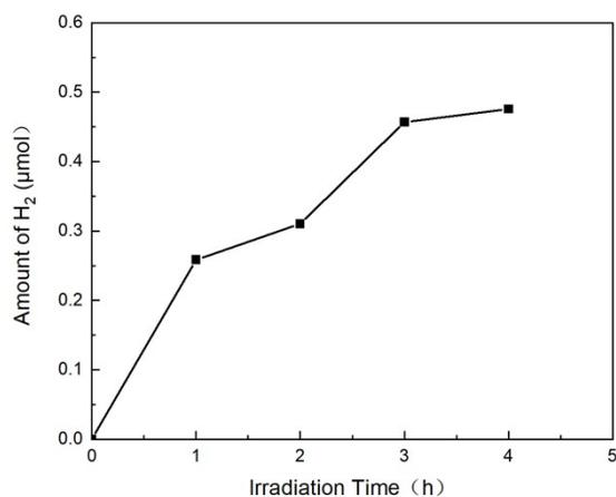
The formation of H<sub>2</sub> over Pt modified CdS in the reaction system has been tentatively measured by offline GC (TCD detector, N<sub>2</sub> as carrier gas). As it shown, a consistent increase of H<sub>2</sub> amount could be observe in the system, suggesting the H<sub>2</sub> evolution is a competing reaction of reduction of NB.
