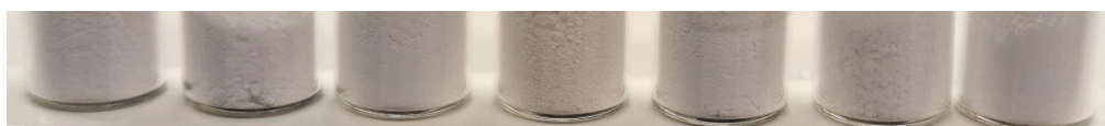
Figure S3: Picture of the zeolite catalysts used in this study. From left to right: H-Y-30, H-BEA-25, H-FER-20, H-MOR-20, H-ZSM-5-30, H-ZSM-5-80 and H-ZSM-5-280.
