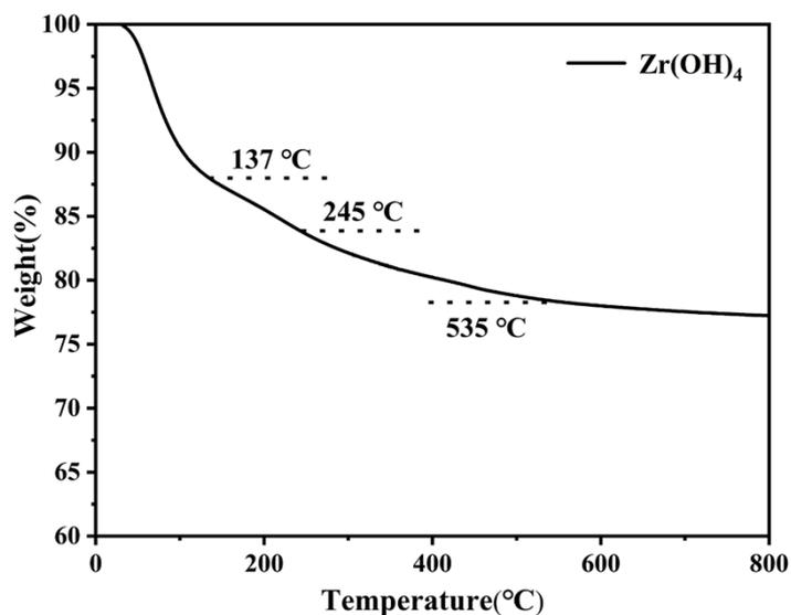
**Figure S4.** TGA curve of the Zr(OH)<sub>4</sub> catalyst.
