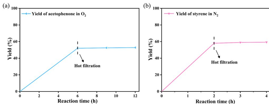
**Figure S5.** Hot filtration experiments of Zr(OH)<sub>4</sub> by continuing the reaction after filtration of the catalyst. Reaction conditions: (a) 1-phenylethanol (1 mmol), Zr(OH)<sub>4</sub> (50 mg), solvent (toluene 5 mL), 800 rpm, 150 °C, 1 MPa O<sub>2</sub>. (b) 1-phenylethanol (1 mmol), Zr(OH)<sub>4</sub> (50 mg), solvent (dichloromethane 5 mL), 800 rpm, 150 °C, 1 MPa N<sub>2</sub>.
