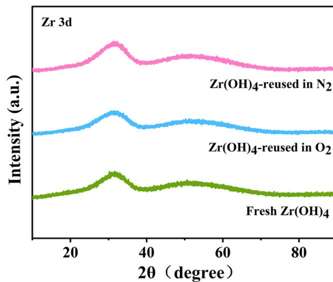
**Figure S2.** XRD patterns of fresh  $\text{Zr(OH)}_4$  and six times reused  $\text{Zr(OH)}_4$  after oxidative dehydrogenation and dehydration reaction.
