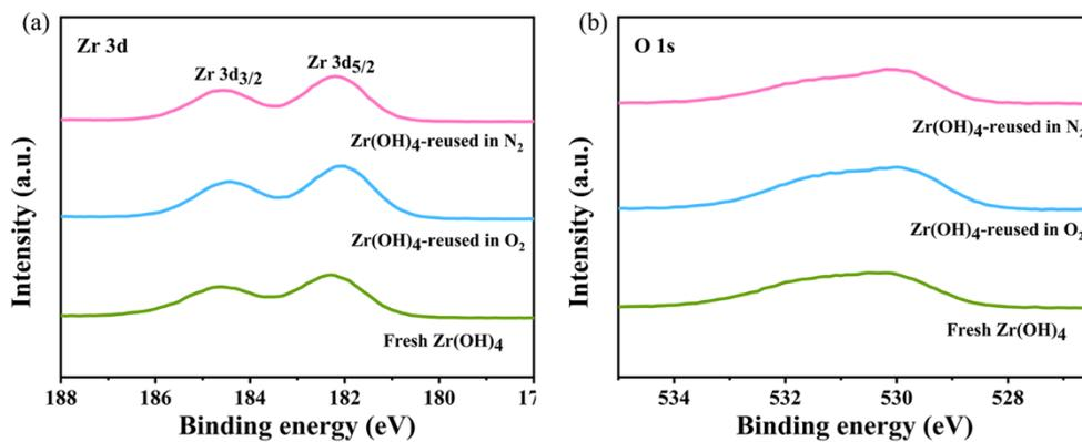
**Figure S3.** Zr 3d (a) and (b) O 1s XPS spectra of fresh  $\text{Zr(OH)}_4$  and six times reused  $\text{Zr(OH)}_4$  after oxidative dehydrogenation and dehydration reaction.
