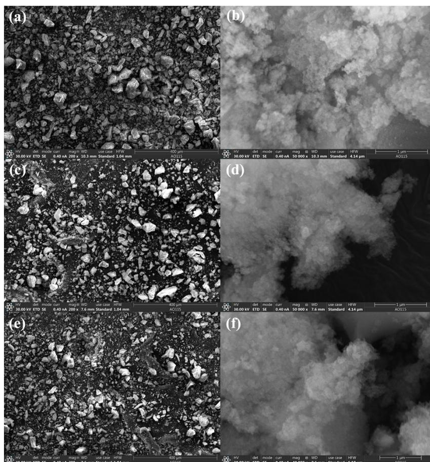
**Figure S1.** Scanning electron microscope (SEM) figures of fresh  $Zr(OH)_4$  (a, b) and six times reused  $Zr(OH)_4$  after oxidative dehydrogenation (c, d) and dehydration reaction (e, f).
