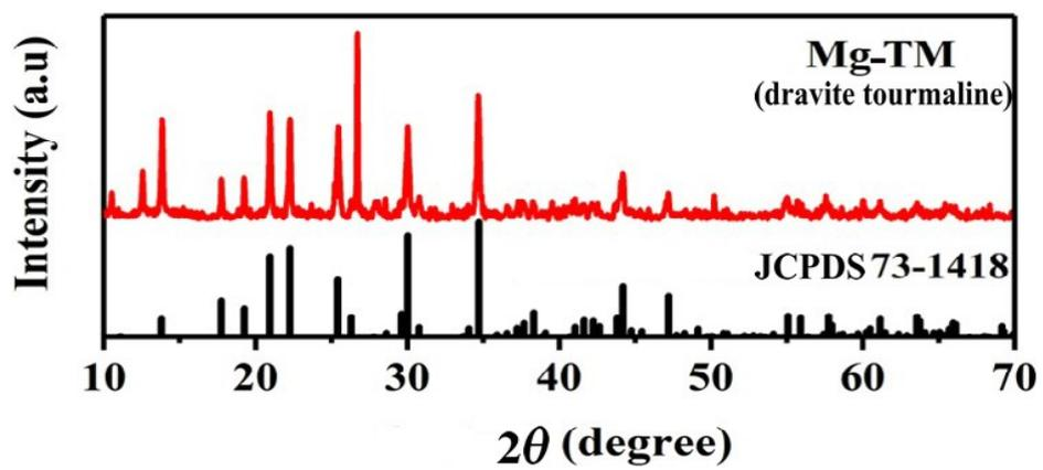
Fig. S2 XRD pattern of Mg-TM.
