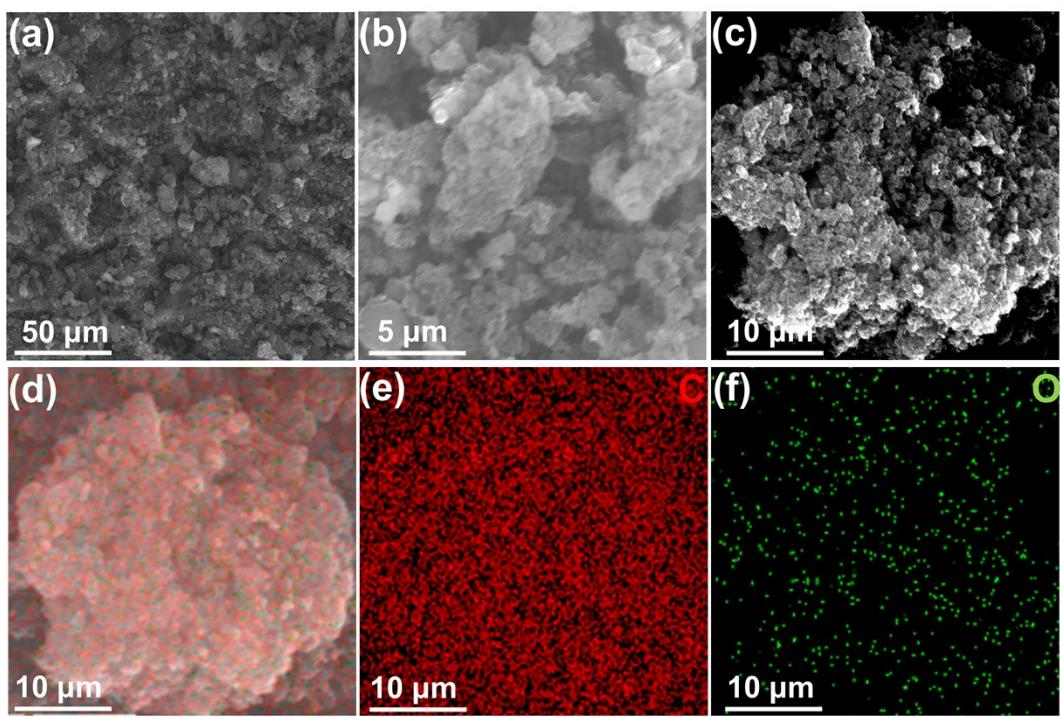
Figure S3. Morphology and element distribution of SMC-1000. (a-b) SEM images. (c-f) SEM and corresponding elemental mapping images.
