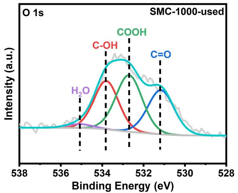
Figure S7. Deconvolution of O 1s XPS spectra of SMC-1000-used.
