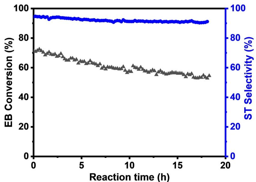
Figure S6. EB conversion and ST selectivity as a function of reaction time.
