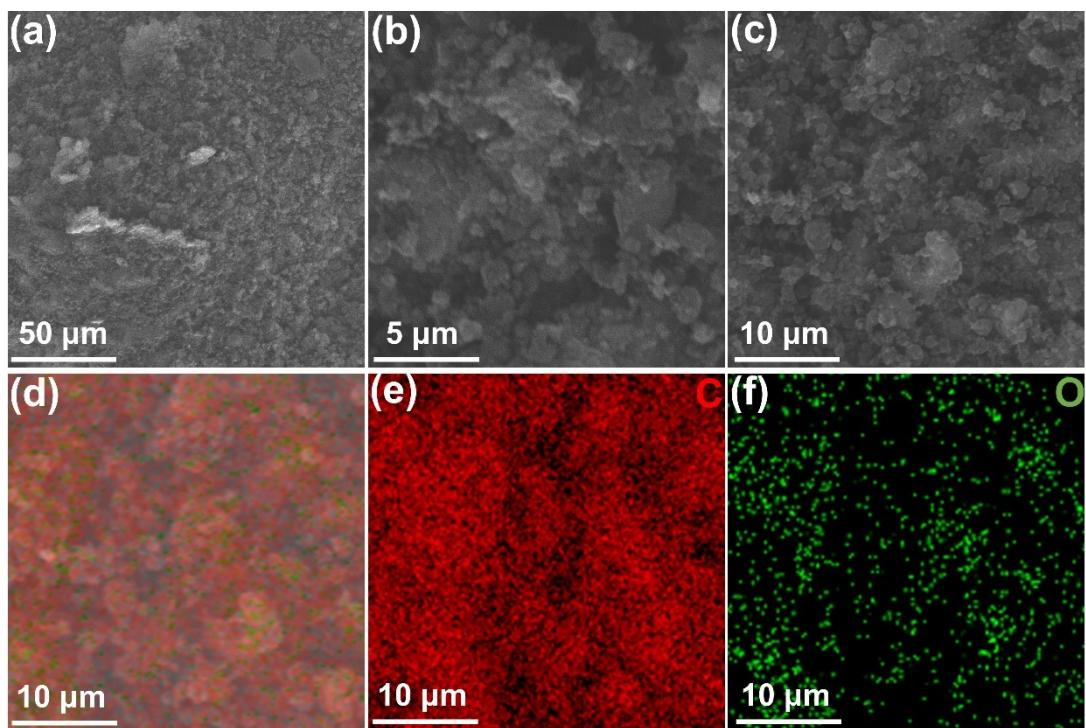
Figure S4. Morphology and element distribution of SMC-1200. (a-b) SEM images. (c-f) SEM and corresponding elemental mapping images.
