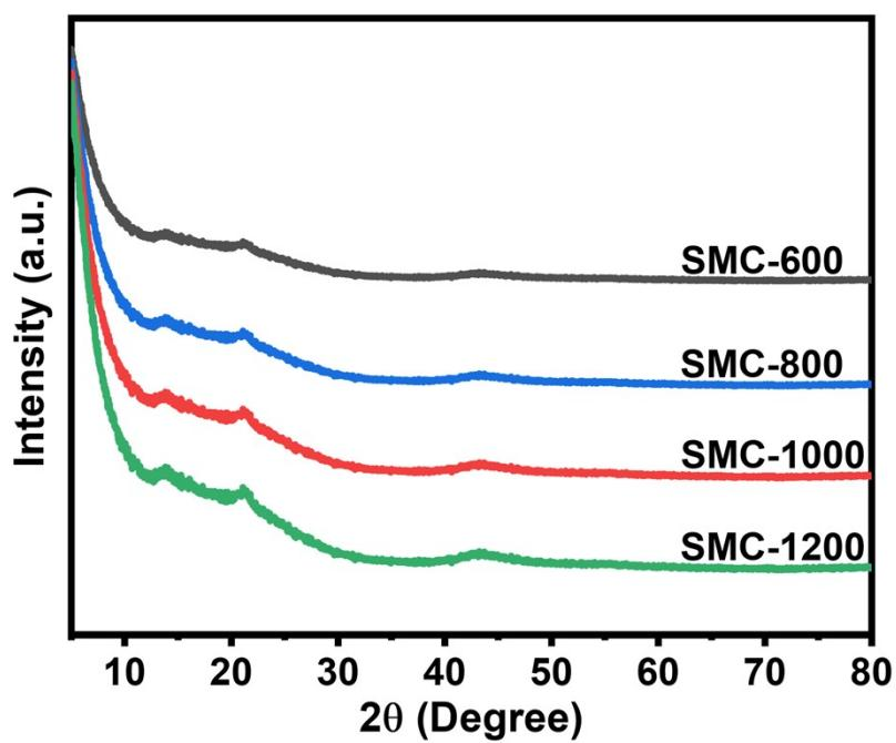
Figure S5. Powder X-ray diffraction pattern of SMC-x.
