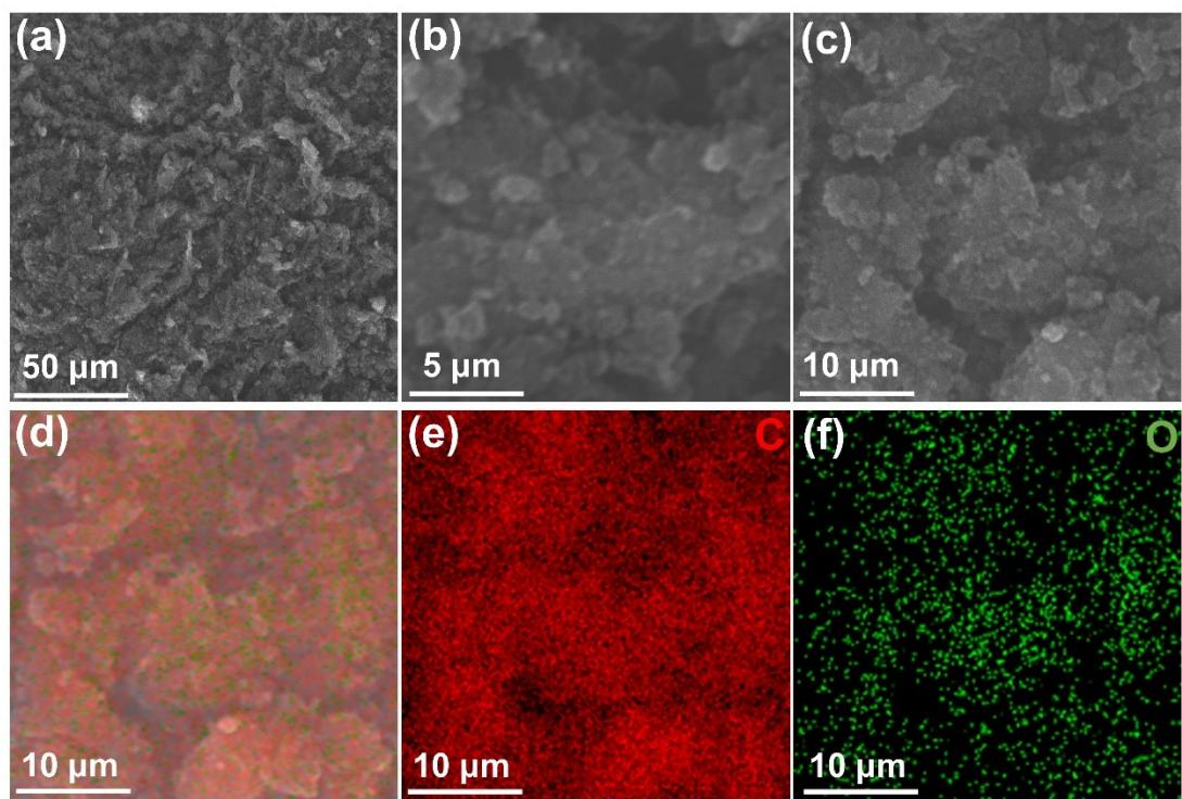
Figure S2. Morphology and element distribution of SMC-800. (a-b) SEM images. (c-f) SEM and corresponding elemental mapping images.
