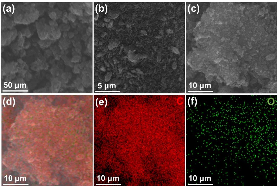
Figure S1. Morphology and element distribution of SMC-600. (a-b) SEM images. (c-f) SEM and corresponding elemental mapping images.
