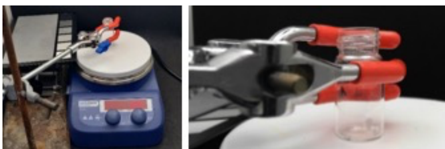
Figure S1: Top – Labelled apparatus set up for video-recording of forensic spot tests. Bottom – close-up of the vial positioning.
