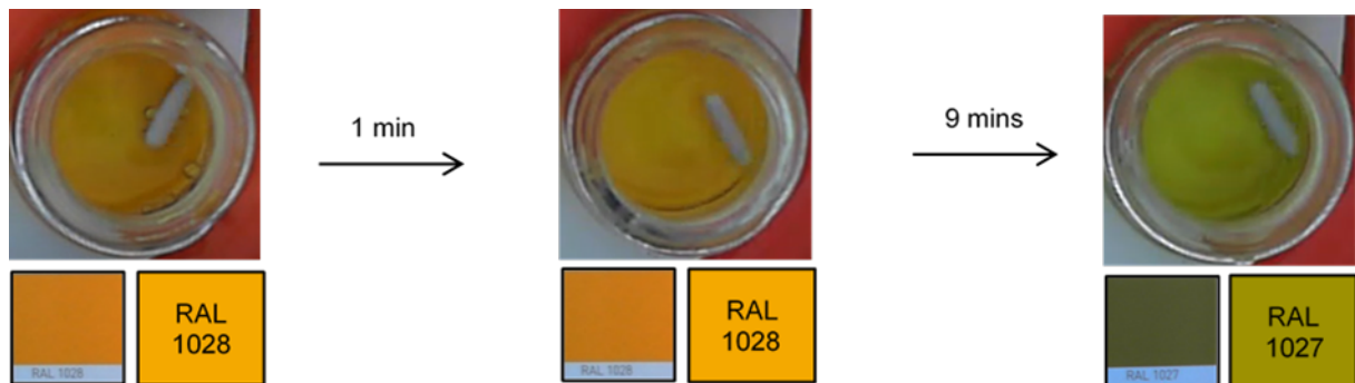
Figure S6: Images of spot test at start (left) and end (right) of the reaction of Glucose with Mandelin reagent.
