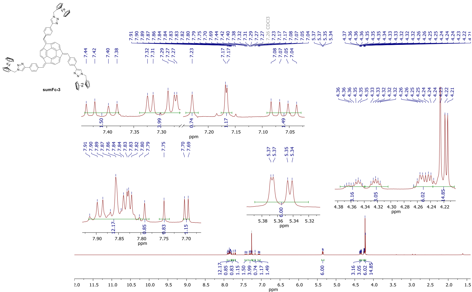
Figure S26. 1 H NMR (500 MHz, CDCl 3 ) spectrum of sumanene-ferrocene conjugate sumFc-3 .
