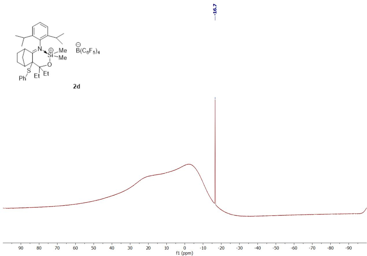
**Figure S20:**  $^{11}\text{B}$  NMR (160 MHz,  $\text{CD}_2\text{Cl}_2$ ) of **2d**
