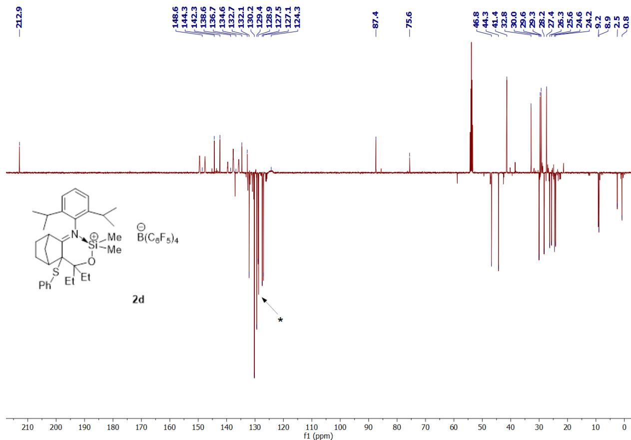
**Figure S18:**  $^{13}\text{C}\{^1\text{H}\}$  NMR (126 MHz,  $\text{CD}_2\text{Cl}_2$ ) of **2d** (\*benzene)
