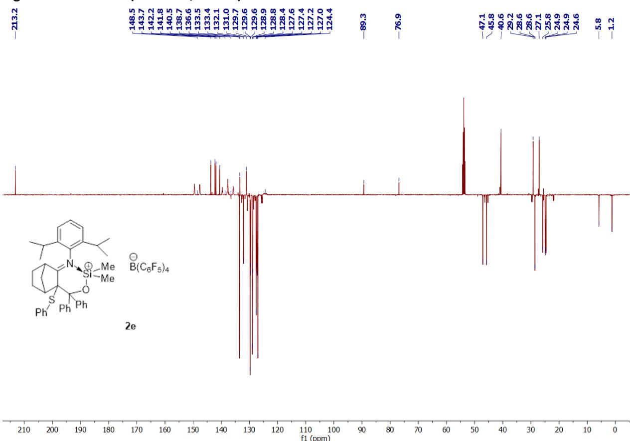
**Figure S23:**  $^{13}\text{C}\{^1\text{H}\}$  NMR (126 MHz,  $\text{CD}_2\text{Cl}_2$ ) of **2e** **Figure S24:**  $^{19}\text{F}$  NMR (471 MHz,  $\text{CD}_2\text{Cl}_2$ ) of **2e**
