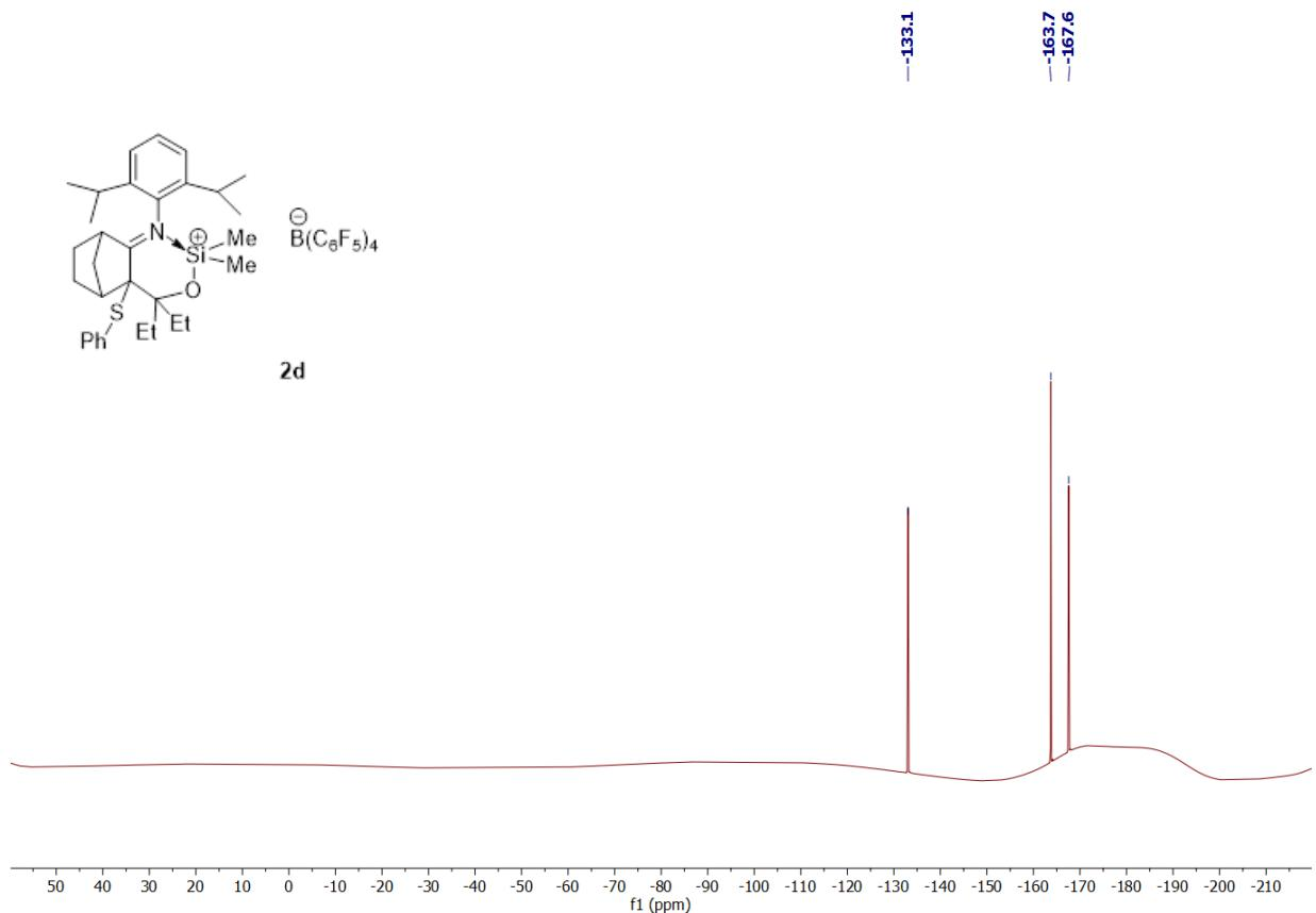
**Figure S19:**  $^{19}\text{F}$  NMR (471 MHz,  $\text{CD}_2\text{Cl}_2$ ) of **2d**
