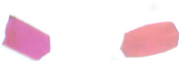
Figure S4. The photographs of the single crystal of 1 under 65% (left) and 95% RH(right).
