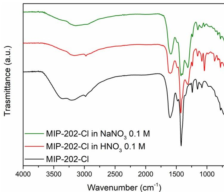
**Figure S11.** ATR-IR spectra of MIP-202-Cl as synthesised (black), after soaking in HNO<sub>3</sub> 0.1 M (red) and after soaking in NaNO<sub>3</sub> 0.1 M (green).
