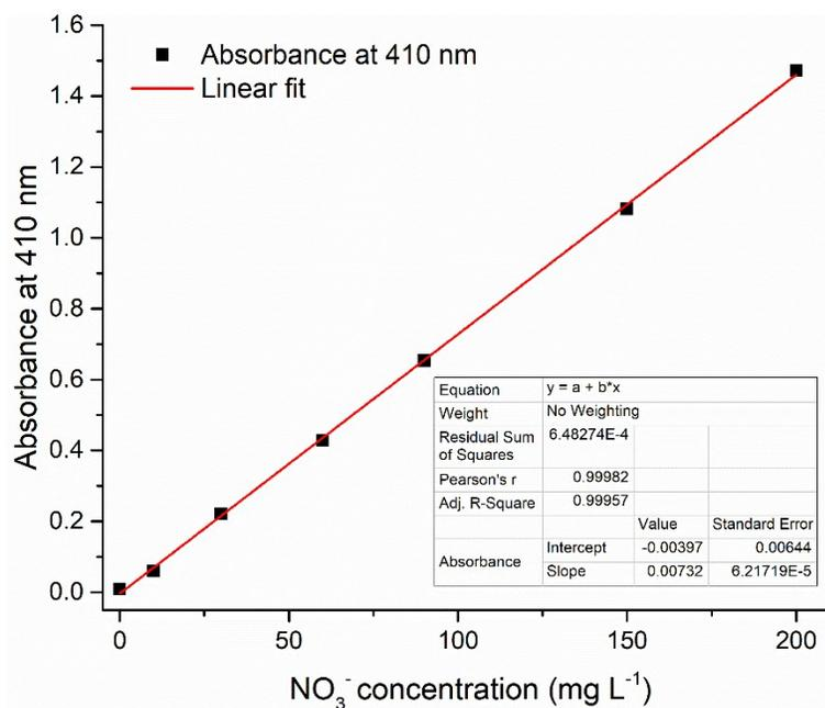
**Figure S1.** Calibration curve used for the quantification of nitrate released in aqueous solution by MIP-202-NO<sub>3</sub>.
