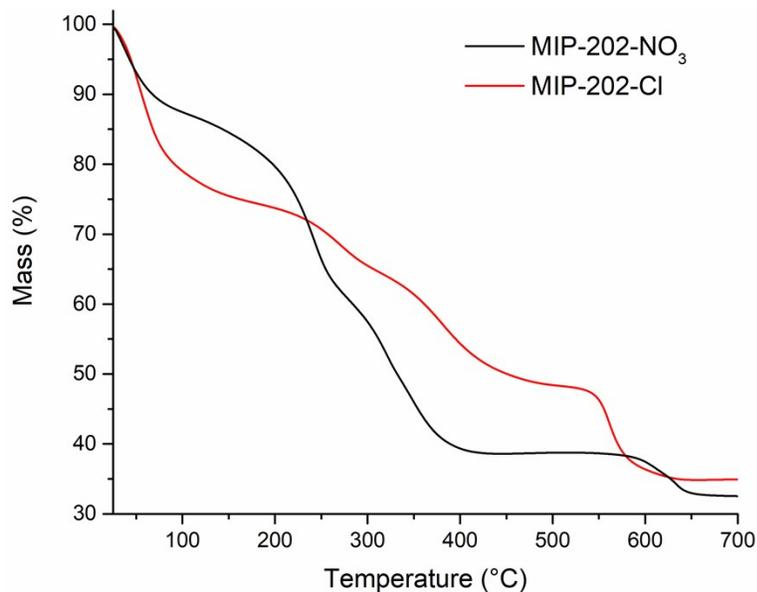
**Figure S6.** Thermogravimetric curves of MIP-202-NO<sub>3</sub> (black) and MIP-202-Cl (red).
