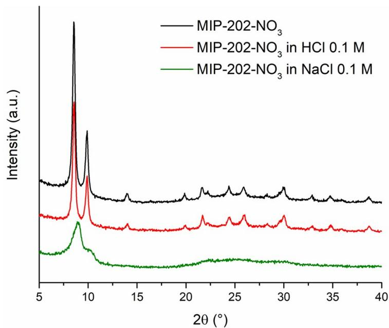
**Figure S8.** PXRD patterns of MIP-202-NO<sub>3</sub> as synthesised (black), after soaking in HCl 0.1 M (red) and after soaking in NaCl 0.1 M (green).
