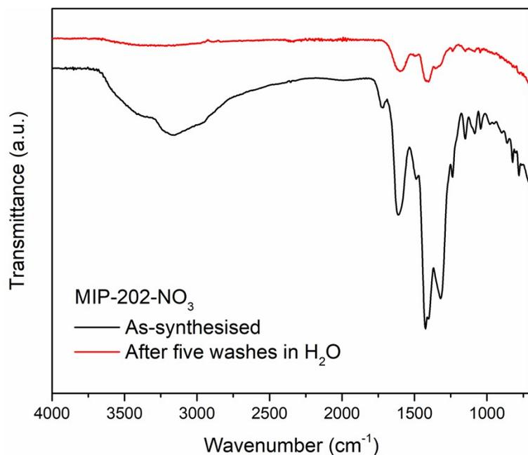
**Figure S20.** ATR-IR spectra of MIP-202-NO<sub>3</sub> as synthesised (black) and after five water washes (red).
