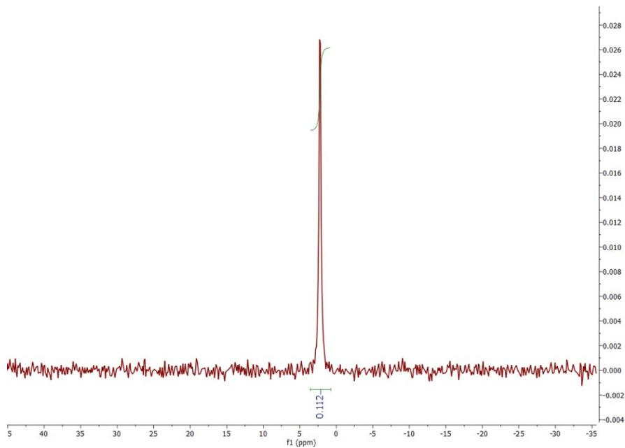
**Figure S13.**  $^{35}\text{Cl}$ -NMR spectrum of 11.1 mg of dry MIP-202- $\text{NO}_3/\text{HCl}$  digested in 1 mL of 1 M NaOH in  $\text{D}_2\text{O}$  in the presence of 0.100 M fumaric acid. The value shown for the integral (0.112) is the absolute value. The same signal for the external standard (0.050 M NaCl solution in 1 M aqueous NaOH) integrates 0.225. The concentration of chloride is derived to be 0.0249 M, corresponding to 0.88 mg of chloride in the original solid (7.9 wt%).
