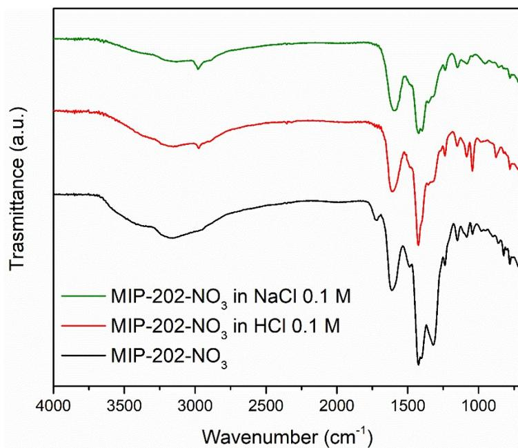
**Figure S10.** ATR-IR spectra of MIP-202-NO<sub>3</sub> as synthesised (black), after soaking in HCl 0.1 M (red) and after soaking in NaCl 0.1 M (green).
