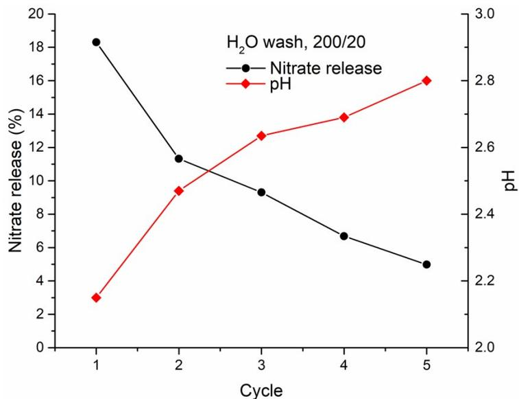
**Figure S21.** Nitrate release (black) and pH of the supernatant (red) during five cycles of washing of 200 mg of MIP-202-NO<sub>3</sub> in 20 mL water.
