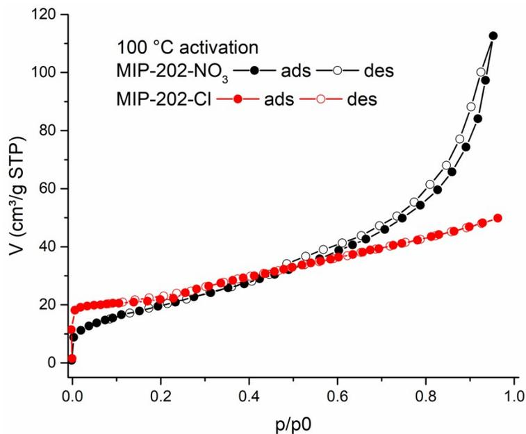
**Figure S7.** N<sub>2</sub> adsorption (filled symbols) and desorption (empty symbols) isotherms of MIP-202-NO<sub>3</sub> (black) and MIP-202-Cl (red) upon activation at 100 °C for 16 h.
