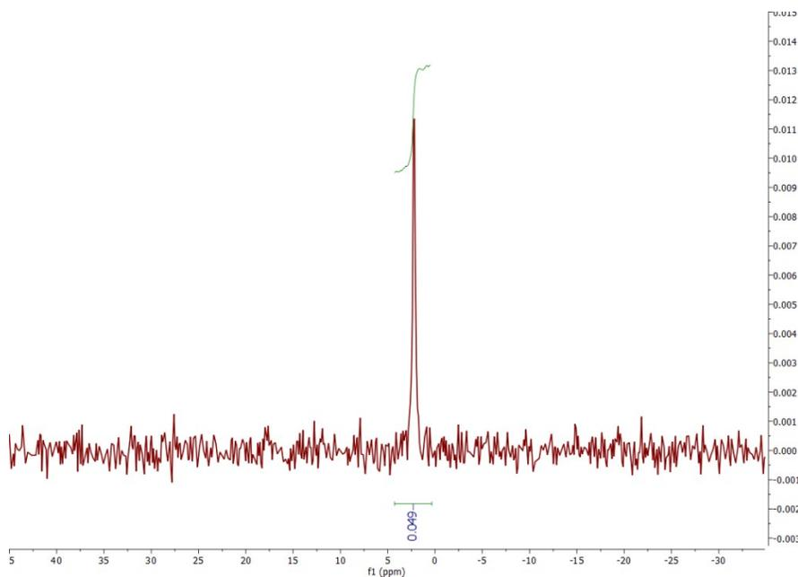
**Figure S15.**  $^{35}\text{Cl}$ -NMR spectrum of 12.8 mg of dry MIP-202-Cl/HNO<sub>3</sub> digested in 1 mL of 1 M NaOH in D<sub>2</sub>O in the presence of 0.100 M fumaric acid. The value shown for the integral (0.049) is the absolute value. The same signal for the external standard (0.050 M NaCl solution in 1 M aqueous NaOH) integrates 0.225. The concentration of chloride is derived to be 0.0107 M, corresponding to 0.38 mg of chloride in the original solid (3.0 wt%).
