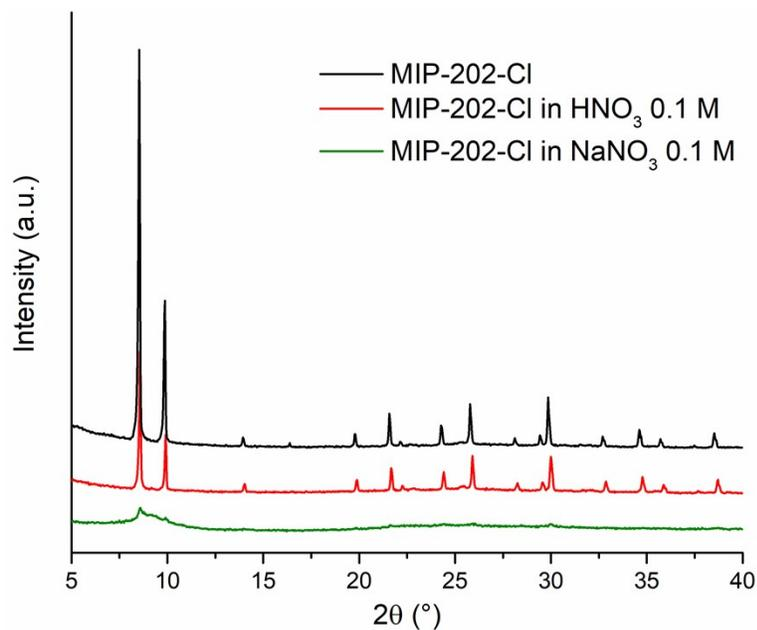
**Figure S9.** PXRD patterns of MIP-202-Cl as synthesised (black), after soaking in HNO<sub>3</sub> 0.1 M (red) and after soaking in NaNO<sub>3</sub> 0.1 M (green).
