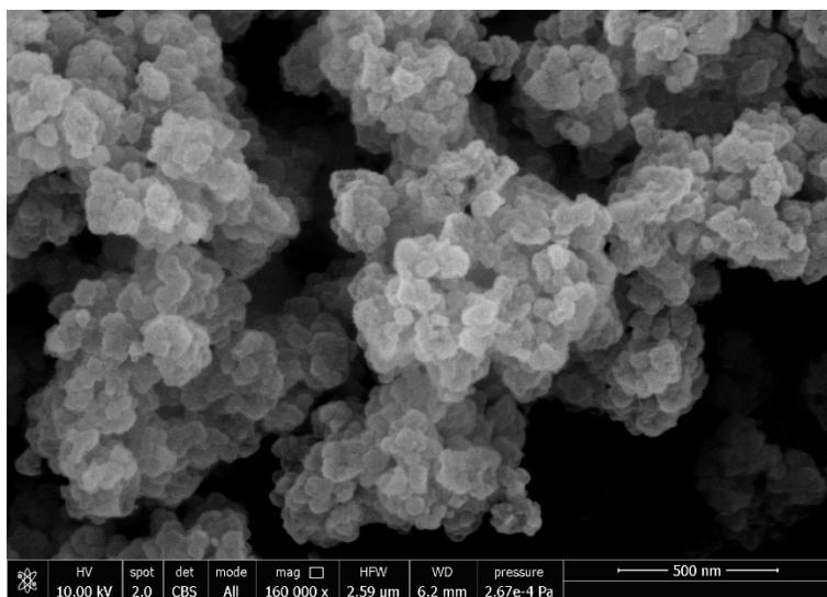
**Figure S2.** SEM micrograph of MIP-202-NO<sub>3</sub>.
