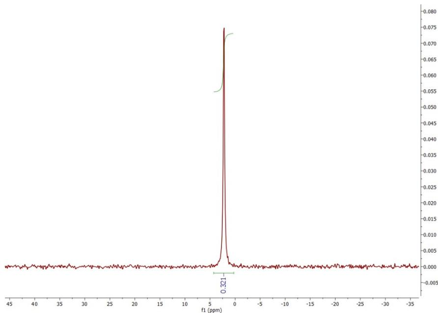
**Figure S5.**  $^{35}\text{Cl}$ -NMR spectrum of 16.5 mg of dry MIP-202-Cl digested in 1 mL of 1 M NaOH in  $\text{D}_2\text{O}$  in the presence of 0.100 M fumaric acid. The value shown for the integral (0.321) is the absolute value. The same signal for the external standard (0.050 M NaCl solution in 1 M aqueous NaOH) integrates 0.225. The concentration of chloride is derived to be 0.0713 M, corresponding to 2.53 mg of chloride in the original solid (15.3 wt%).
