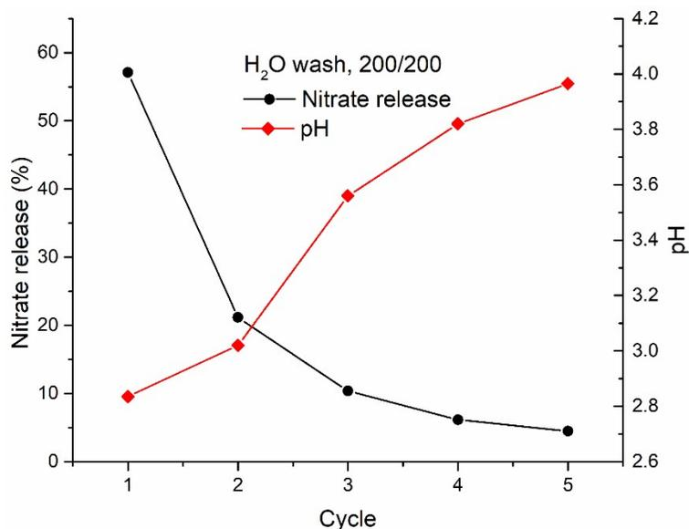
**Figure S16.** Nitrate release (black) and pH of the supernatant (red) during five cycles of washing of 200 mg of MIP-202-NO<sub>3</sub> in 200 mL water.
