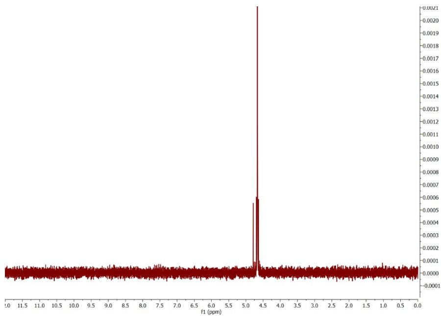
**Figure S17.** Full <sup>1</sup>H-NMR spectrum of the supernatant when 2 mg of MIP-202-NO<sub>3</sub> were dispersed in 200 mL of D<sub>2</sub>O for 1 h.
