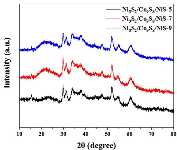
Fig. S1 XRD patterns of Ni<sub>3</sub>S<sub>2</sub>/Co<sub>9</sub>S<sub>8</sub>/NiS-7 (x = 5, 7 and 9 cycles).
