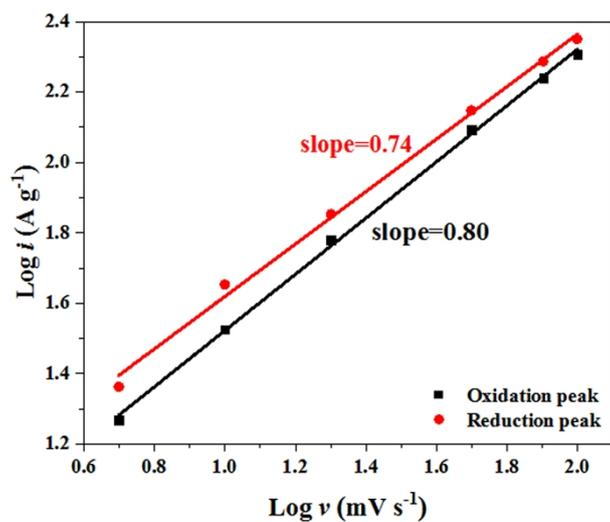
Fig. S8 Straight line relationship of  $\log i$  and  $\log v$  of Ni<sub>3</sub>S<sub>2</sub>/Co<sub>9</sub>S<sub>8</sub>/NiS-9 electrode.
