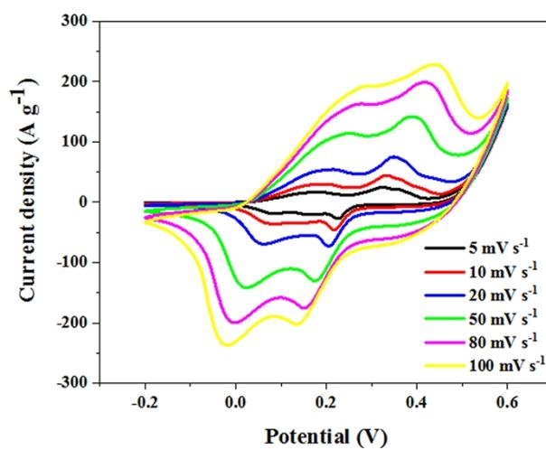
Fig. S5 CV curves of  $\text{Ni}_3\text{S}_2/\text{Co}_9\text{S}_8/\text{NiS}$ -5.
