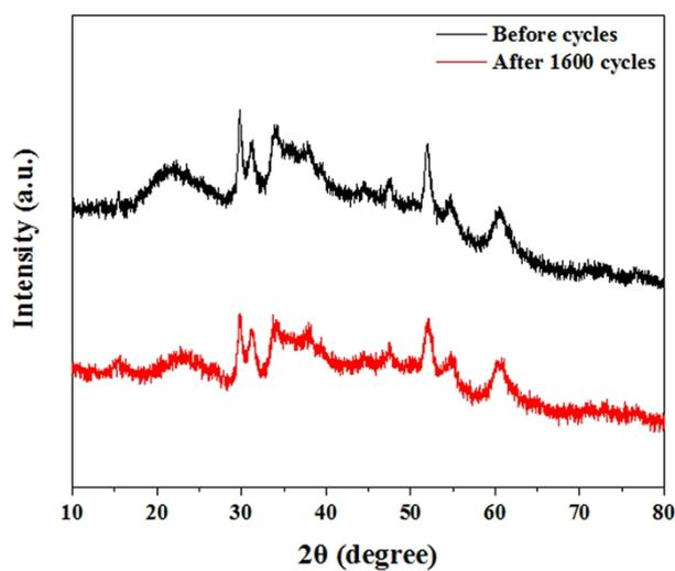
**Fig. S15** XRD of before and after 1600 cycles for Ni<sub>3</sub>S<sub>2</sub>/Co<sub>9</sub>S<sub>8</sub>/NiS-7 electrode.
