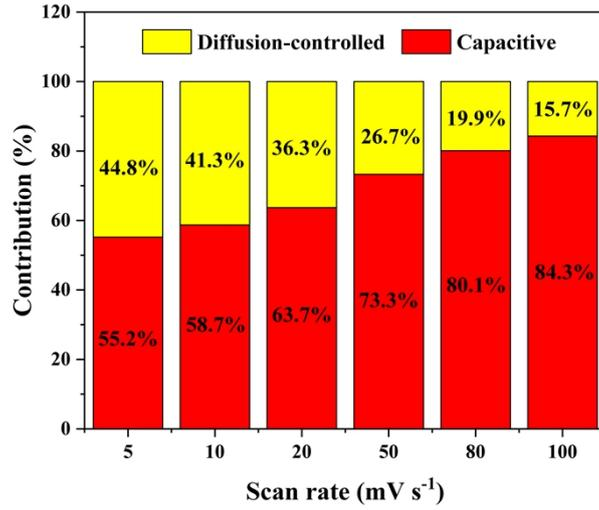
Fig. S9 Normalized contribution ratio of capacitive capacities at different scan rates of Ni<sub>3</sub>S<sub>2</sub>/Co<sub>9</sub>S<sub>8</sub>/NiS-5 electrode.
