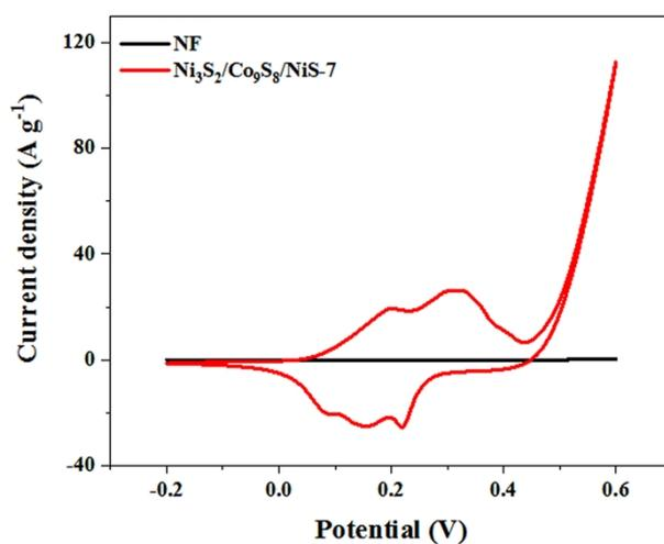
Fig. S4 The CV curves of NF and  $\text{Ni}_3\text{S}_2/\text{Co}_9\text{S}_8/\text{NiS}$ -7 at  $5 \text{ mV s}^{-1}$ .
