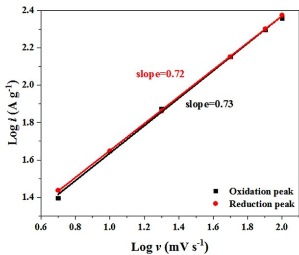
Fig. S7 Straight line relationship of  $\log i$  and  $\log v$  of Ni<sub>3</sub>S<sub>2</sub>/Co<sub>9</sub>S<sub>8</sub>/NiS-5 electrode.
