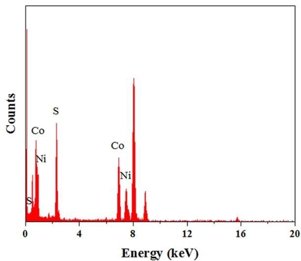
Fig. S3 EDX spectrum of the  $\text{Ni}_3\text{S}_2/\text{Co}_9\text{S}_8/\text{NiS}$ -7.
