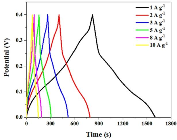
Fig. S12 GCD curves of Ni<sub>3</sub>S<sub>2</sub>/Co<sub>9</sub>S<sub>8</sub>/NiS-9 electrode at different current densities.
