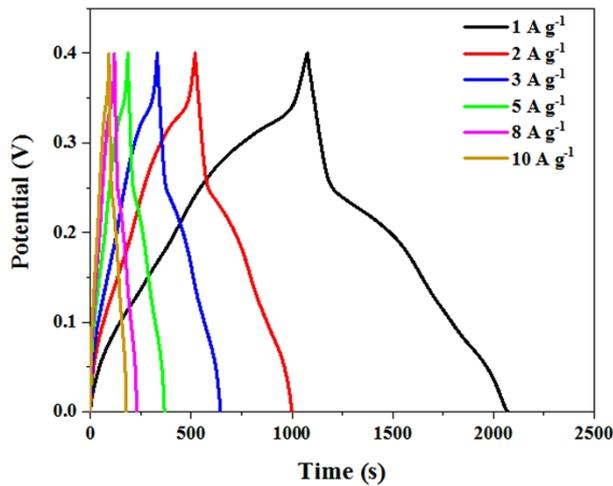
Fig. S11 GCD curves of Ni<sub>3</sub>S<sub>2</sub>/Co<sub>9</sub>S<sub>8</sub>/NiS-5 electrode at different current densities.
