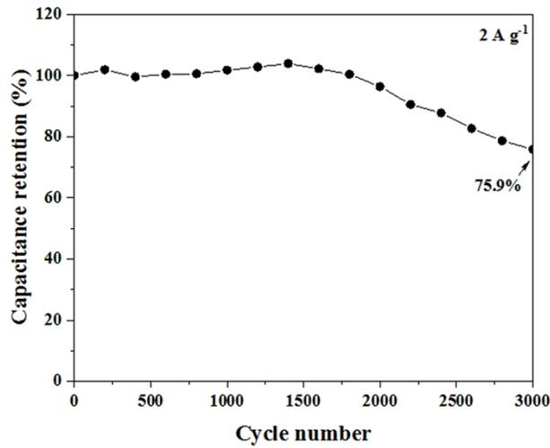
Fig. S13 Cycling stability of Ni<sub>3</sub>S<sub>2</sub>/Co<sub>9</sub>S<sub>8</sub>/NiS-5.
