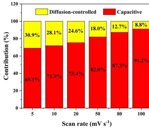
Fig. S10 Normalized contribution ratio of capacitive capacities at different scan rates of Ni<sub>3</sub>S<sub>2</sub>/Co<sub>9</sub>S<sub>8</sub>/NiS-9 electrode.
