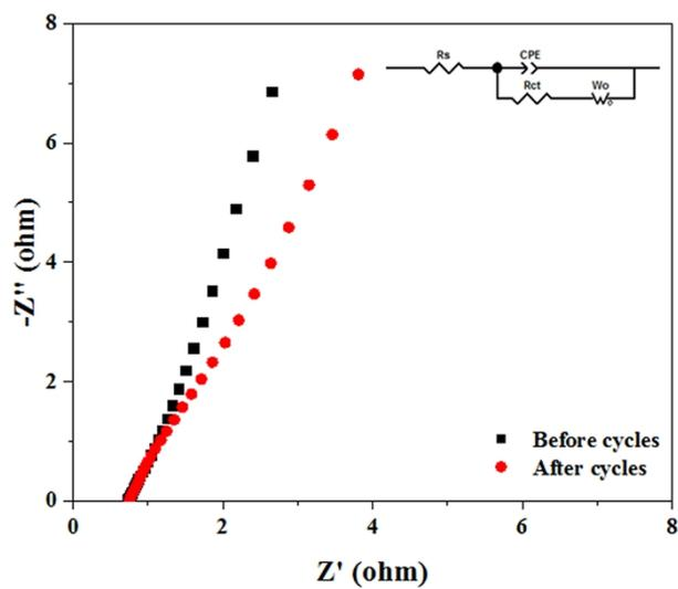
Fig. S16 Nyquist plots of before and after cycles for  $\text{Ni}_3\text{S}_2/\text{Co}_9\text{S}_8/\text{NiS-7}$  electrode.
