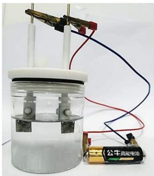
Figure S15. The photograph of overall water splitting powered by a battery with a nominal voltage of 1.5 V.
