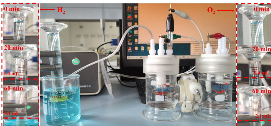
Figure S20. Photograph of the gas collection device and the amount of hydrogen and oxygen gas generated at 0 min, 20min, and 60min.
