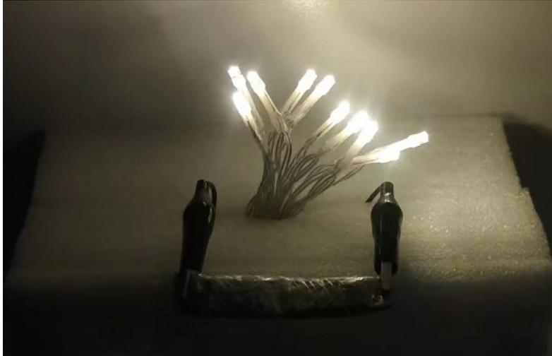
**Fig. S17.** Two series-connected ASC devices light up the LEDs.
