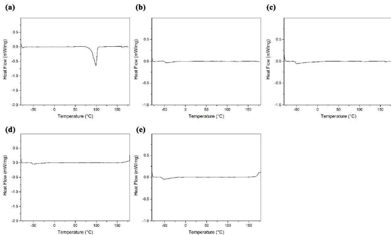
**Figure S69.** DSC Curves of 4a-4e.
