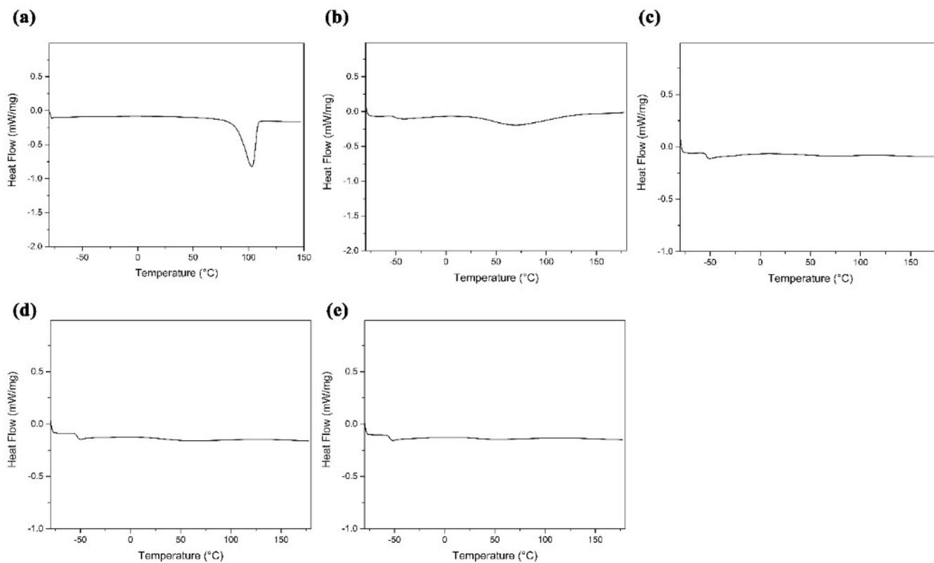
**Figure S68.** DSC Curves of 3a-3e.
