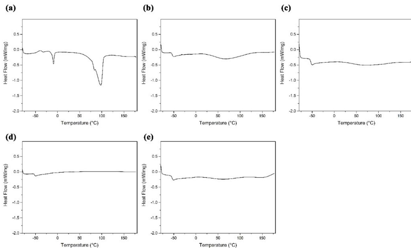
**Figure S66.** DSC Curves of 1a-1e.
