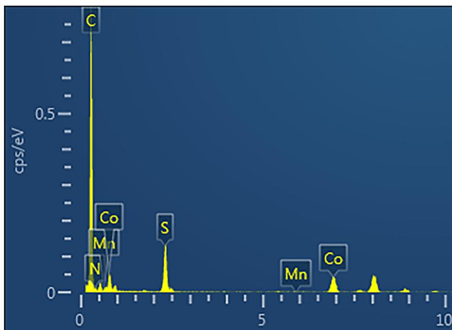
Fig. S4 Energy-dispersive X-ray spectroscopy (EDS) spectrum of  $\text{Co}_{1-x}\text{S}/\text{MnS}/\text{NC}$
