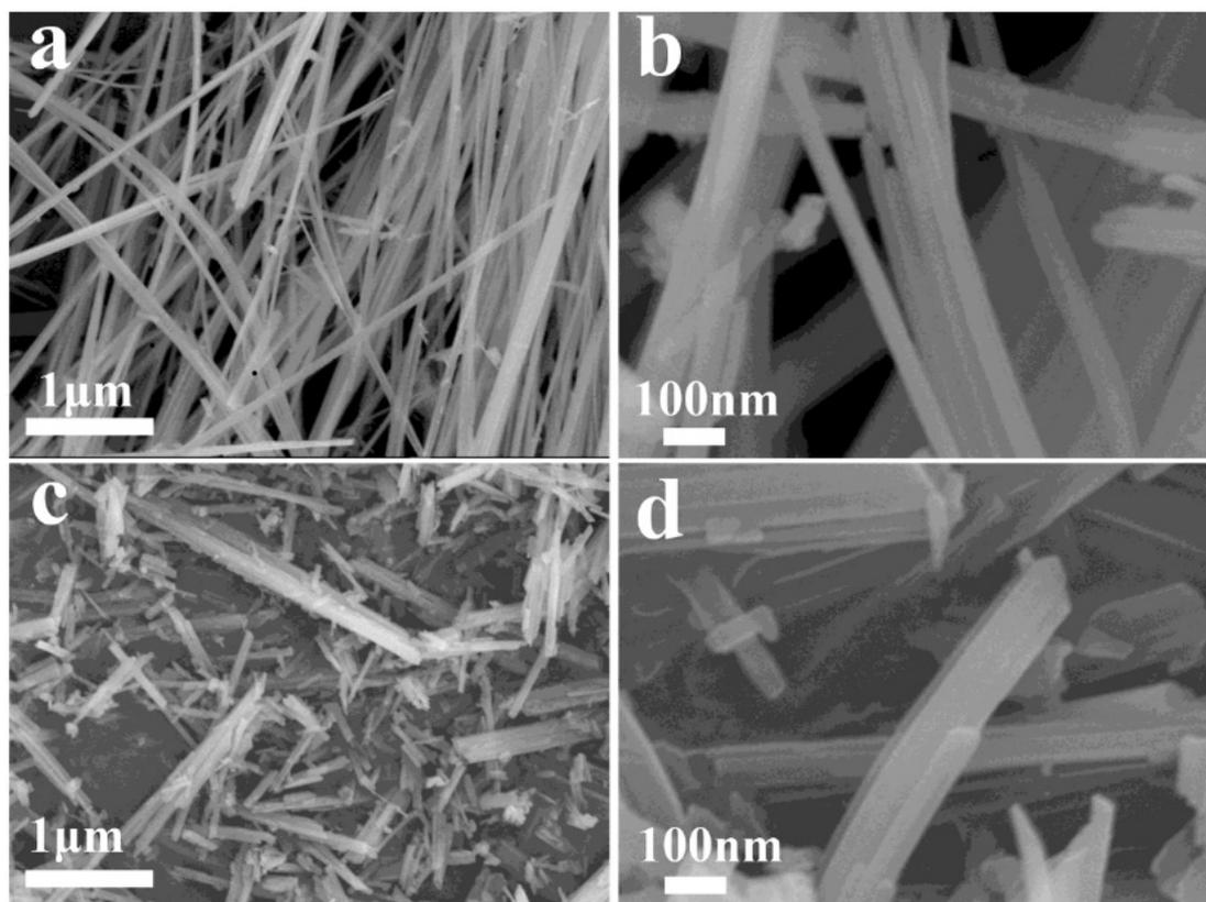
Fig. S2 SEM images of (a, b) Co-NTA precursors. (c, d) Mn-NTA precursors.
