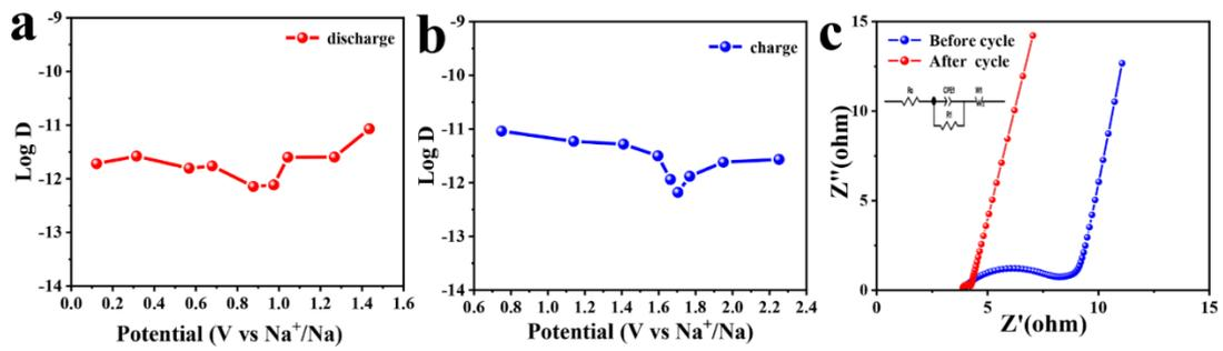
**Fig. S5** (a) The diffusion coefficient of  $\text{Na}^+$  in discharge processes. (b) The diffusion coefficient of  $\text{Na}^+$  in charge processes. (c) Nyquist plots of  $\text{Co}_{1-x}\text{S}/\text{MnS}/\text{NC}$  in SIBS (inset: equivalent circuit).
