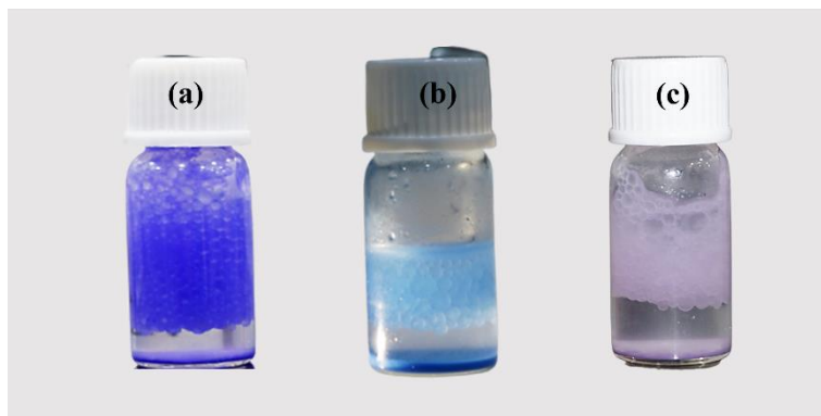
Figure S15. (a) Pickering emulsions of n-heptane-in-water stabilized by UP' MOF particles using Acid violet 49 dye. (b) Stabilized Pickering emulsions of n-heptane-in-water using Trypan blue dye. (c) Stabilized Pickering emulsions of n-heptane-in-water using Colcon dye. (Concentration of each water-soluble dye is 0.35 \times 10^{-3} M).
