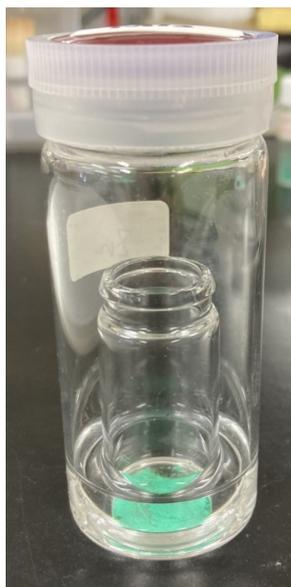
**Figure S5** A small vial (10 mL) containing approximately 20 mg of powder **1** was placed into a larger vial (50 mL) containing 5 mL of either ammonia or amine solution.
