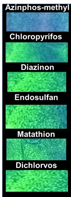
Figure S34. Colour of Tb-phen coated paper strips in presence of different pesticides (75 \mu\text{M} ). Note: the green colour vanishes only in the presence of azinphos-methyl.
