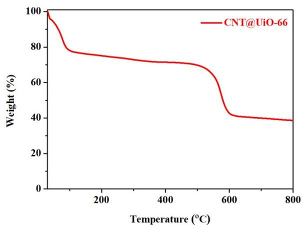
**Fig. S1.** The TGA curve of CNT@UiO-66.
