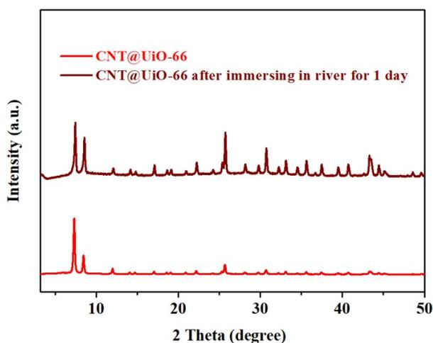
**Fig. S3.** The PXRD patterns of CNT@UiO-66 before and after immersing in river for 1 day.
