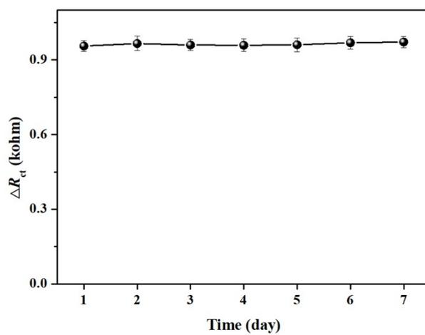
**Fig. S2.** The stability of the CNT@UiO-66-based electrochemical aptasensor for 7 days.
