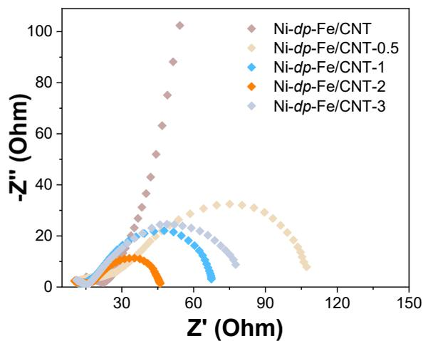
**Fig. S6.** Electrochemical impedance spectra of Ni-*dp*-Fe/CNT, Ni-*dp*-Fe/CNT-0.5, Ni-*dp*-Fe/CNT-1, Ni-*dp*-Fe/CNT-2 and Ni-*dp*-Fe/CNT-3.
