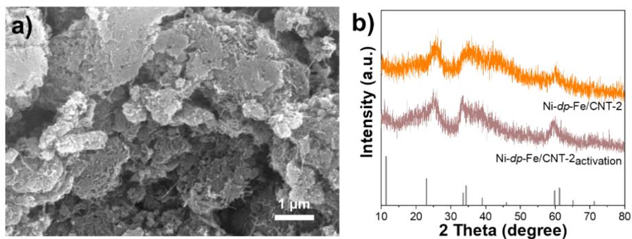
Fig. S3. a) SEM image of Ni-dp-Fe/CNT-2 after activation and b) the XRD pattern.
