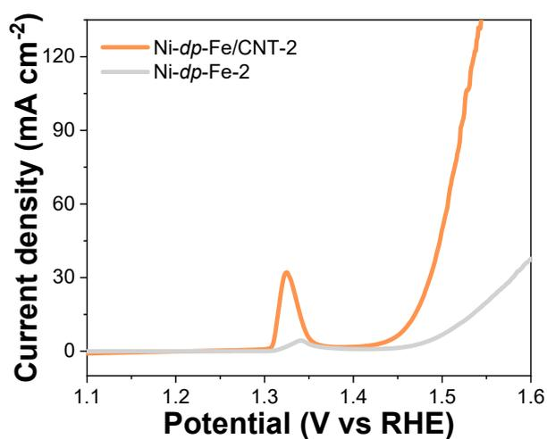
Fig. S4. LSV curves tested on Ni-dp-Fe/CNT-2 and Ni-dp-Fe-2.
