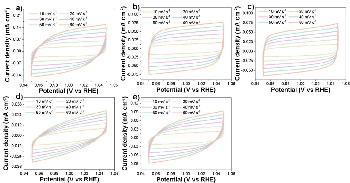
**Fig. S5.** CV curves with different scanning rates of various contrast electrodes. a) Ni-*dp*-Fe/CNT-2, b) Ni-*dp*-Fe/CNT-1, c) Ni-*dp*-Fe/CNT-0.5, d) Ni-*dp*-Fe/CNT and e) Ni-*dp*-Fe/CNT-3.
